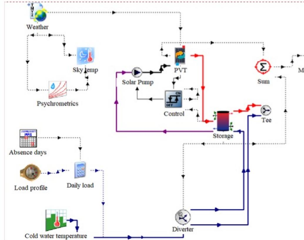
Figure 1: Typical PVT system representation on TRNSYS® deck (Source: Abora Solar).
