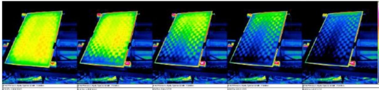
Figure 4: Picture series of a thermal internal shock test according ISO 9806 filing an overheated PVT collector with cold fluid.
