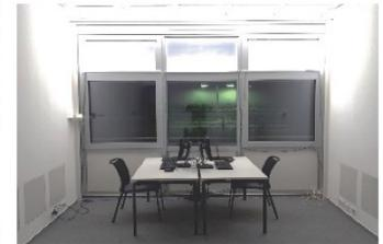
Figure 1. The lab room seen from the inside. The light-emitting structures are placed on the top part of the windows and provide illumination to the room interior.
