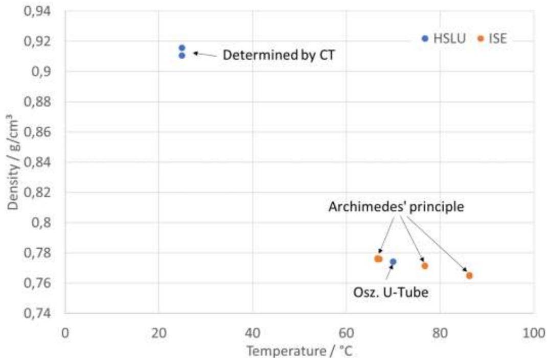
Figure 2: Preliminary results of the round robin test on density measurements.
