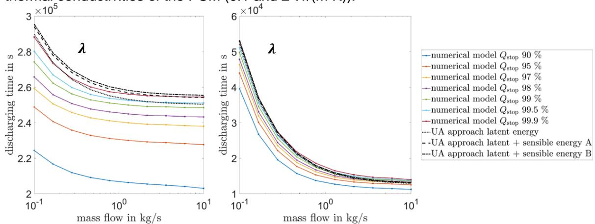
**Figure 8: Comparison of UA approach and numerical model to evaluate the discharging of latent heat storage units.**
