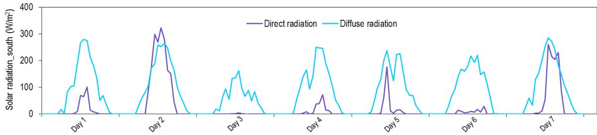
Figure 3: Diurnal variation of direct and diffuse solar radiation for south oriented façade in Amsterdam's climate
