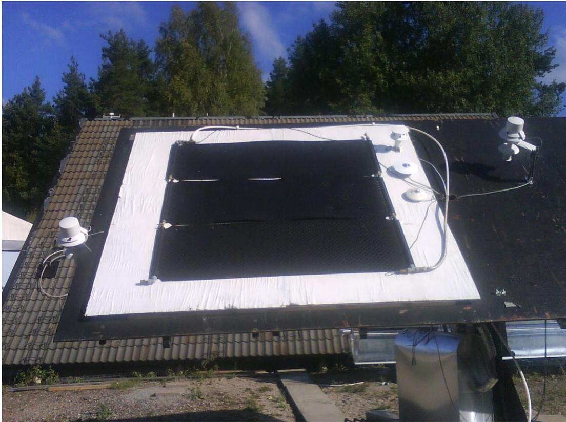
**Fig. 1: The unglazed solar collector on the test stand with extra sensors for humidity, wind speed and air temperature. Also sensors for solar radiation and long-wave thermal sky radiation in the collector plane can be seen to the right of the collector. In the upper right corner a new kind of wind sensor is located. (Photo from SP)**
