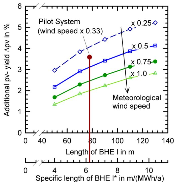
Fig. 7: Influence of the wind speed on the additional PV-yield in the reference system. The length of the BHE is varied while the PVT-collector is 15 m<sup>2</sup>.
