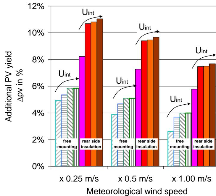
Fig. 8: Additional PV- yield in the reference system (90 m BHE length and 15 m<sup>2</sup> PVT- collector) for varying internal heat transfer  $u_{int}$  rates, wind speeds and different types of installation. The internal heat transfer is varied for values of 25/60/80/95 W/m<sup>2</sup>K.
