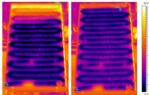
Fig. 5. Thermographs of the absorber plate
