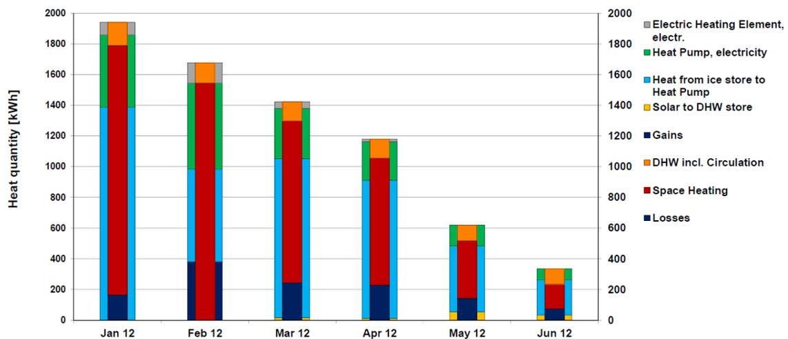
Fig. 4. Monthly energy balances of the monitored solar ice store system
