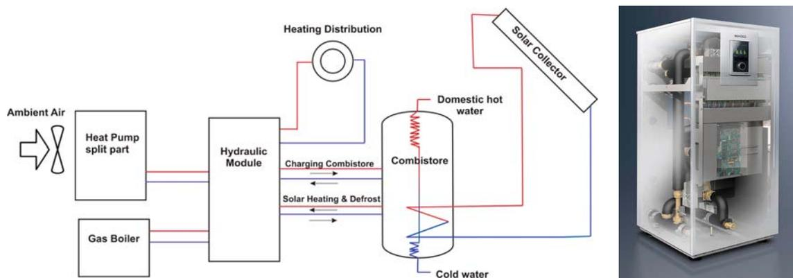
Fig. 1. Simplified hydraulic scheme and inside unit of the air/water split heat pump [Source of picture: Schüco]
