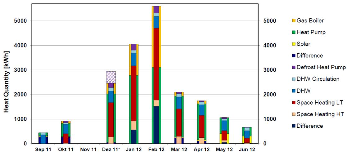
Fig. 2. Monthly energy balances of the monitored hybrid system [\*data for December only from 6.12.2011, 10:00 a.m.]
