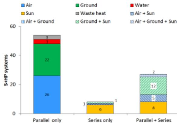
Figure 6: S+HP systems classified accordingly to the plant layout and heat pump source.
