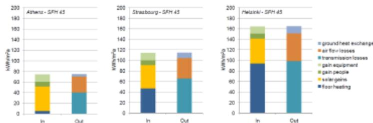
Figure 7: Building energy balances of a Single Family building with an annual heating demand of 45 kWh/(m<sup>2</sup>year) for Strasbourg climate - SFH 45 - at three different reference location.
