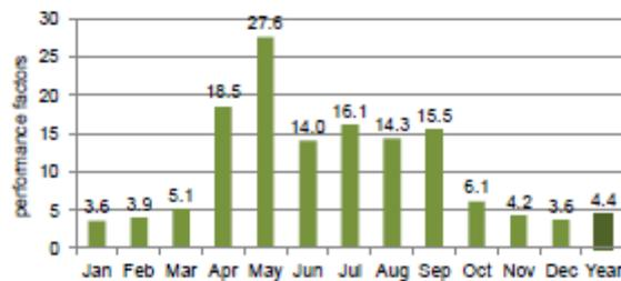
Figure 7: performance factor SPF<sub>DHW</sub> of the system [source: SPF Solartechnik].
