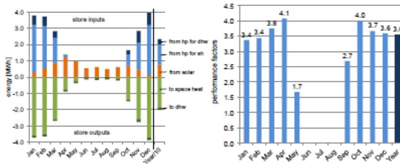
Figure 6: energy balance of the combi-store (left) and performance factor SPF<sub>HP</sub> (right) [source: SPF Solartechnik].
