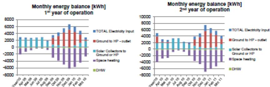
Figure 12: energy balance during the first (left) and second (right) year of operation of the system [source: ISFH].
