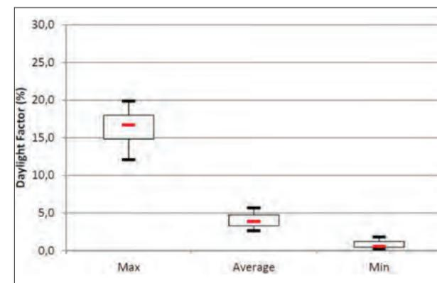
▲ **Figure 5. Exemplary results from the state-of-the-art review of 13 simulation tools. The graphs above show the calculated daylight factors for a test scenario before and after retrofit. The general drop of the daylight factor due to lower light transmittance of new glazing systems (due to low coating) is shown. Plus, the review shows quite a significant spread in the calculation results.**
