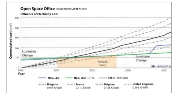
▲ Figure 1. Cumulated costs for typical open space offices as a function of existing installed power, equipment cost and electricity costs. The same representations were generated, for personal offices, manufacturing halls and wholesale / retail.
