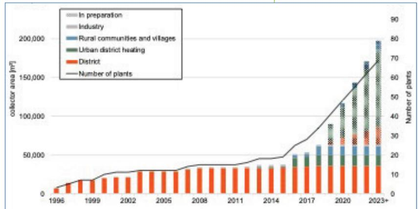
Figure 2 shows that the integration of solar thermal into urban district heating represents about 75% of the newly installed capacity expected for the coming years.
