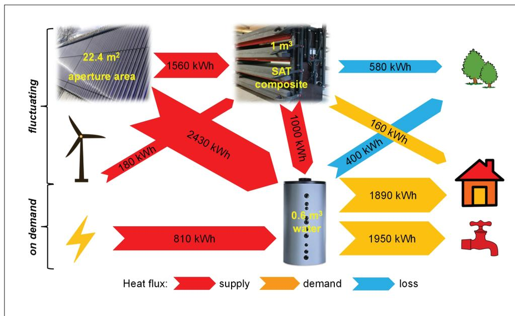
◀ Figure 1. Simulated annual heat flux for a house with 3 occupants in the Danish climate. About 80% of heat demand could be covered by using solar collectors and a recharge of the SAT composite with wind power in January.<sup>3</sup>
