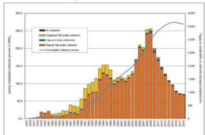
▲ **Figure 2. Market development of solar thermal collectors in Austria until 2018.** (Source: AEE INTEC)
