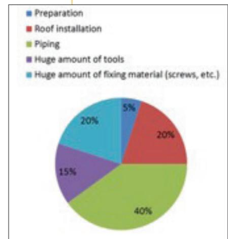
▲ Figure 5. Results of IEA SHC Task 54 installation survey of 23 installation companies in 7 countries. The diagram displays the most time-consuming parts of the installation process.
