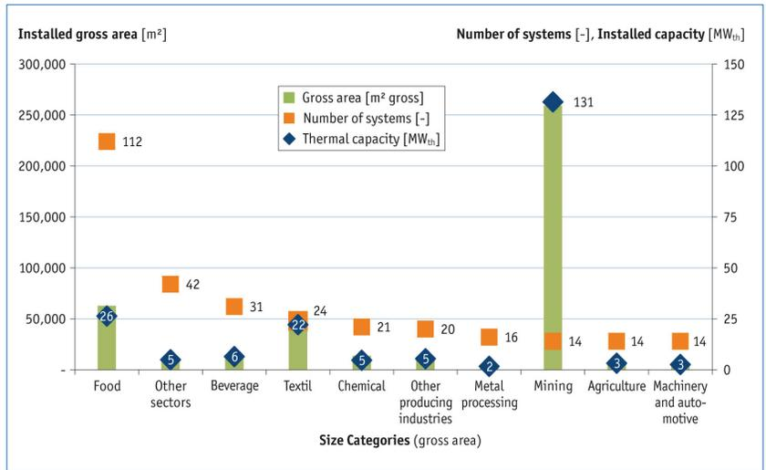
▲ Global solar process heat systems in operation by the end of March 2019 – industry sector. (Source: IEA SHC Task49 / IV SHIP database)
