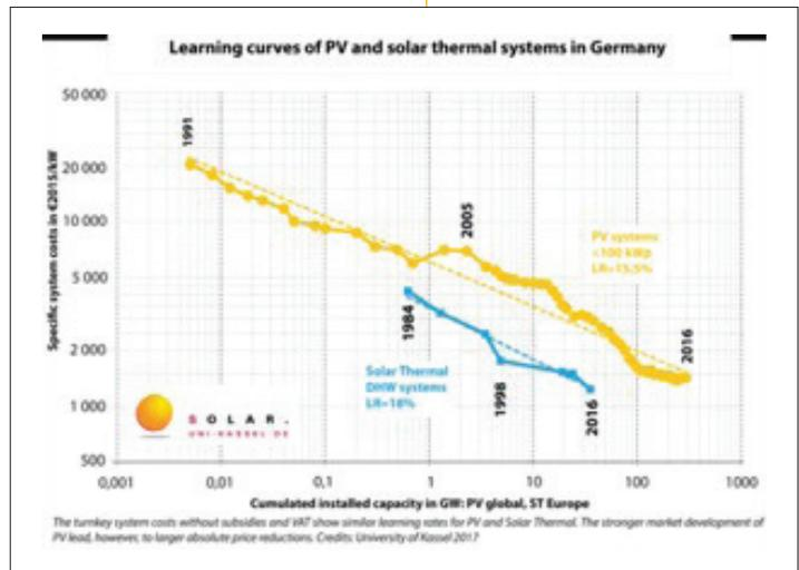
▲ Figure 4. Learning curves of PV and solar thermal systems in Germany (Source: University of Kassel).
