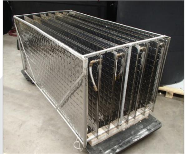
▲ Experimental ice storage heat exchanger using flat plat collectors in stainless steel.
