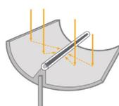
Parabolic trough collector
