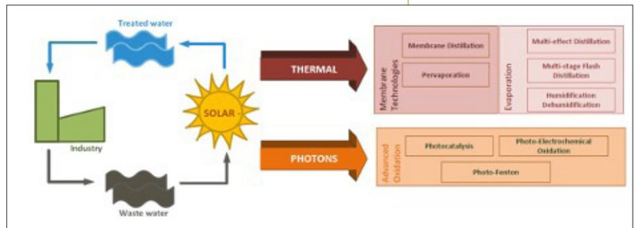
▲ **Figure 1. Overview of technologies potentially being supplied by solar thermal energy or solar photons.** (Source: AEE INTEC)
