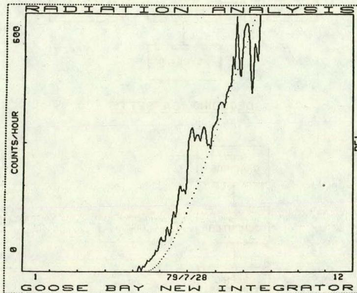
Fig. 11 Radiation trace for morning hours with superimposed clear sky reference curve
