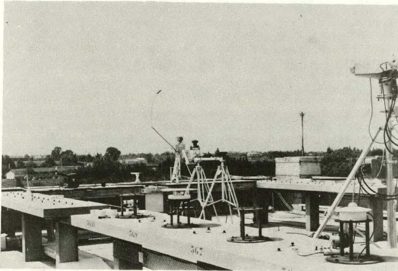
Fig. IV - 9. A shading disc always occults direct solar beam from a fish-eye camera.
