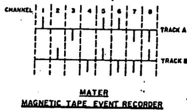
Fig. 3 Encoding tape channel signals
