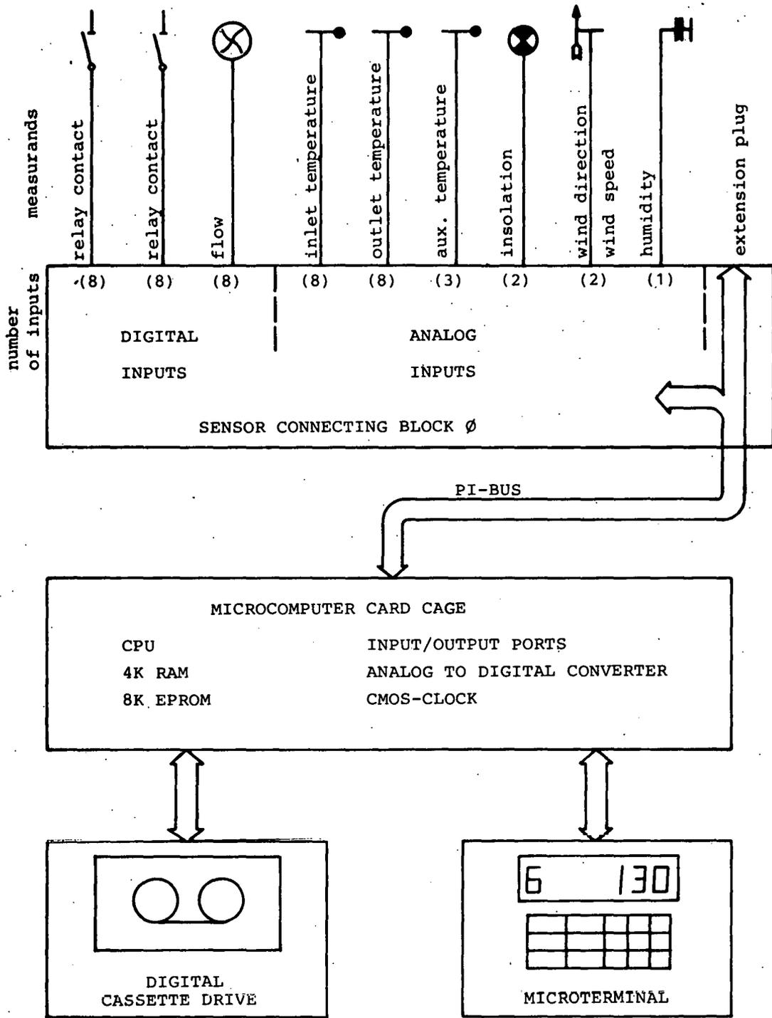
Fig.4. Block diagram of the data acquisition package HELIO-DATA
