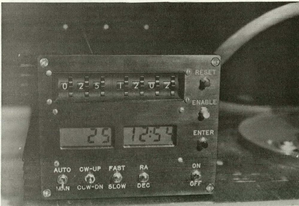
Fig. III-6 Sun Following Pyrheliometer mount and control unit.
