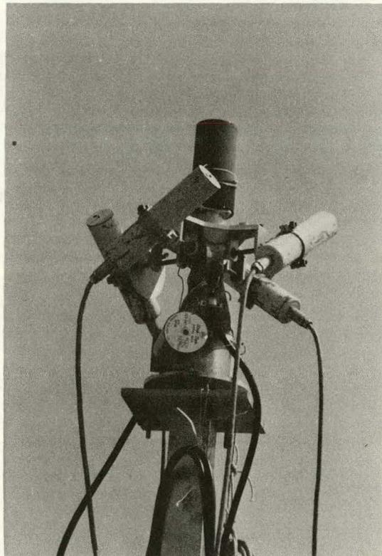
Fig. IV - 8. Four pyroelectric detectors scan the sky ( $5^{\circ}$  aperture)
