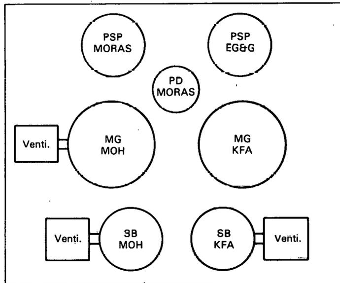
Fig. V-3: Distribution of Radiation Sensors Over the Tilttable Desk (Area: 1.2m x 1.0m) (Pyranometers: PD, PSP, MG Balancemeters: SB)
