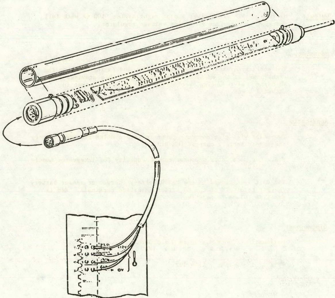
MITS FOR MATERMicropower Integrating Temperature Sensor
