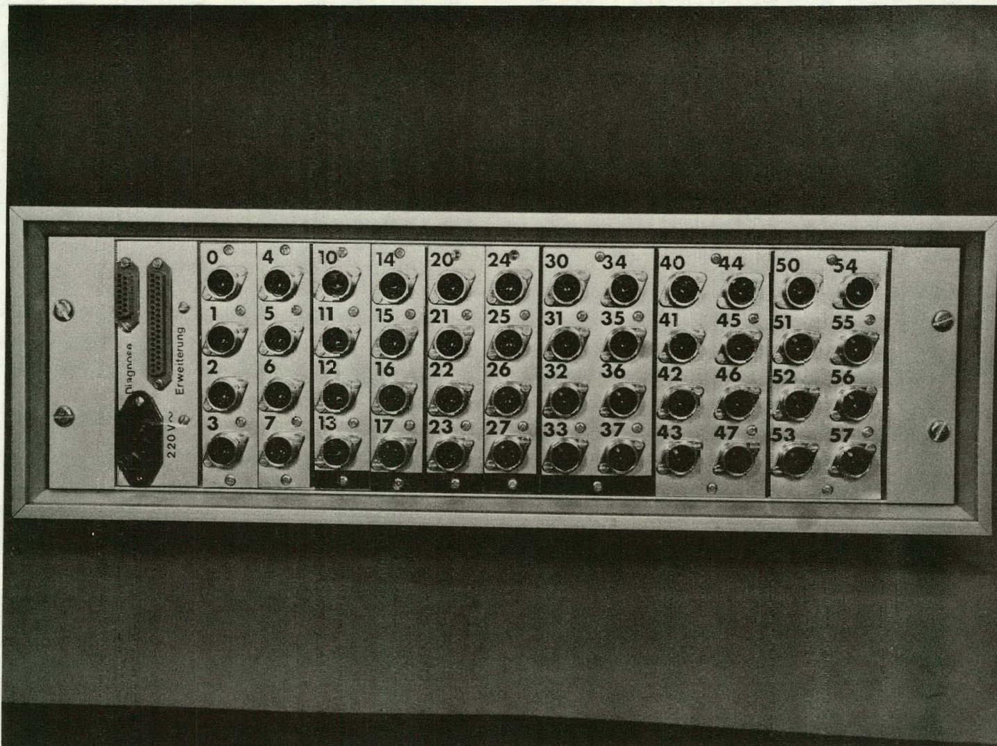
Fig. 3: Rear view of the compact data acquisition device HELIO-DATA 1 shows 24 analog inputs (bayonet socket Nos. 0 - 27) and 24 digital inputs (bayonet socket Nos. 30 - 57) as well as the extension bus socket for additional sensor connecting blocks.
