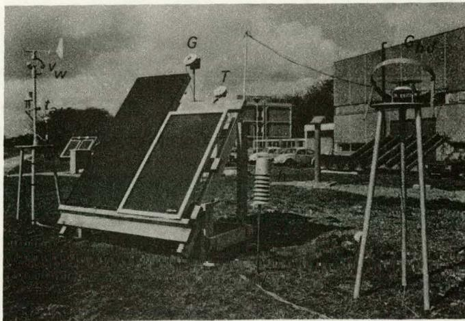
Fig. II-1: Application of the IEA instrument package for determining collector stagnation temperatures.
