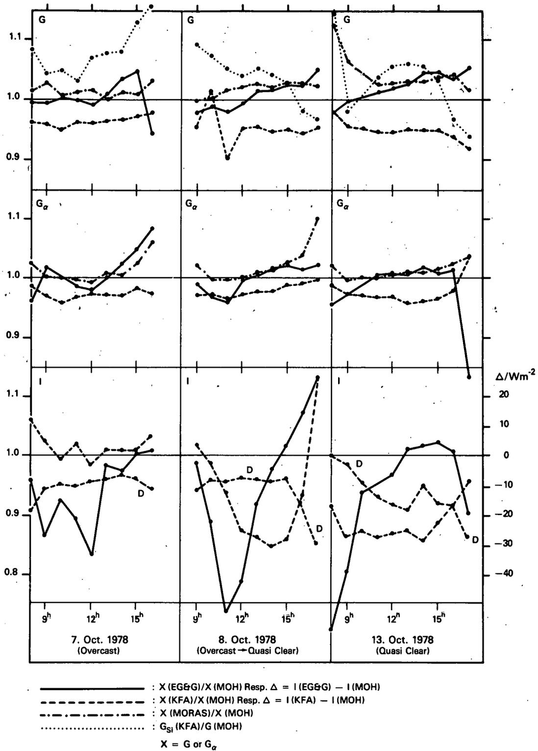
Fig. V-4: Daily Course of Ratios Resp. Differences of Hourly Means Related to the Reference Values, for 3 days with Different Weather Type.
