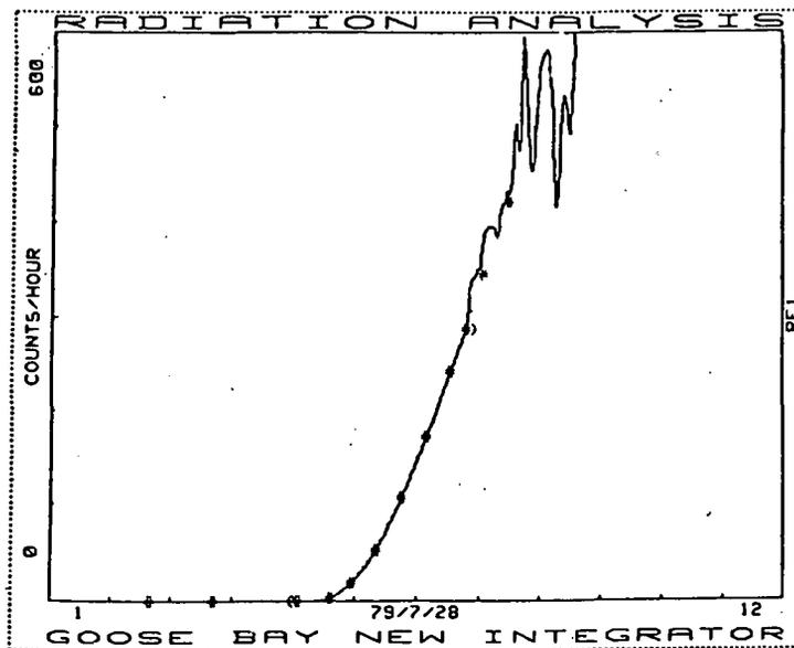
Fig. 13 Radiation trace corrected to clear sky cursor points
