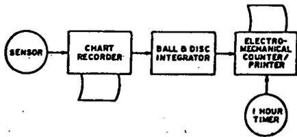
Fig. 1 Current mechanical integrator system
