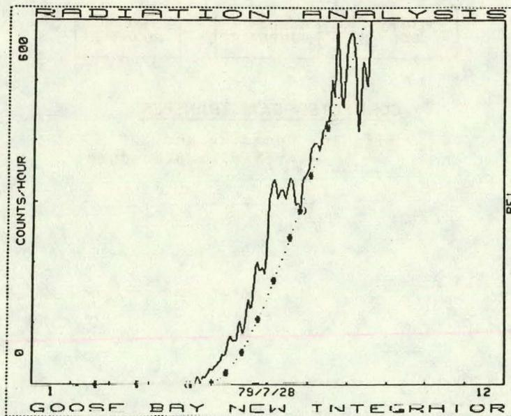
Fig. 12 Radiation trace with cursor points on clear sky reference curve
