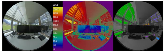
Figure 6. Representative workplace on April 8, 14:00 CEST, additional glare protection screens not activated:  $E_v = 2576\text{lx}$ ,  $DGP = 0.316$  („imperceptible glare“), maximum luminance: ca. 25.000 cd/m<sup>2</sup> in reflection at windowsill.
