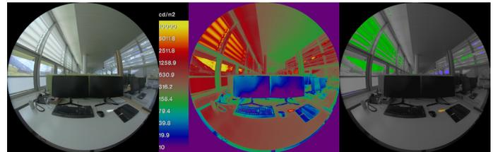
Figure 7. Representative workplace on April 8, 14:00 CEST, additional glare protection screens activated to block direct sunlight:  $E_v = 1898\text{lx}$ ,  $DGP = 0.274$  („imperceptible glare“), maximum luminance: ca. 15.000 cd/m<sup>2</sup> in bright cloud above mountain.
