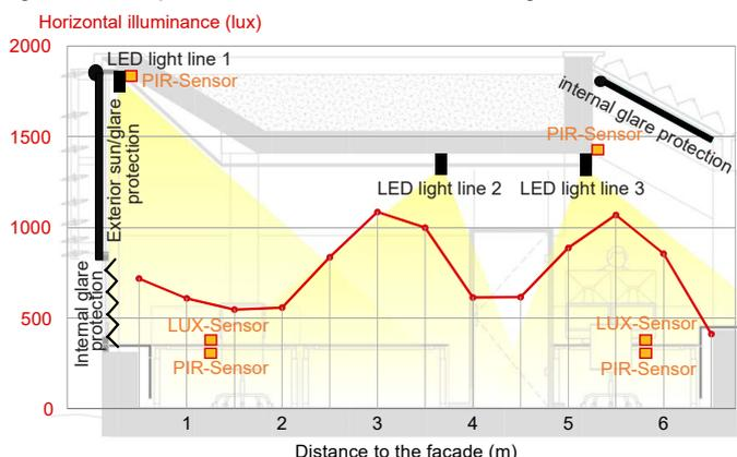
Figure 3. Position of light sensors, actuators, and maximum artificial illuminance. See Figure 2 for orientation of the office.
