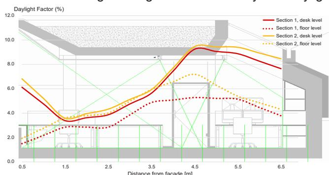
Figure 5. Distribution of Daylight Factor in the building section. Location of Section 1 and 2 is provided in Figure 2.
