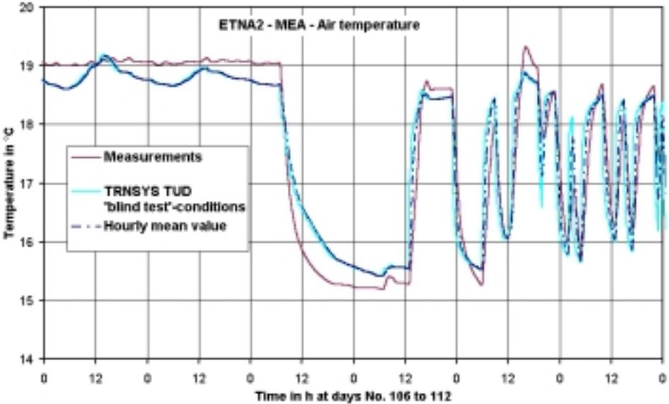
Figure 3 : Air temperature for MEASURE test cell. ETNA2
