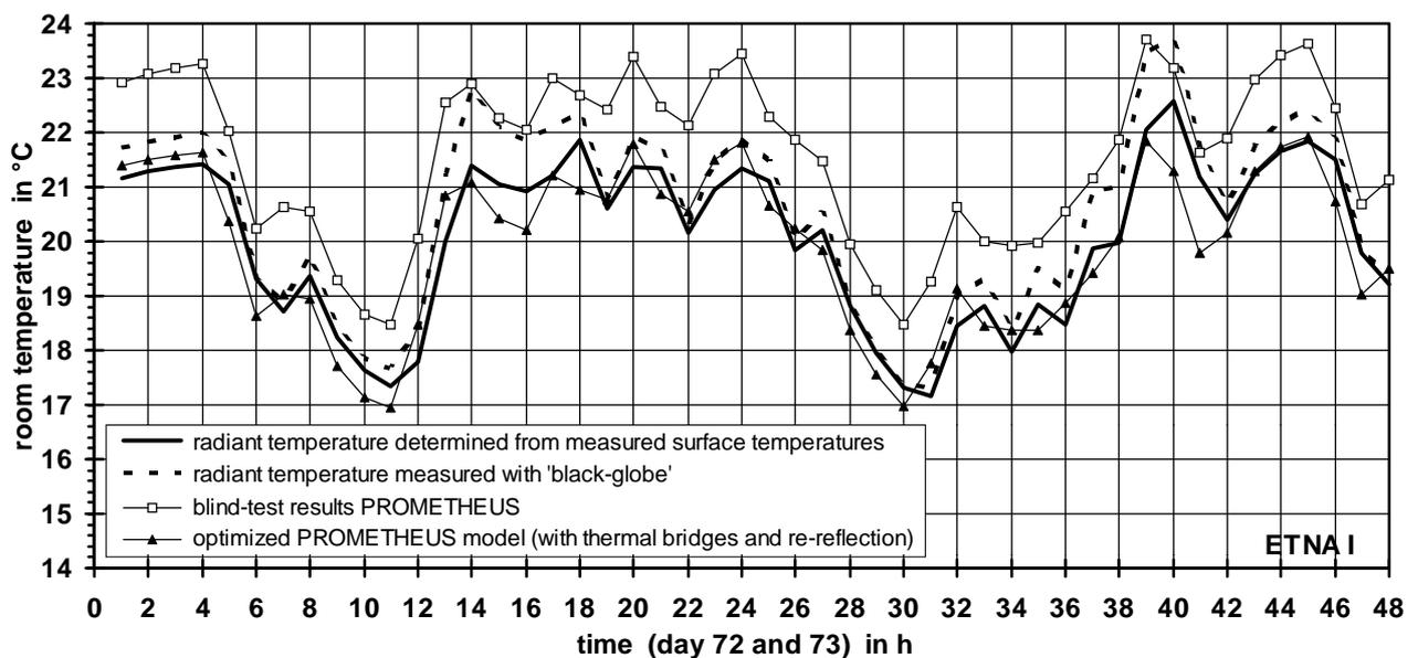
Figure 4 : Comparison of room temperature determined from measured surface temperatures and results of the optimized PROMETHEUS model (only 72<sup>th</sup> and 73<sup>th</sup> day)
