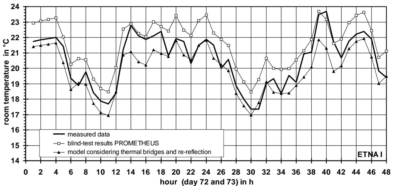
Figure 2 : Comparison of measured room temperature and results of the optimized PROMETHEUS model (only 72<sup>th</sup> and 73<sup>th</sup> day)
