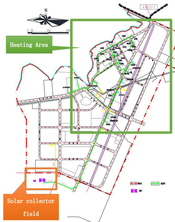
**Fig. 10. Solar collector field and the heating area**
