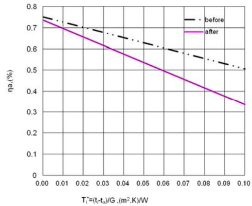
**Fig.4. thermal performance change of GSETC**
