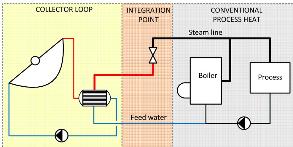
**Figure 10: SHIP system for indirect steam generation** (Helmke and Hess, in Muster-Slawitsch et al., 2015)
