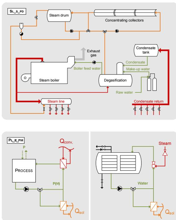
**Figure 3: Integration concepts for direct solar steam generation (above) and solar heating of a product or process media with external heat exchanger (below)** (Schmitt, in Muster-Slawitsch et al., 2015)
