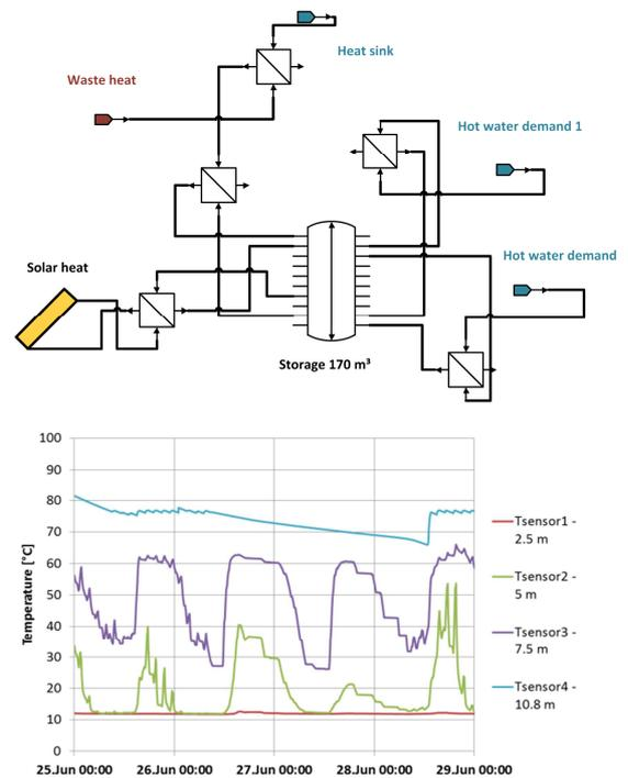
**Figure 2: Heat integration concept with solar heat and simulation result of a combined storage** (Krummenacher and Muster-Slawitsch, 2014)
