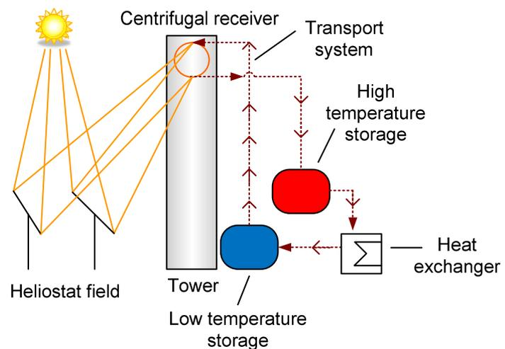
**Figure 15: Solar particle receiver – new high temperature concept** (Prosinecki, in Muster-Slawitsch et al., 2016)
