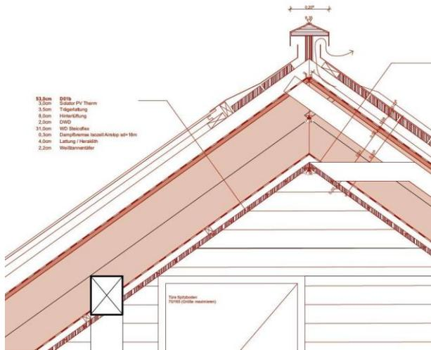
Figure 83: Roof structure with the integrated PV panels, ridge, © Bernhard Breuer Produktentwicklung Architektur Städtebau
