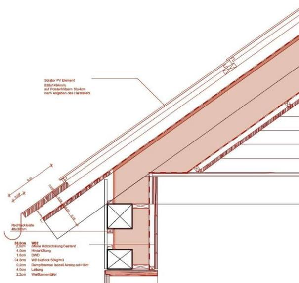
Figure 82: Roof structure with the integrated PV panels, eaves, © Bernhard Breuer Produktentwicklung Architektur Städtzsbau
