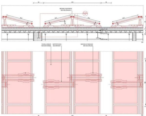
Figure 112: Palacinema Locarno. Connection system, © Greenkey Sagl
