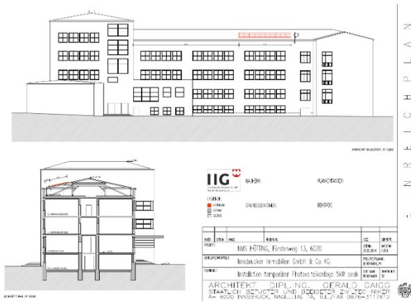
Figure 4 - Location of the PV-array (view from south-west and cross section), © IIG
