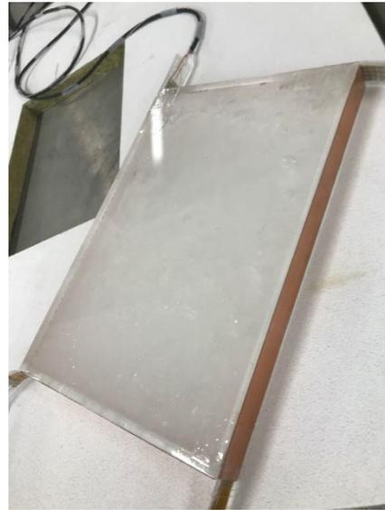
Figure 2: PMMA sample containing PCM with the lateral heat fluxmeters before installation in the insulation
