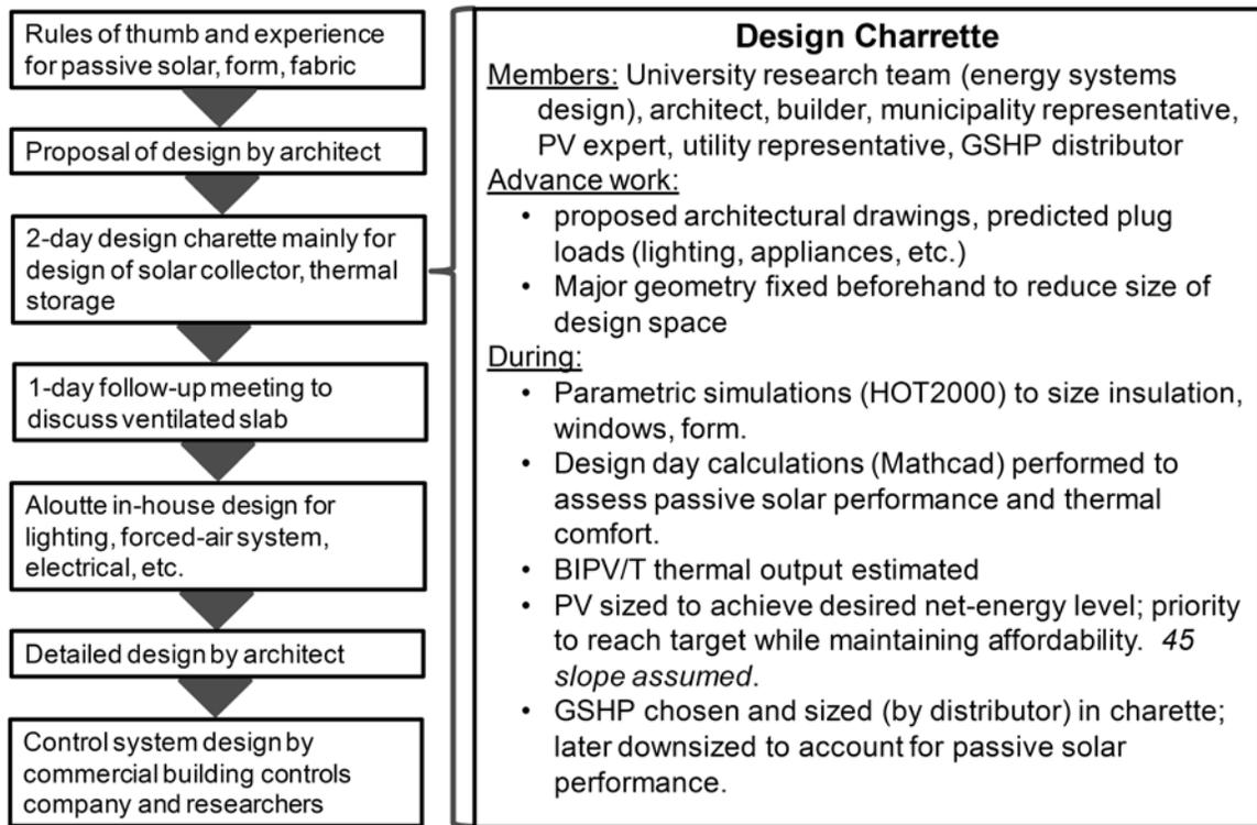
Figure 3: Design process outline for ÉcoTerra
