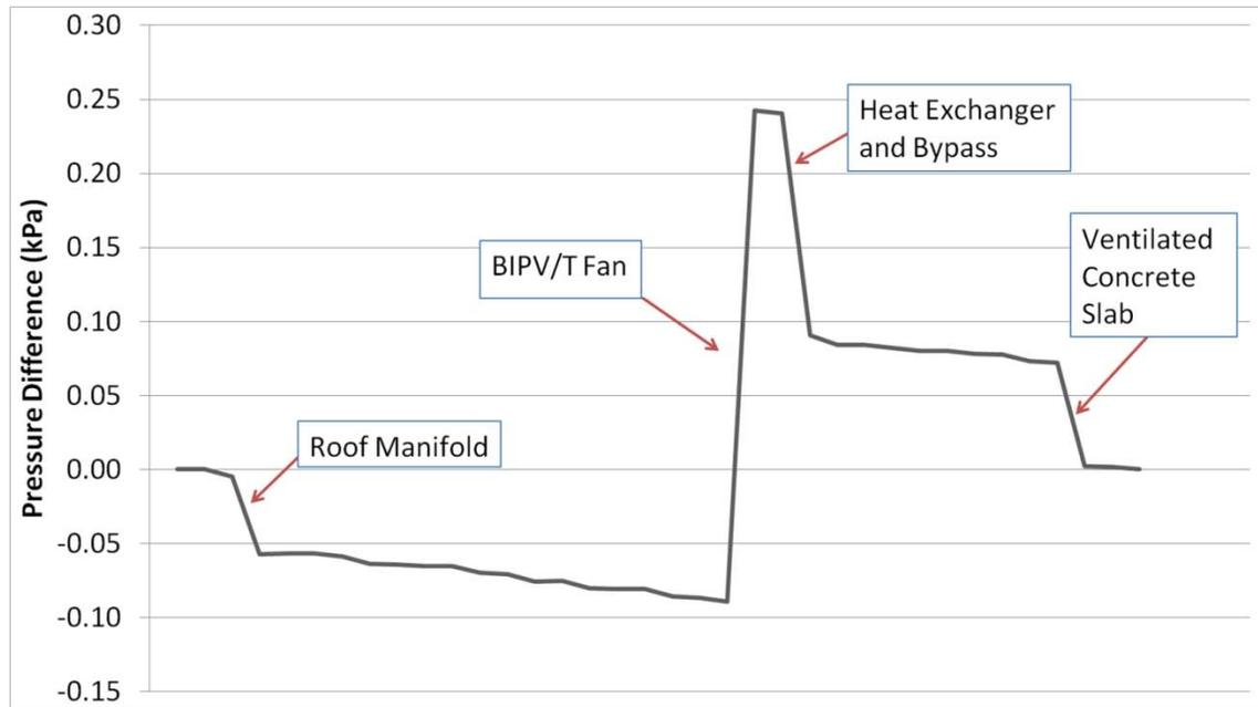
Figure 6: Pressure losses in the duct system for the1 estimated worst-case
