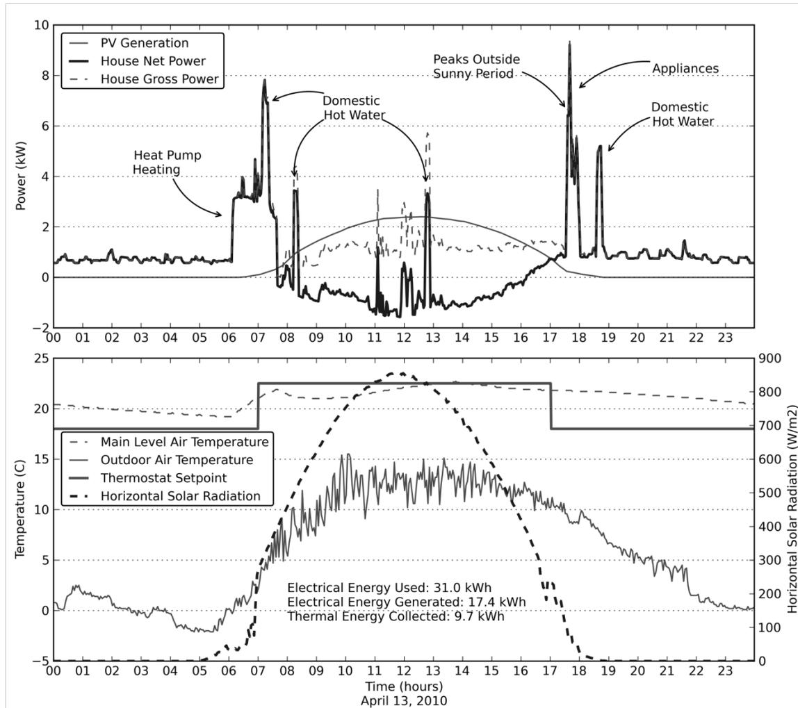
Figure 12: Sample electricity demand and generation profiles (April 13, 2010) (top) and weather conditions and indoor conditions (bottom).
