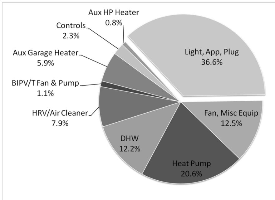
Figure 5: ÉcoTerra's existing, annual electricity end-use breakdown.
