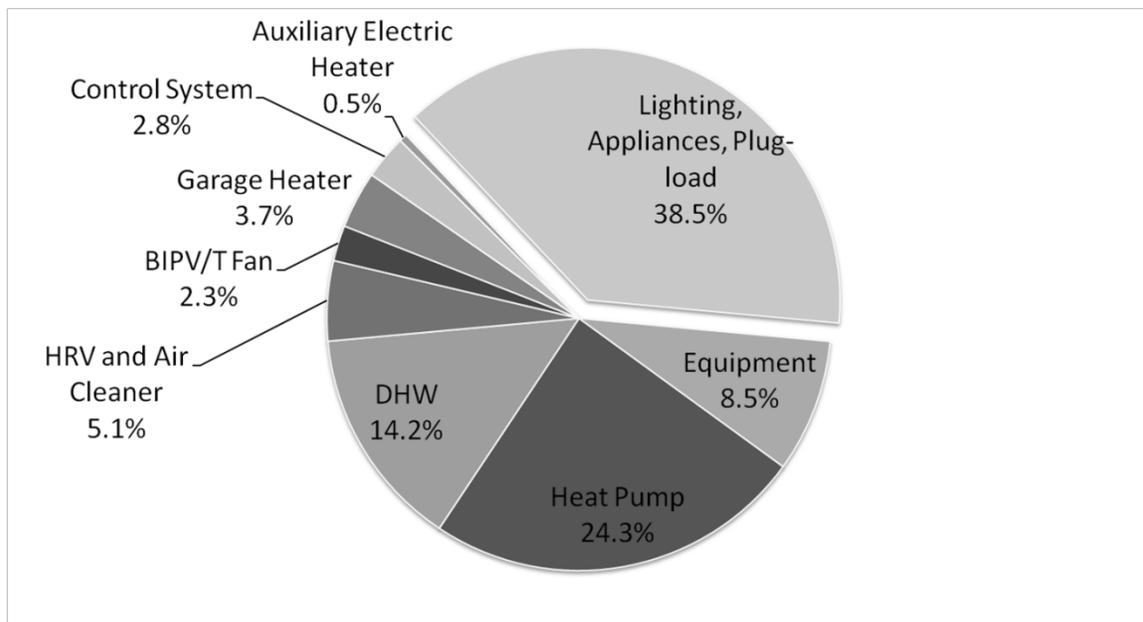
Figure 10: Potential energy end-use breakdown after potential improvements.
