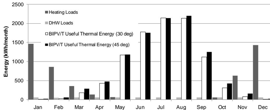
Figure 11: Comparison of thermal output of BIPV/T roof.
