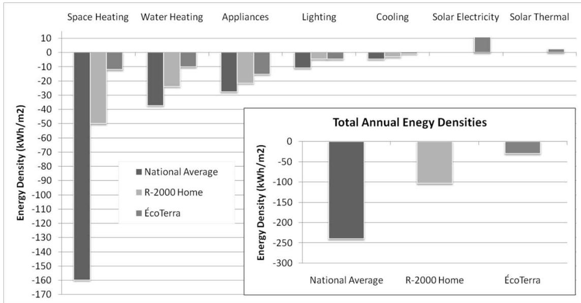
Figure 4: Comparison of ÉcoTerra with typical homes R-2000 is a successful energy efficiency standard that was established in Canada the 1980s that required significant savings primarily through envelope improvements and air tightness.
