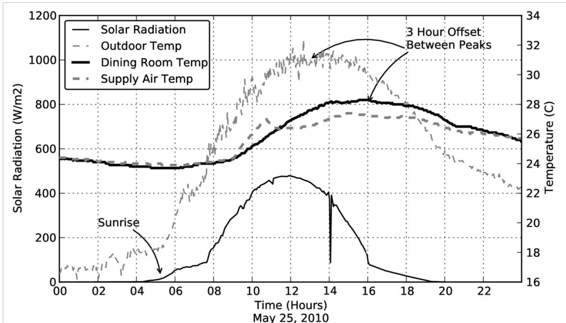
Figure 7: Solar radiation and indoor temperature – May 25, 2010
