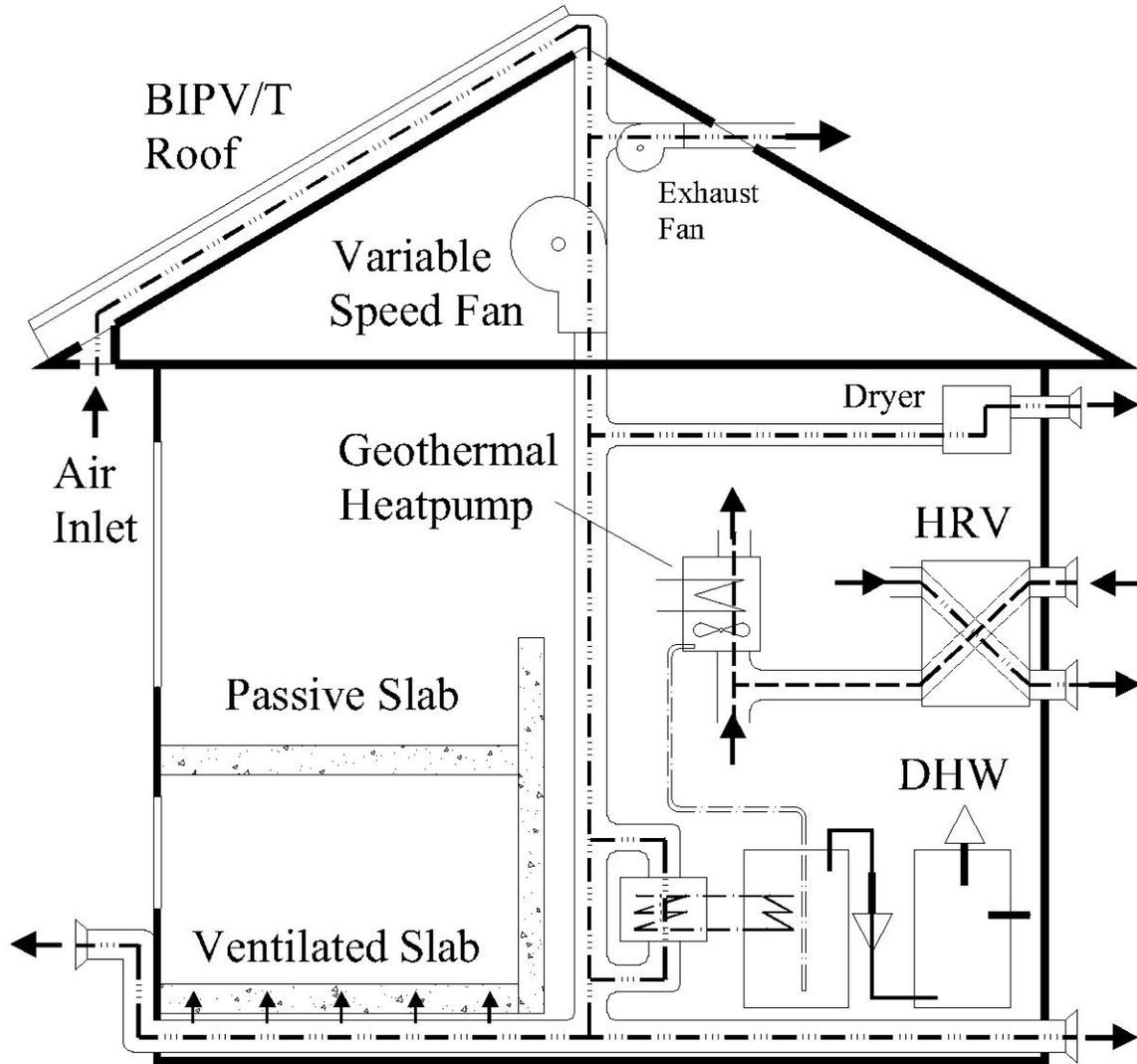
Figure 2: ÉcoTerra system schematic (Chen et al. 2010)
