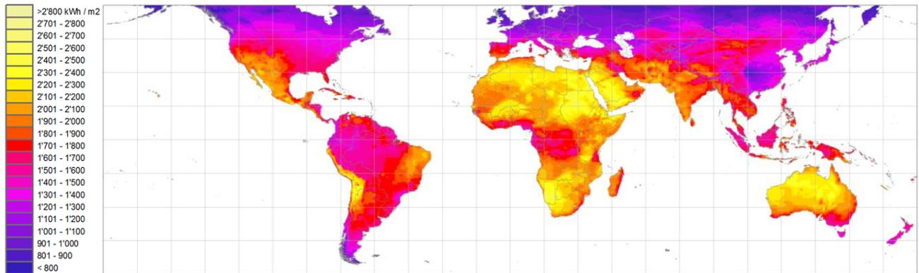
Figure 2: Yearly sum of Global Horizontal Irradiation (GHI); ; Source Meteonorm 7.0 ([www.meteonorm.com](http://www.meteonorm.com)); uncertainty 8%; Period 1986 – 2004; grid cell size: 0.25°
