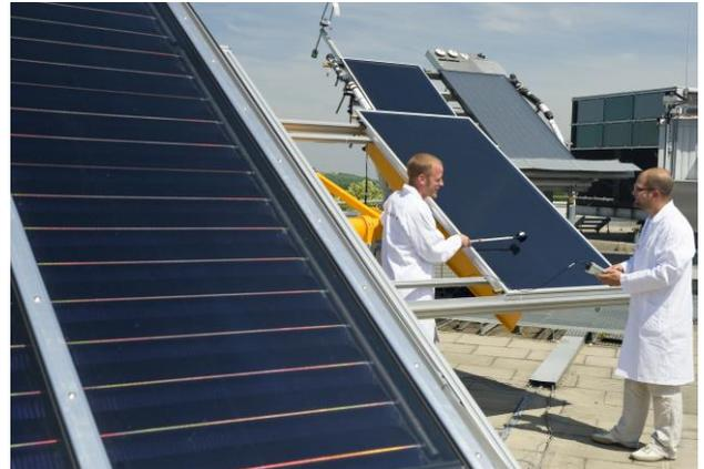
Figure 1: Test setup at TestLab Solar Thermal Systems, Fraunhofer ISE.
