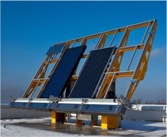
Figure 1: Typical outdoor test facility, Fraunhofer ISE
