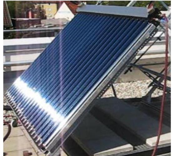
Figure 1: Internal thermal shock test; Fraunhofer ISE
