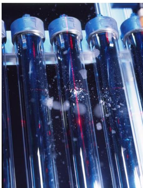
Figure 2: Collector after ice ball impact test
