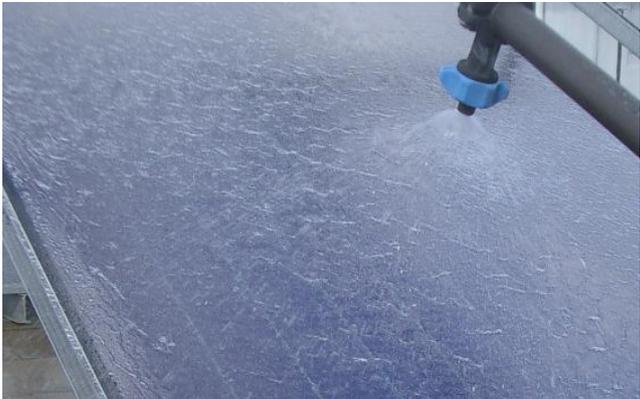
Figure 1: External Thermal Shock Test; Fraunhofer ISE
