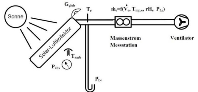
Figure 3: Open to ambient test layout for SAHC
