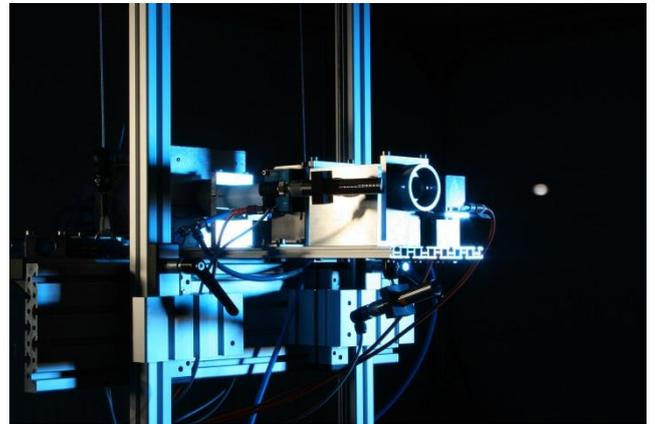
Figure 1: Impact resistance testing facility at Fraunhofer ISE
