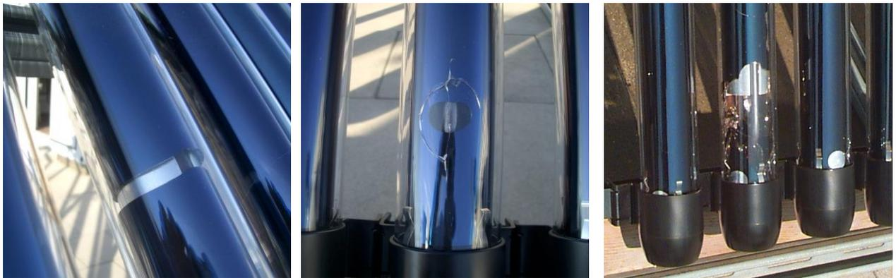
Figure 2: Damaged collectors after testing; Fraunhofer ISE
