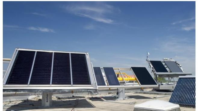
Figure 1: Outdoor exposure at the testing facility of Fraunhofer ISE
