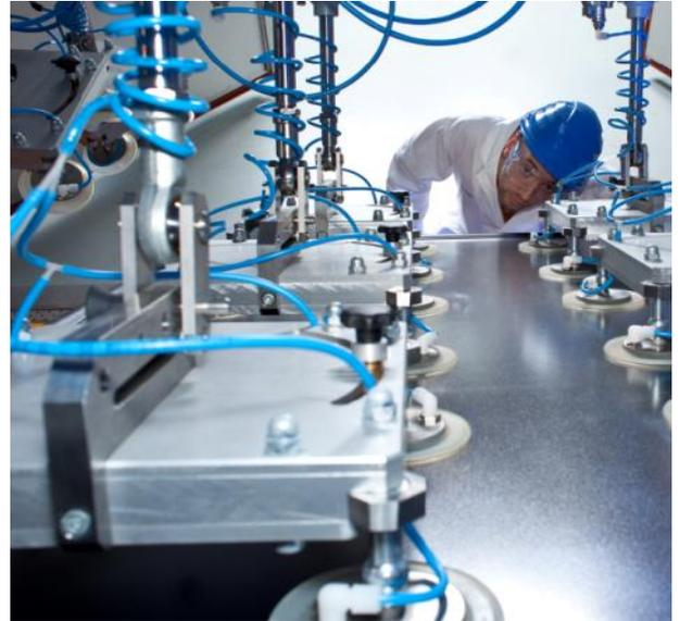
Figure 1: Mechanical load test; Fraunhofer ISE
