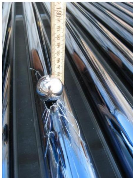
Figure 3: Damaged collector after steel ball impact test
