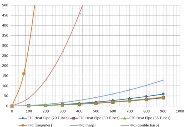
Figure 2: Typical pressure drop values for different SLHCs
