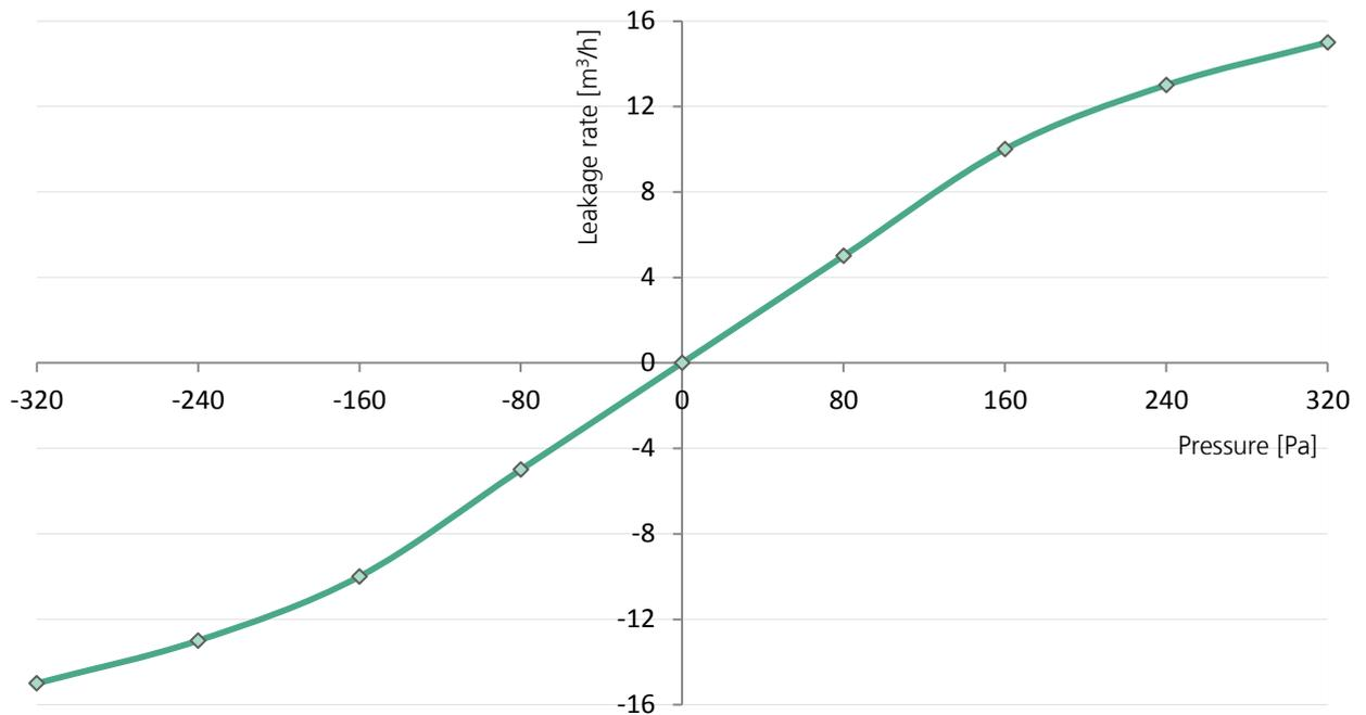
Figure 2: Typical Leakage rate curve fitted with a 3<sup>rd</sup> order polynomial on the basis of flow measurement points for positive and negative pressures.
