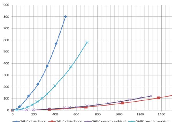
Figure 3: Typical pressure drop values for different SAHCs
