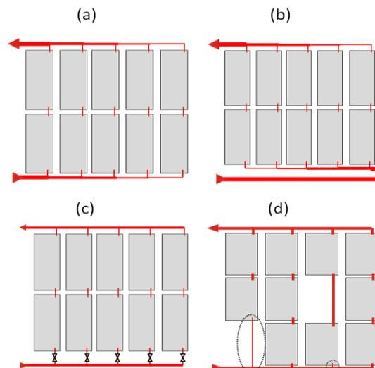
Example: Methods for achieving a homogeneous mass flow distribution. (a) Adjustment of the supply and return pipes diameters. (b) Tichelmann connection in combination with adjustments to the pipe diameters. (c) Installation of mechanical balancing valves. (d) Adjustment of the collector connecting pipe diameters.
