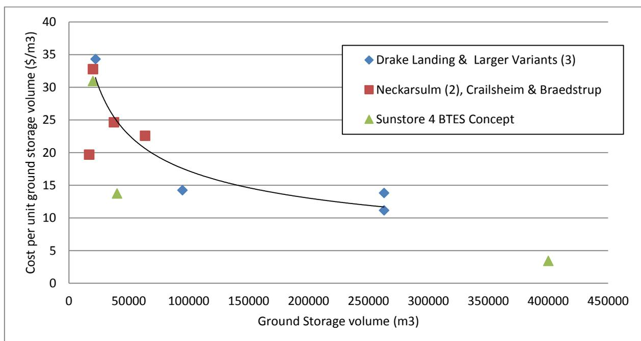
Figure 10. Specific installed cost for several borehole thermal energy storages
