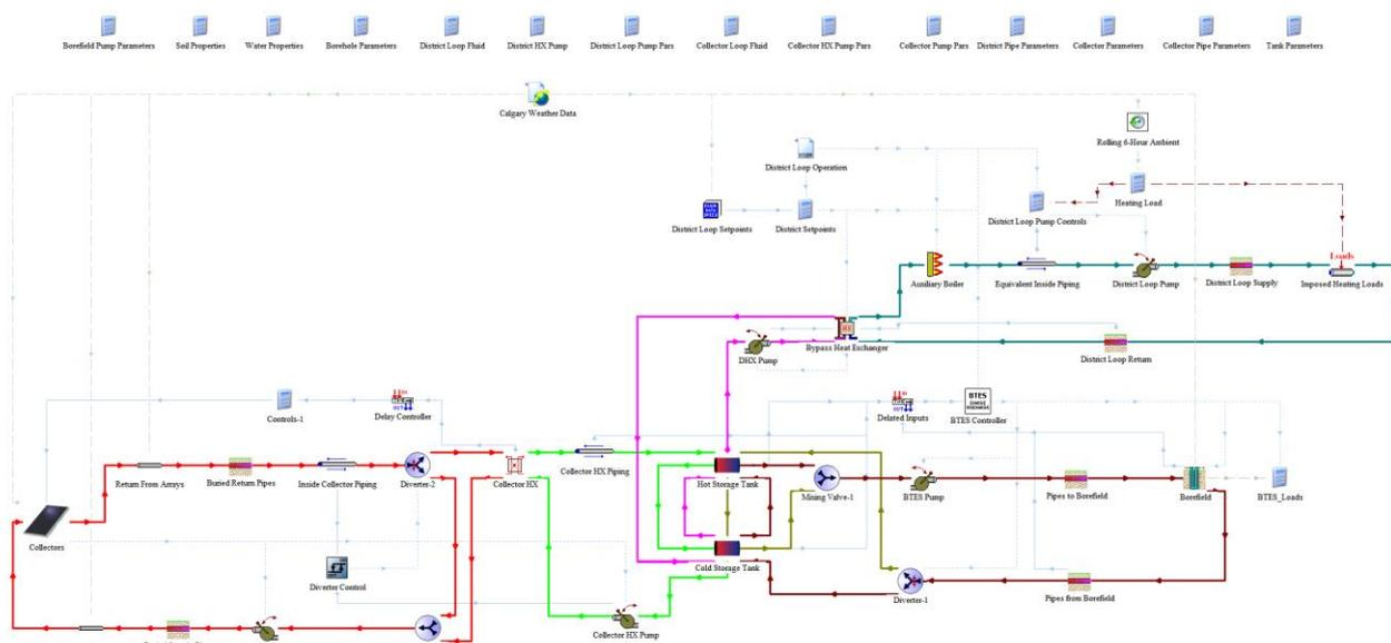
Figure 9. Graphical interface representation of the simplified TRNSYS model of the seasonal solar district heating system at Drake Landing using a BTES.
