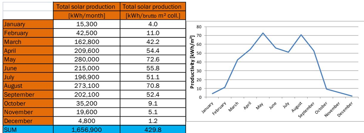
Figure 7. Measured solar output
