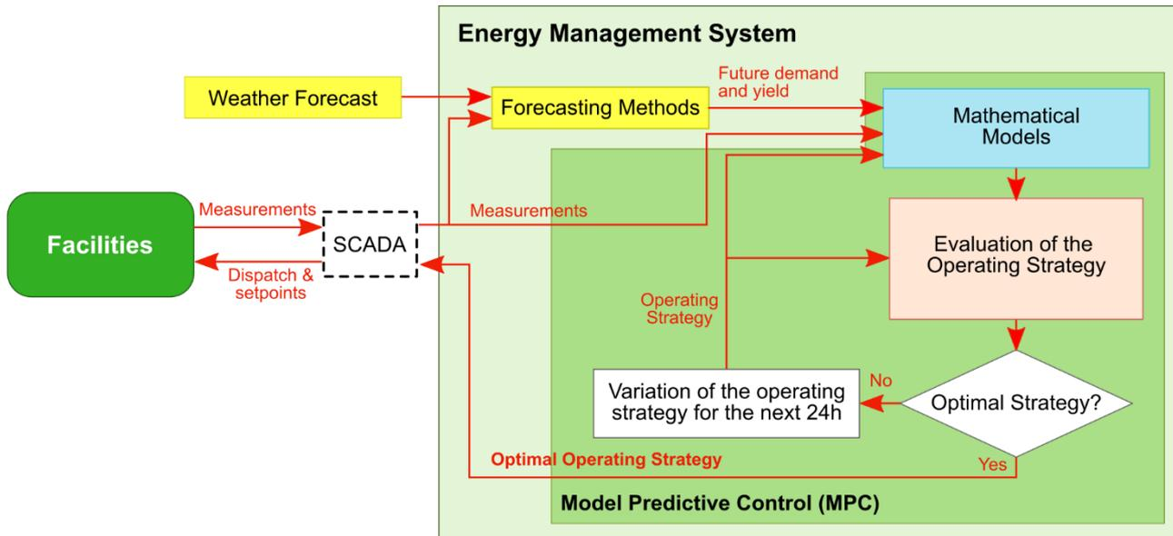
Figure 3: Structure of an optimization-based predictive supervisory control (Energy Management System)
