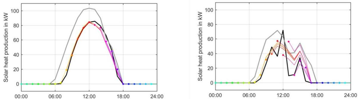
Figure 4: Exemplary forecasts for the solar heat production of a large-scale solar thermal plant
