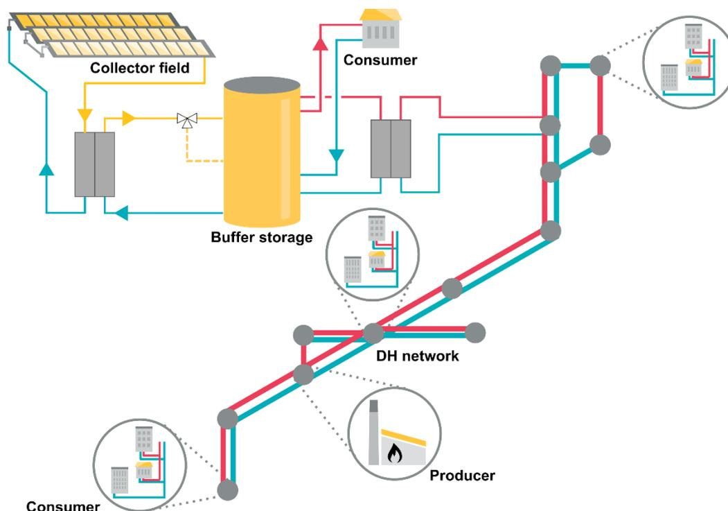
Figure 1: Scheme of a typical large-scale solar thermal system with a decentral, bi-directional connection to a DH network
