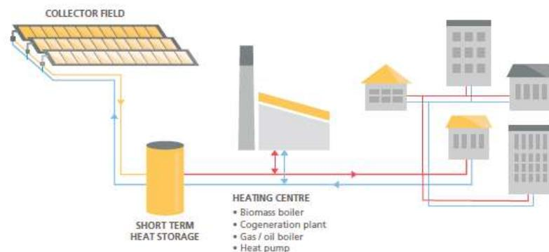
Example of a simple large-scale solar thermal system integration into district heating.
