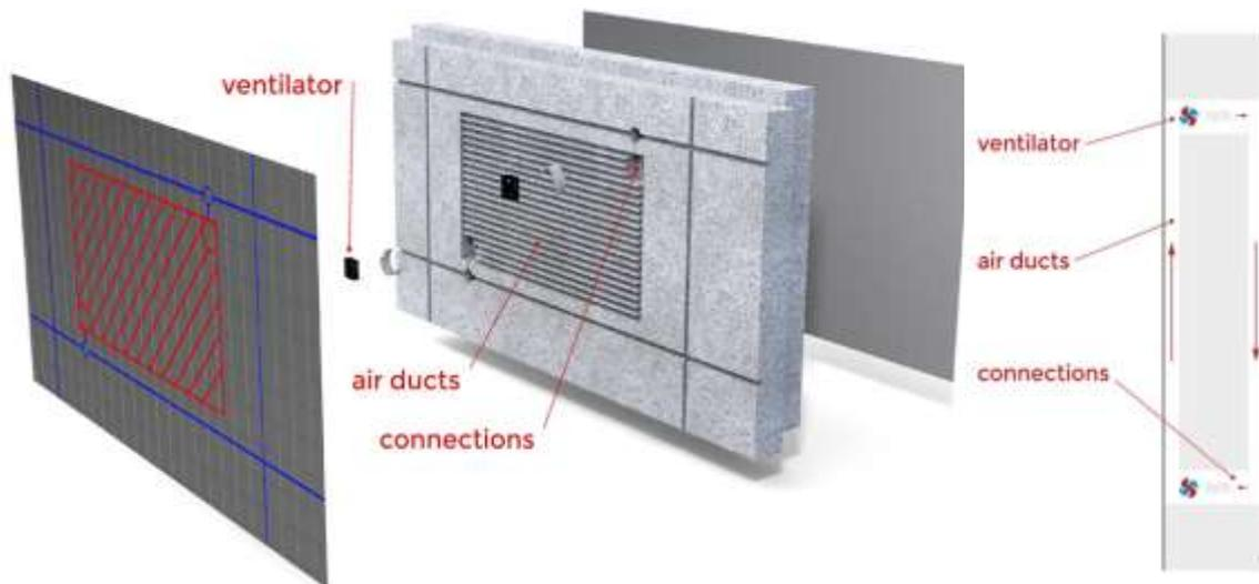
Figure 5. Schematic working principle of Active Insulation.
