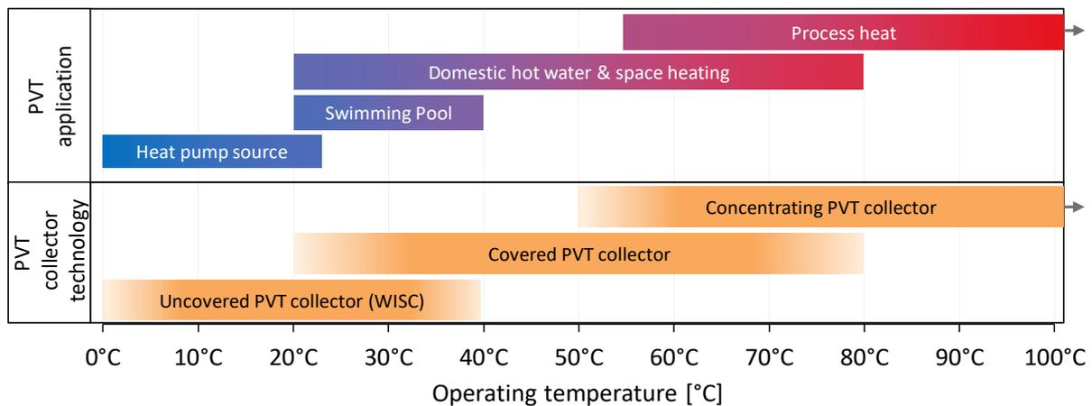
**Figure A.2: Map of PVT collector technologies and application as function of the application temperature based on median values for the minimum and maximum temperatures of the collector and application ranges.**
