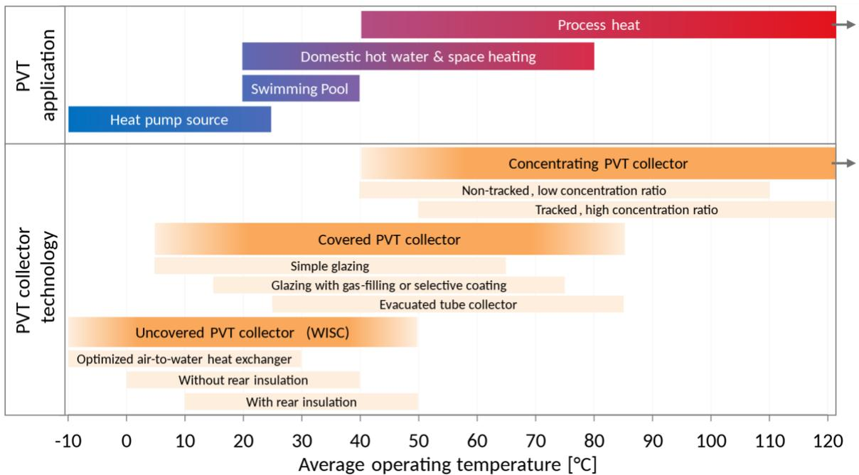
Figure A.4: Extended map featuring further sub-classification of collector technologies. Temperature ranges based on the 25<sup>th</sup> percentile for the minimum boundary and 75<sup>th</sup> percentile for the maximum boundary. <sup>27</sup>
