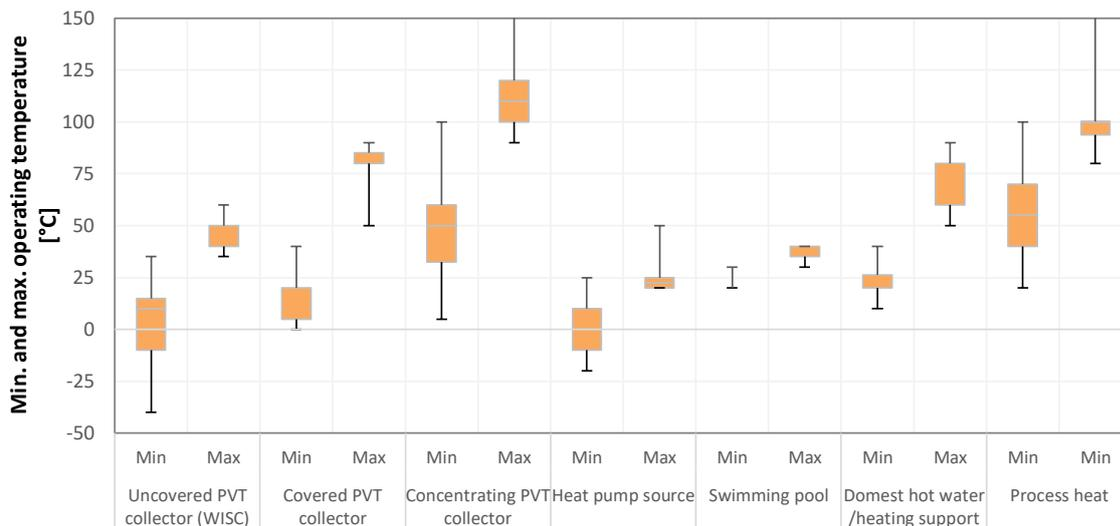
**Figure A.1: Box plot diagram of the survey responses, boxes represent the 25<sup>th</sup> and 75<sup>th</sup> quantile and the median, and the error indicators represent the absolute minimum and maximum values.**
