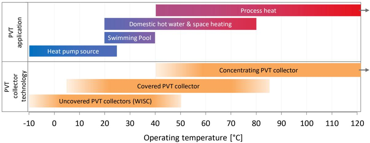
Figure A.3: Map of collector technologies and applications with 25<sup>th</sup> percentile for the minimum boundary and 75<sup>th</sup> percentile for the maximum boundary
