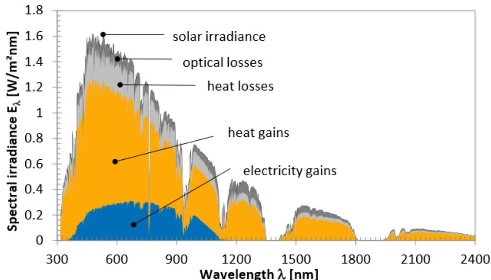
**Figure 1.2: Utilization of the electromagnetic solar spectrum by a PVT collector.<sup>11</sup>**
