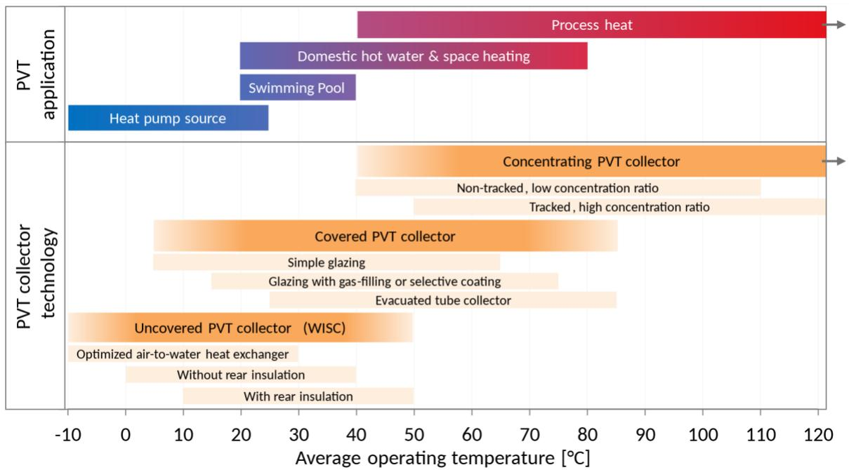
**Figure 1.3: Map of PVT collector technologies and PVT applications per operating temperature.<sup>21</sup>**
