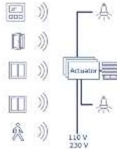
Figure 9. Centralized Control System (Source:EnOcean Alliance).
