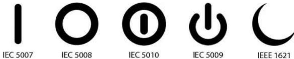
Figure 6. Examples of Power, Standby and Sleep symbols and relevant sources.<sup>6</sup>
