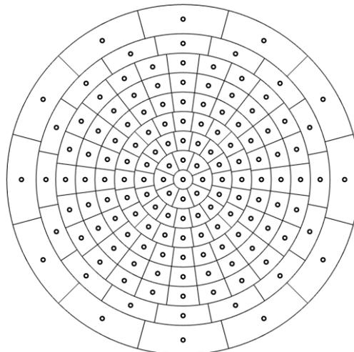
Figure 2. Klems BSDF angular basis [Klems 1994] for incident / exiting hemispheres.
