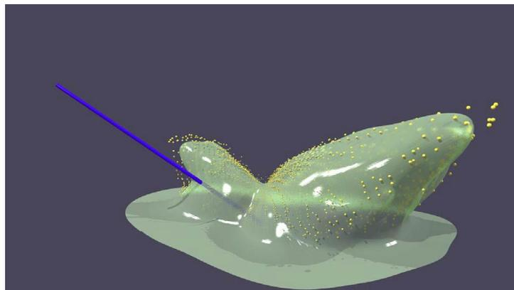
Figure 7. Fitting of an interpolant RBF model (green) to a set of measured values (yellow points), log scale. Source: G. Ward [Lee 2018].
