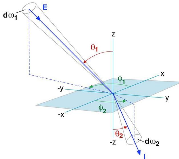
Figure 1. Polar and azimuthal angles of incident and exiting directions. Source: LBNL.
