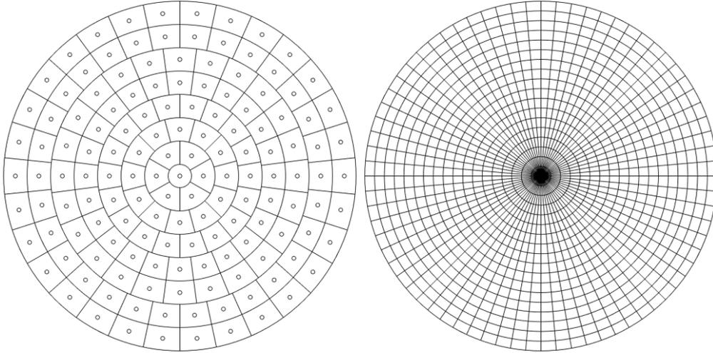
Figure 3. IEA21 BSDF angular basis [IEA 1999] for incident (left) and exiting (right) hemispheres.
