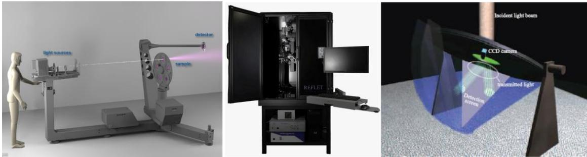
Figure 6. Examples of goniophotometer measurement setups: left: pab Ltd Gonio-Photometer II; center: Lighttec Reflet 180S; right: LESO-PB / EPFL video-goniophotometer. Sources: [pab 2020], [Light Tec 2020], [Andersen 2005].
