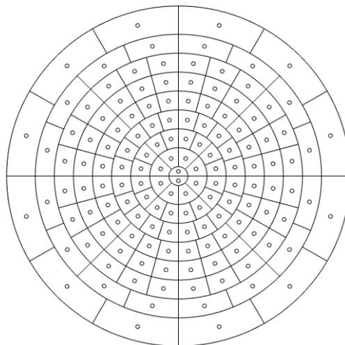
Figure 4. McNeil BSDF angular basis [McNeil et al. 2017] for incident / exiting hemispheres.
