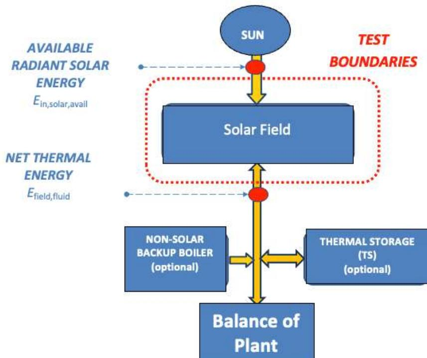
**Figure 1:** General diagram of the Solar Field Test Boundary
