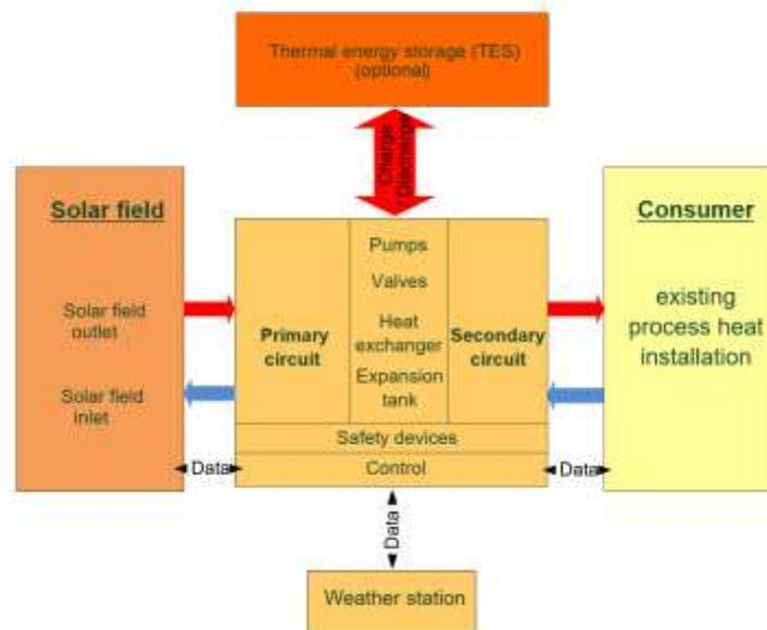
**Figure 3:** BoP function modules and interfaces
