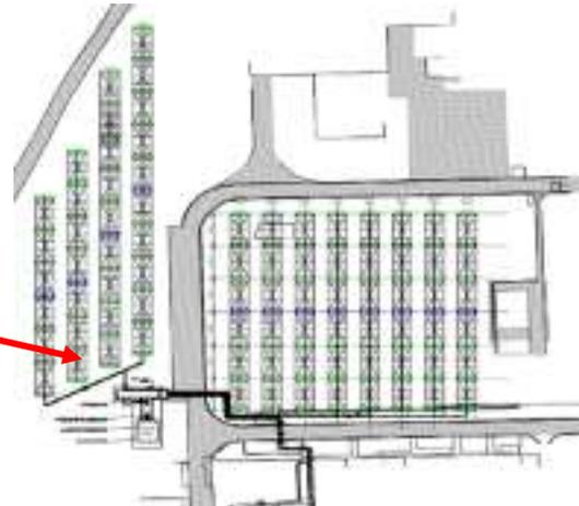
**Figure 10:** Solar field layout for Turnhout, Belgium (right). Each cross indicates a collector module
