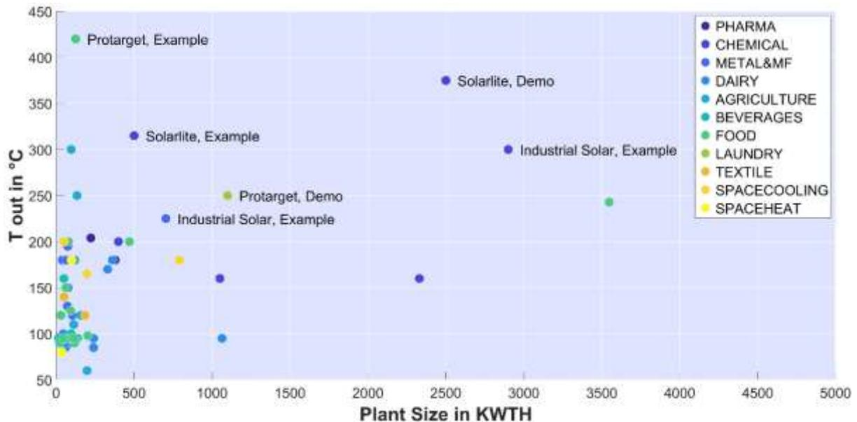
**Figure 4:** System power and process temperature of exemplarily selected process heating systems already installed (Example) by the project partners and planned in Modulus (Demo), in comparison to systems registered in ship-plants.info
