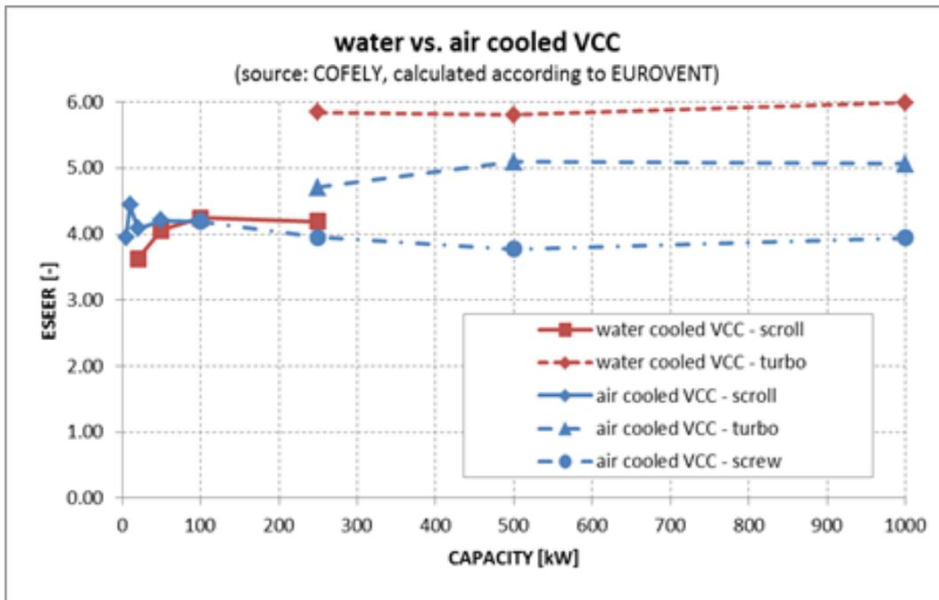
**Figure 2: Reference efficiency for air/water cooled vapour compression chillers**
