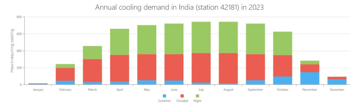
Figure 5: Climate Profiling Tool: monthly cooling hours according to the set threshold (22°C) value for the selected location (New Delhi / Palam)
