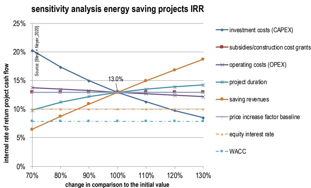
**Figure 9: LCCBA sensitivity analyses: project IIR = f(input data ±30%) (Sources: Energetic Solutions)**
