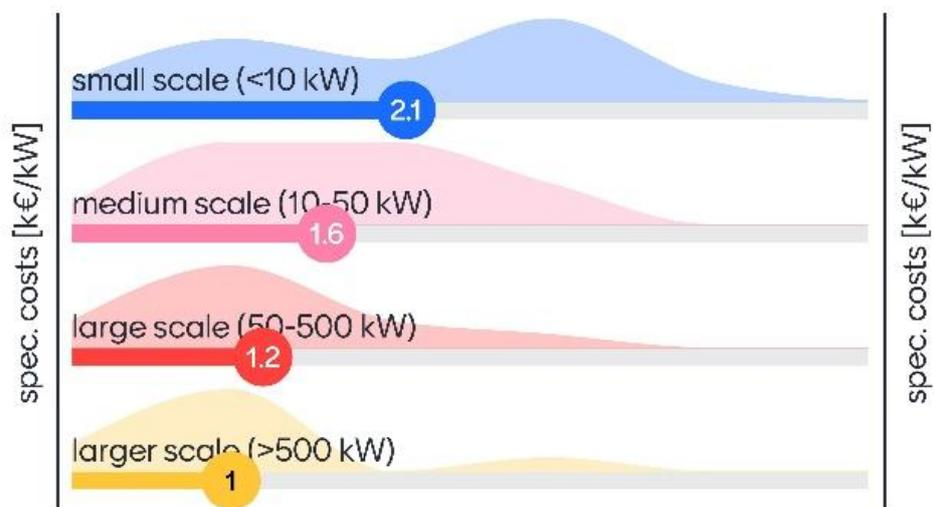
**Figure 1: Estimated system costs for small (<10 kW), medium (10–50 kW), large (50–100 kW) and larger (>500 kW) ST cooling systems; elaborated during a Task 65 expert meeting**
