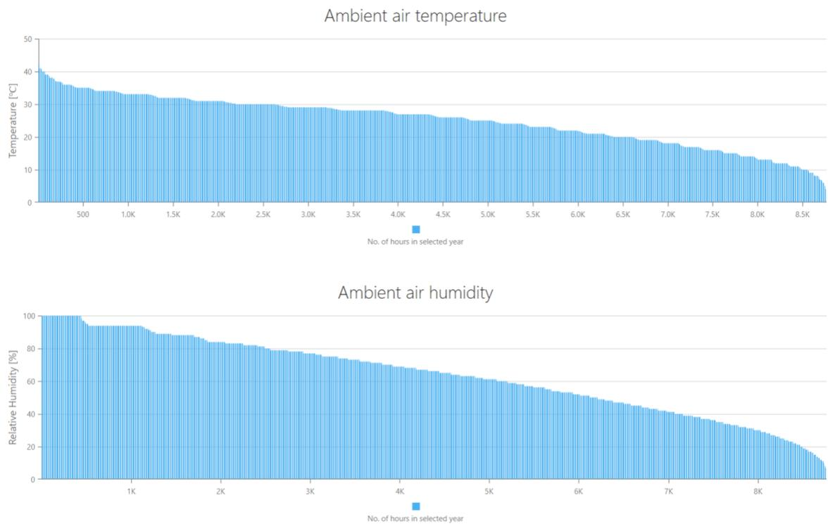
**Figure 6: Climate Profiling Tool: sorted ambient air temperature and humidity for the selected location**
