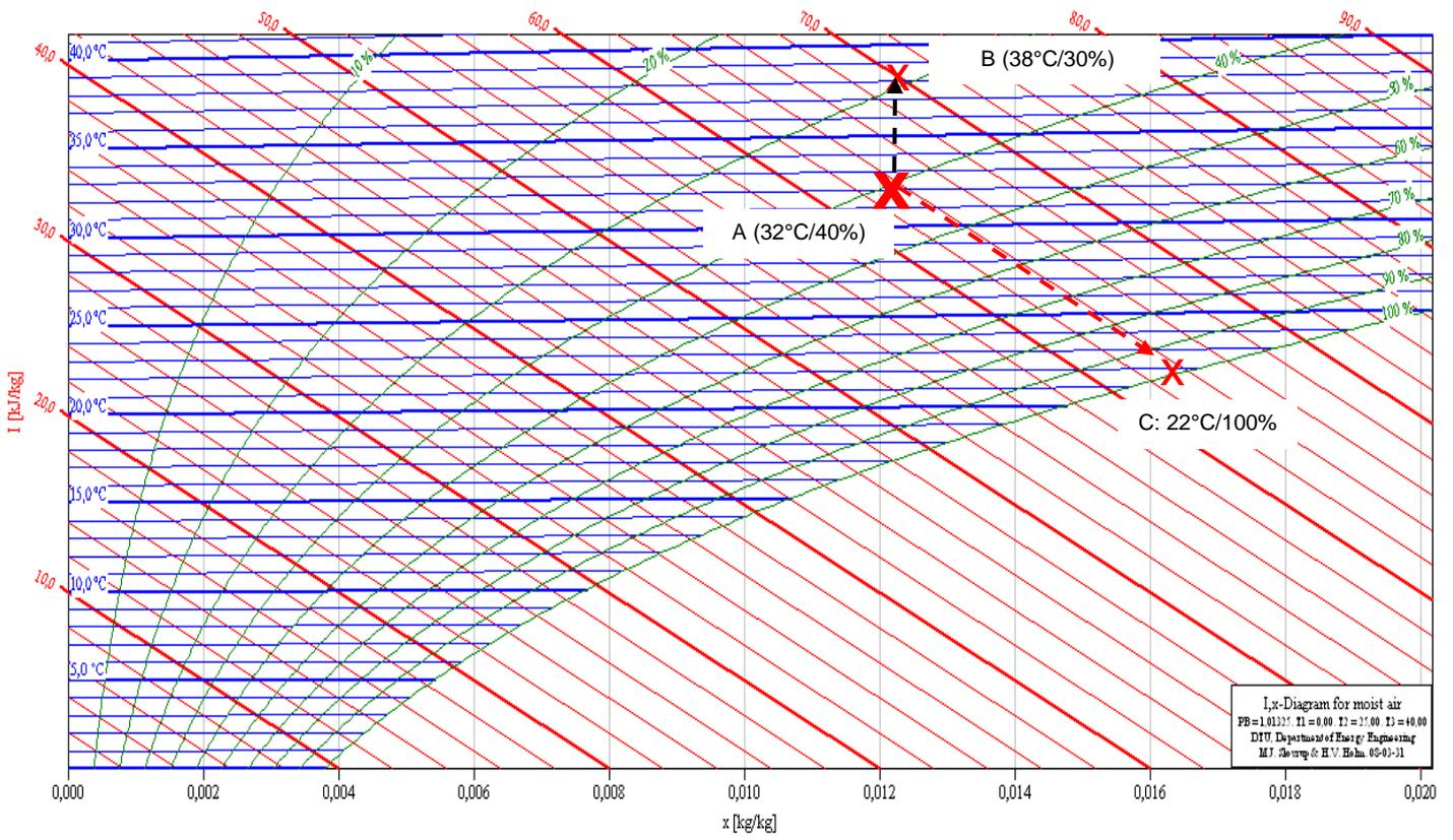
Fig. 2: The temperature change of the air in a dry cooler: A: Ambient condition, B outlet temperature from dry cooler and C wet bulb temperature of the ambient condition
