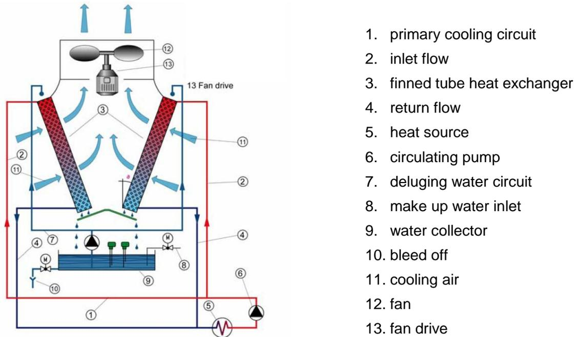
Fig. 9: Sketch of a hybrid dry cooling system (Jaeggi, [http://www.guentner.ch/pdfs/Evaluation of Aircooled Cooling Systems.pdf](http://www.guentner.ch/pdfs/Evaluation%20of%20Aircooled%20Cooling%20Systems.pdf), 26.03.2009)
