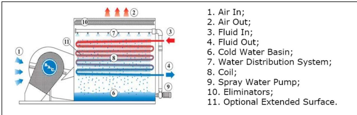
Fig. 4: Sketch of a closed cooling tower (BAC type VFL, [www.baltimoreaircoil.be](http://www.baltimoreaircoil.be))
