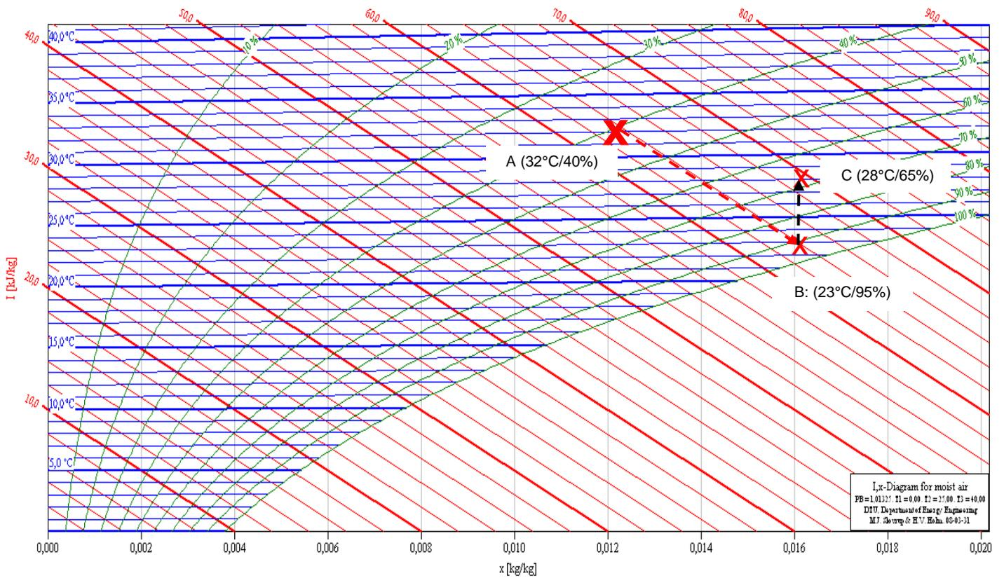
Fig. 8: The temperature change of the air in a evaporative pre cooled dry cooler: A: Ambient condition, B outlet temperature from dry cooler and C wet bulb temperature of the ambient condition
