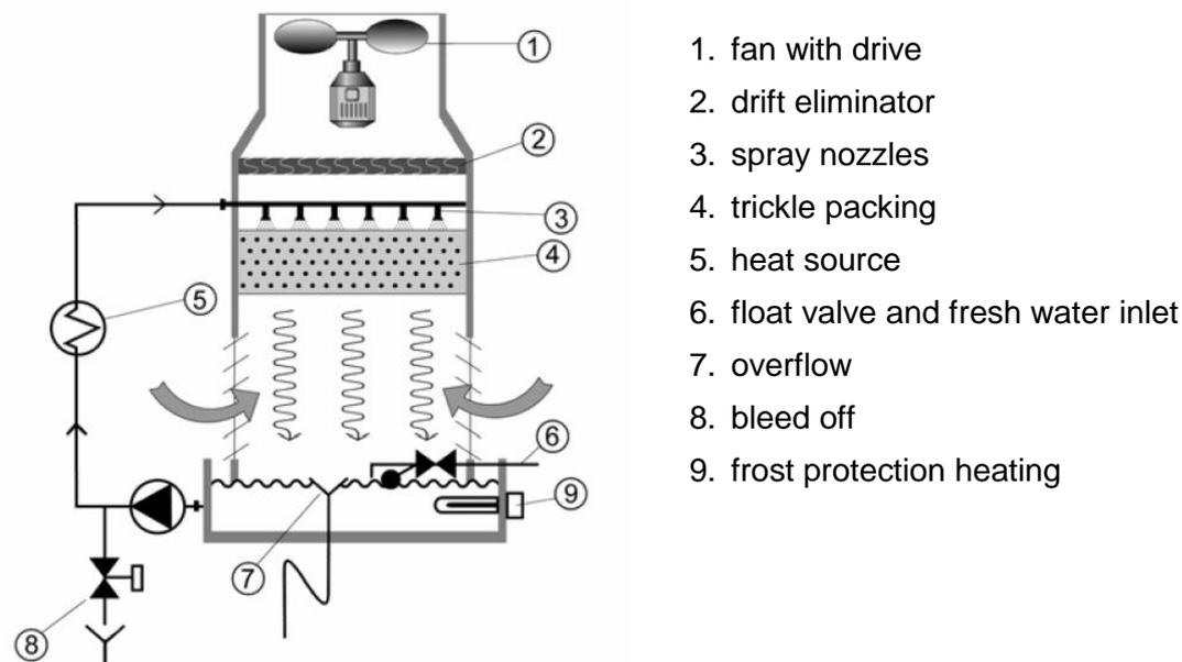
Fig. 3: Sketch of a open cooling tower (Jaeggi, [http://www.guentner.ch/pdfs/Evaluation of Air-cooled Cooling Systems.pdf](http://www.guentner.ch/pdfs/Evaluation%20of%20Air-cooled%20Cooling%20Systems.pdf), 26.03.2009)
