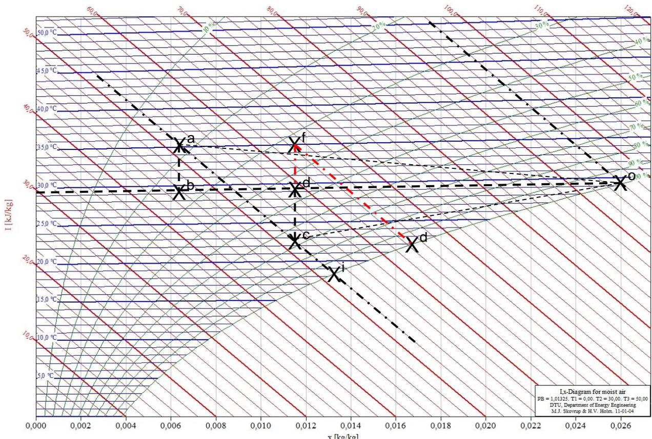
Fig. 6 Open cooling tower: Impact of ambient temperature and humidity
