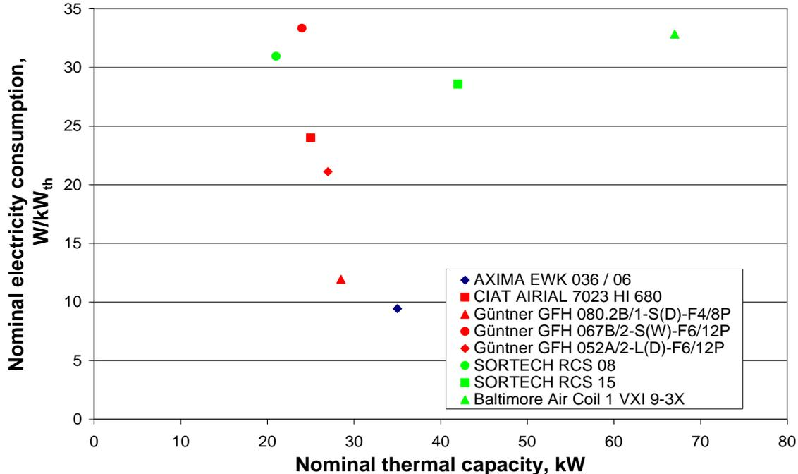
Fig. 11: Nominal electricity consumption of heat rejection systems installed in Task 38 monitoring installations in Watts per kW rejected heat
