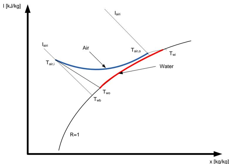
Fig. 5 IX diagram showing the air process in the cooling tower
