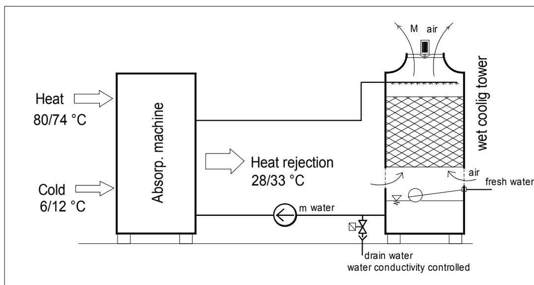
Figure 3-1: Principle of a thermal driven cooling with wet heat rejection
