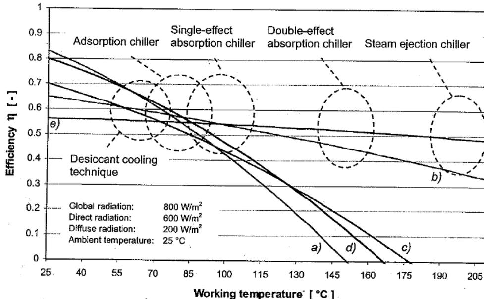
Figure 3: Comparison of different collectors at 800 W/m<sup>2</sup>. a) Single glazed flat-plate with AR, b) Evacuated tube collector of the Sydney type, c) CPC flat-plate with Teflon foil, d) Flat-plate with double AR-glazing and inert gas filling, e) Small parabolic trough (under development; only the fraction of direct radiation = 600 W/m<sup>2</sup> can be used). The values are for normal irradiance and refer to the aperture area.
