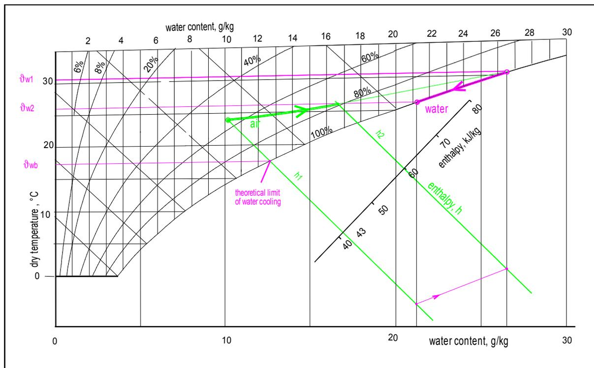
Figure 3-2: States of the air and temperatures of the cooling water inside of the cooling tower
