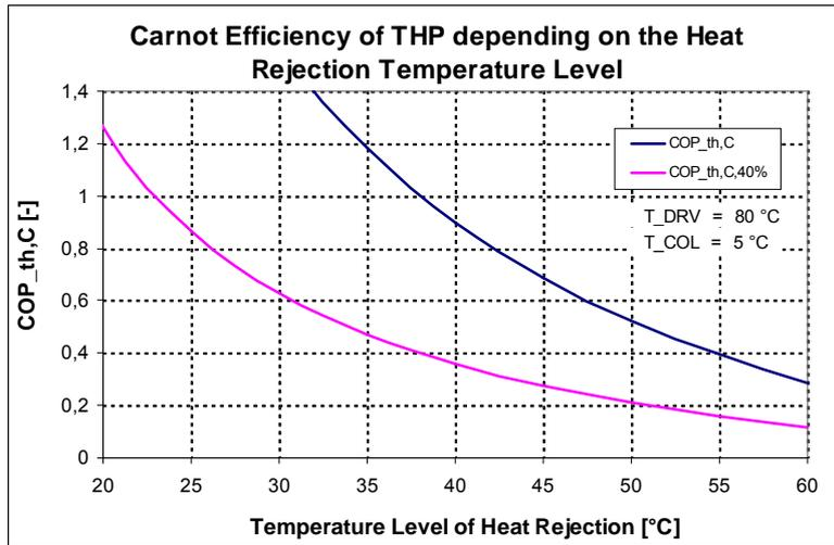
Figure 1-3: Carnot efficiency for different temperature levels of the heat rejection system ( $T_{DRV}=80^{\circ}\text{C}$ ,  $T_{COL}=5^{\circ}\text{C}$ )
