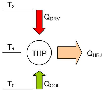
Figure 1-1: Sketch of heat flows and temperature levels for a thermally driven heat pump
