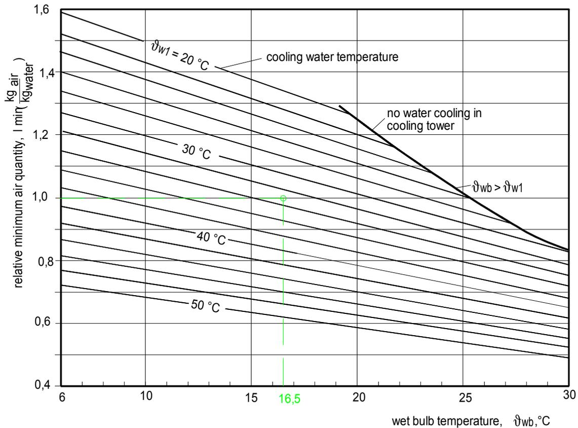
Figure 3-3: Relative minimum quantity of air (Recknagel Sprenger, 1997/98)
