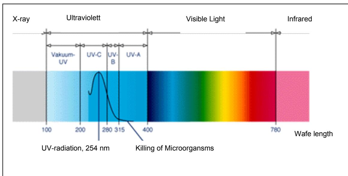
Figure 5-3: Position of the UV-C radiation in the frequency band from 100 to 750 nm
