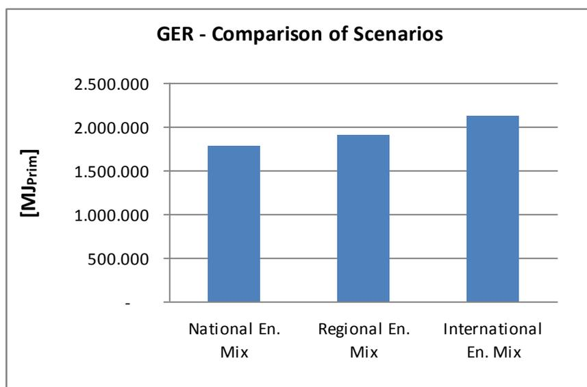
Figure 51: Comparison of GER values due to different electricity eco-profiles
