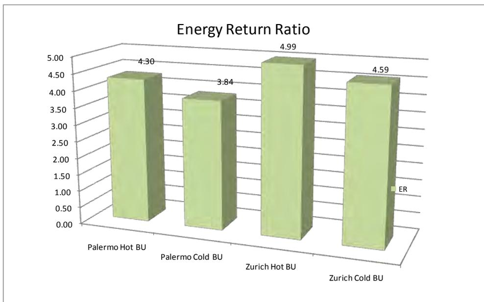
Figure 27:  $E_{RR}$  for Absorption Solar Cooling systems with hot and cold back-up
