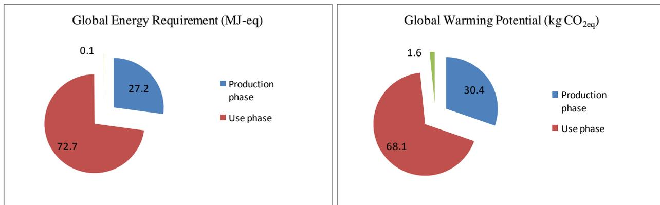
**Figure 15: Percentage contribution of different phases of the plant life-cycle to GER and GWP for Palermo**
