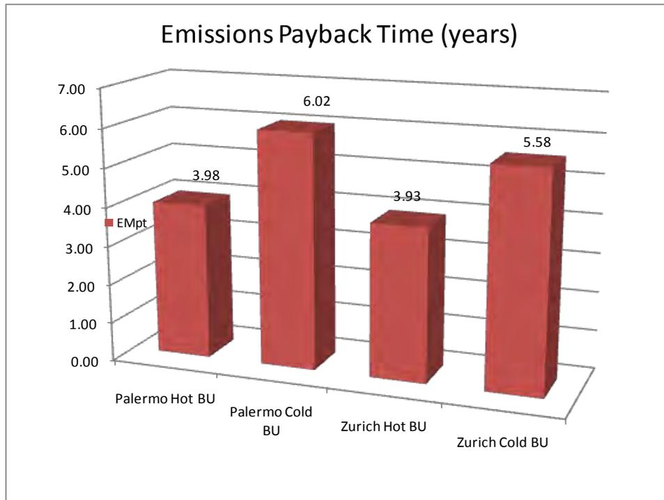
Figure 26: Emissions Payback Time for Absorption Solar Cooling systems with hot and cold back-up
