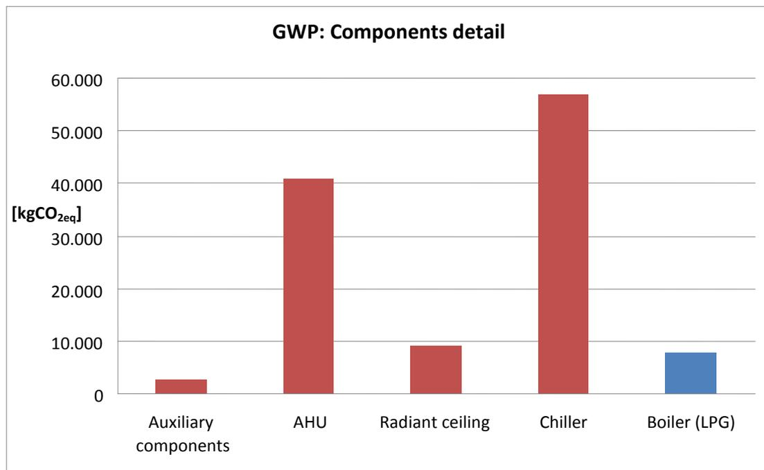
Figure 50: Comparison of impacts related to system components (GWP)
