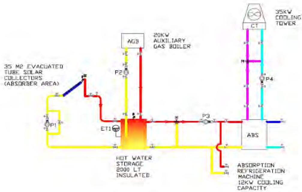
**Figure 4: Schematic representation of the absorption chiller plant (hot backup configuration)**
