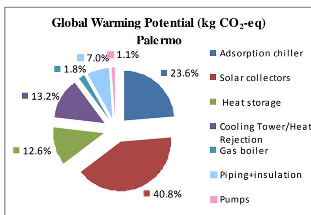
**Figure 31: Production phase: Percentage contribution of different plant components to GER and GWP for Palermo**
