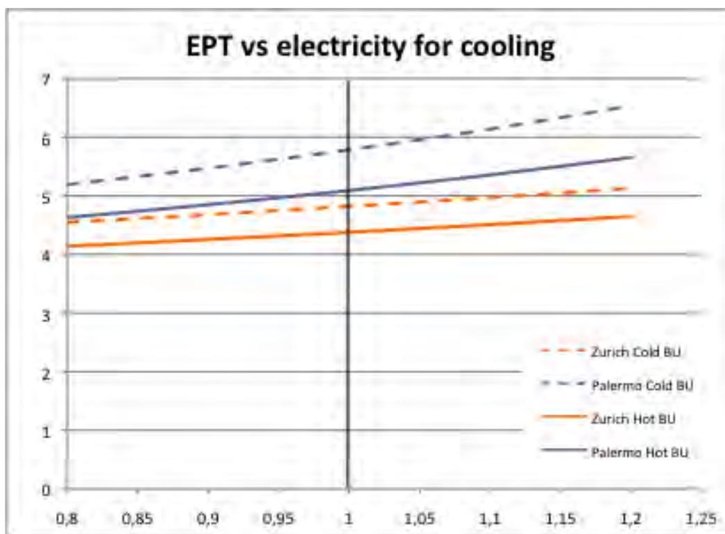
**Figure 24: Relationship between  $E_{PT}$  and electricity consumption for cooling operation for Absorption Solar Cooling system with hot and cold back-up**
