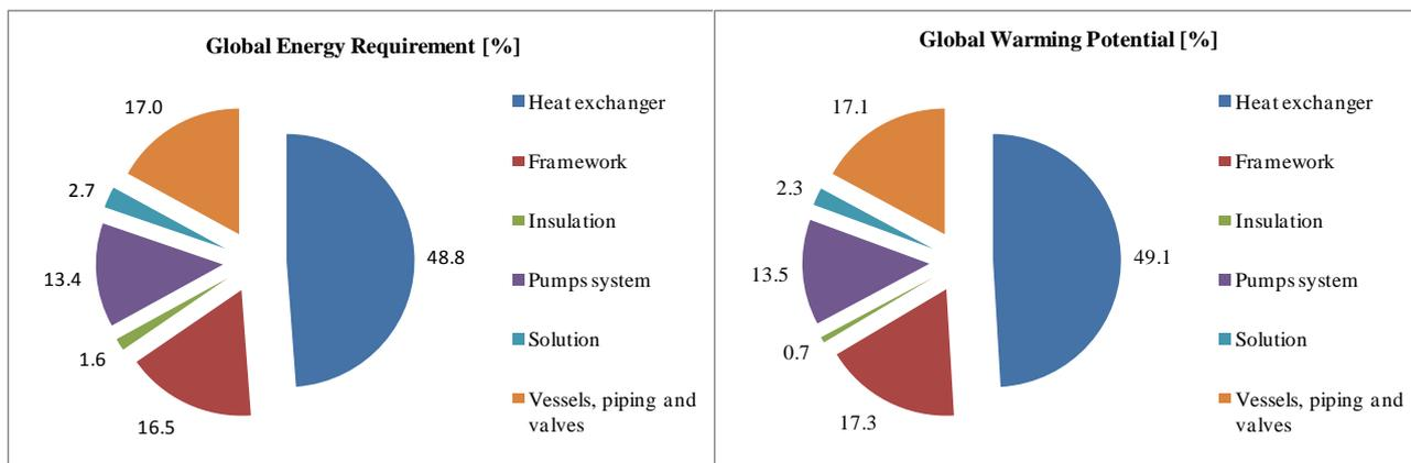
**Figure 10: Percentage contribution of different chiller components to GER and GWP**
