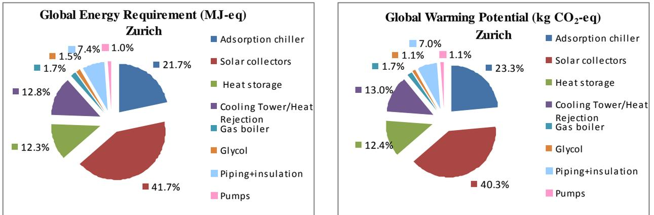
**Figure 32: Production phase: Percentage contribution of different plant components to GER and GWP for Zurich**
