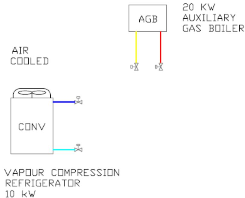
**Figure 1: Schematic representation of the conventional system**
