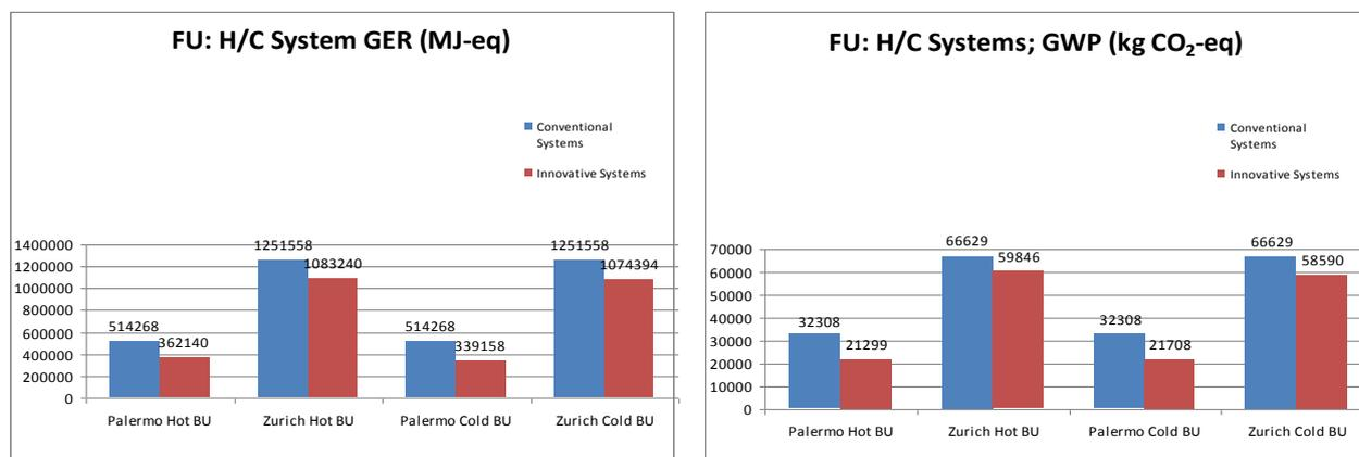
Figure 39: Comparison for the whole system during 25 years of energy use in both climates and both back-up for GER and GWP
