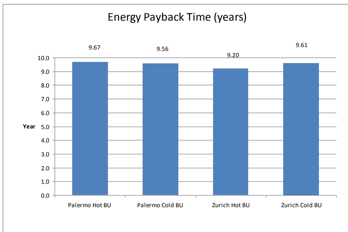
**Figure 42:  $E_{PT}$  for Adsorption Solar Cooling systems with hot and cold back-up**
