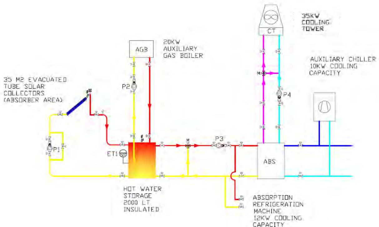
**Figure 5: Schematic representation of the absorption chiller plant (cold backup configuration)**
