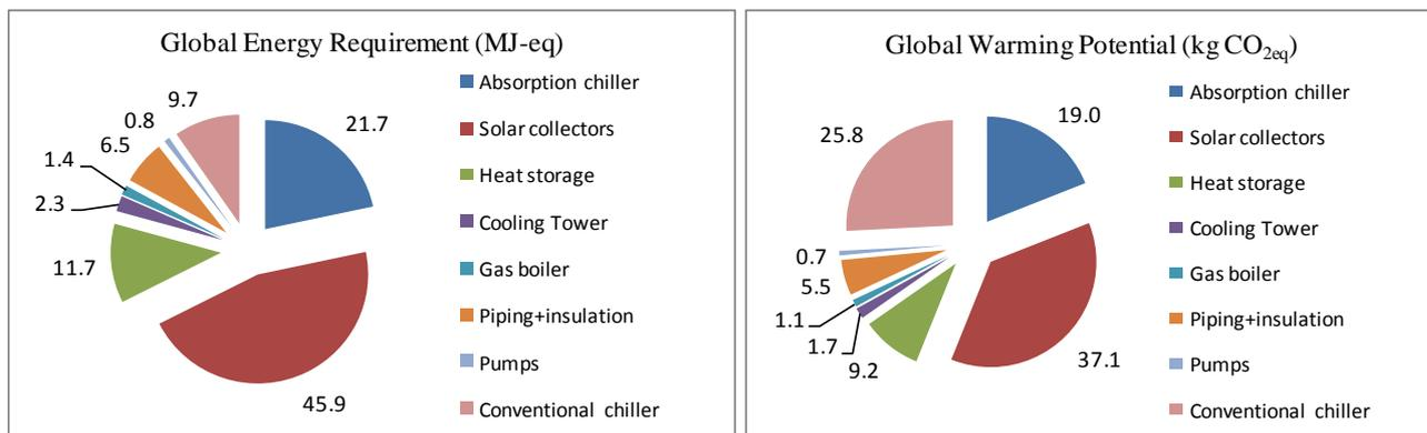
**Figure 17: Production phase. Percentage contribution of different plant components to GER and GWP for Palermo**
