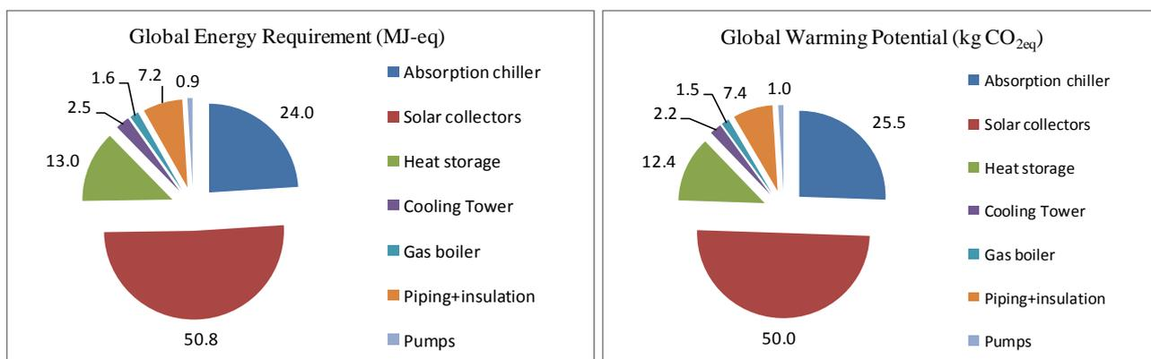
Figure 13: Production phase. Percentage contribution of different plant components to GER and GWP for Palermo
