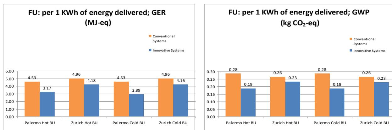
**Figure 41: Comparison per 1 kWh of energy produced during 25 years of energy use in both climates and both back-up for GER and GWP**
