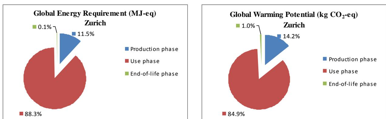
Figure 38: Percentage contribution of the three different phases for the whole life-cycle to GER and GWP for Zurich
