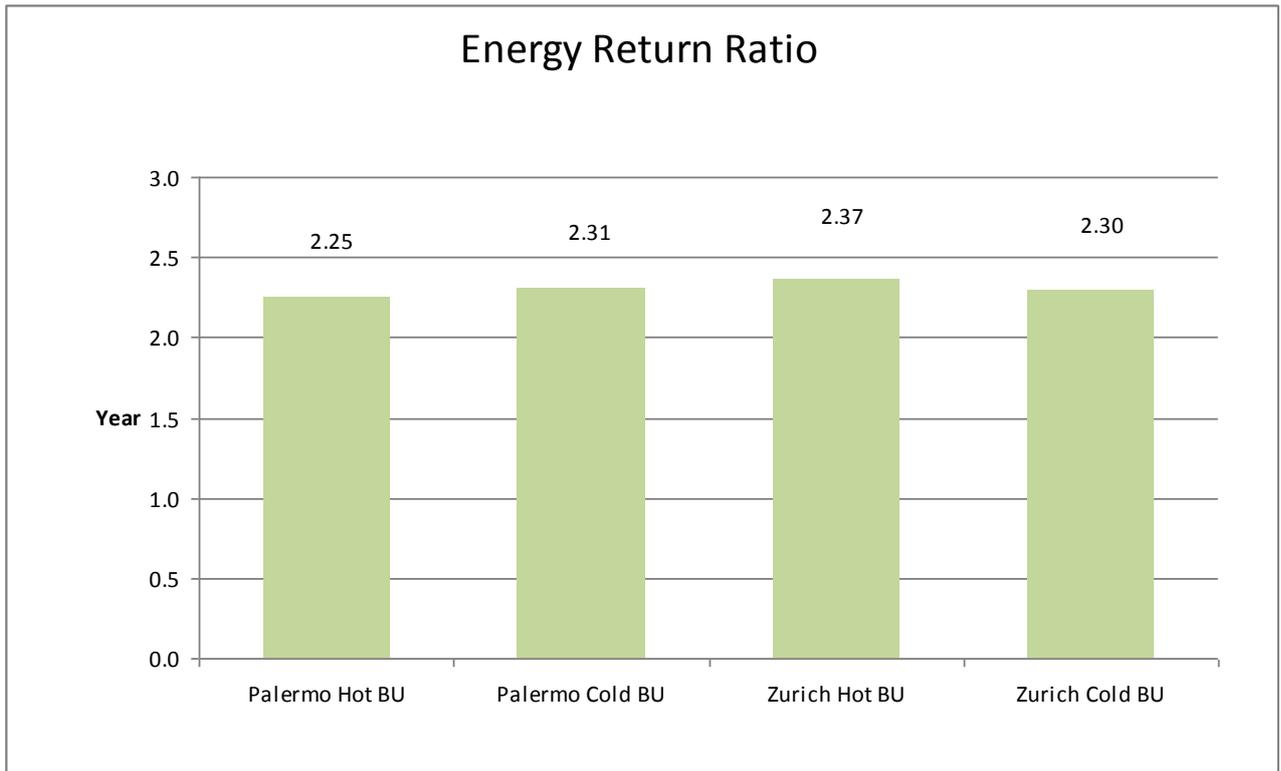
**Figure 44: E<sub>RR</sub> for Adsorption Solar Cooling systems with hot and cold back-up**
