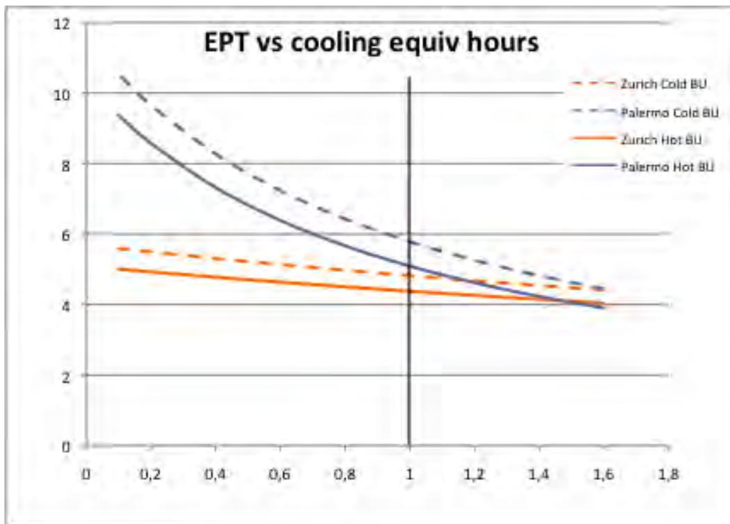
Figure 23: Relationship between  $E_{PT}$  and the number of equivalent hour of cooling operation for Absorption Solar Cooling systems with hot and cold back-up
