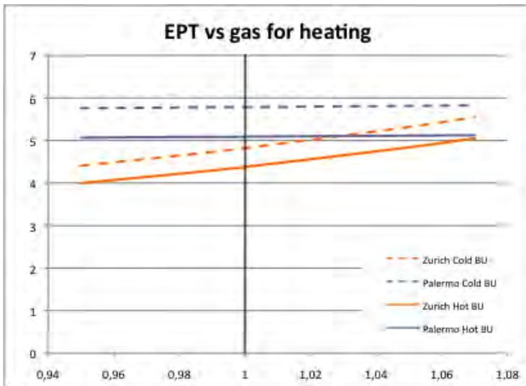
**Figure 25: Relationship between  $E_{PT}$  and gas consumption for Absorption Solar Cooling systems with hot and cold back-up**
