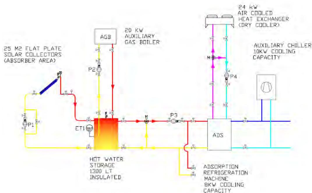
**Figure 28: Schematic representation of the adsorption chiller plant**
