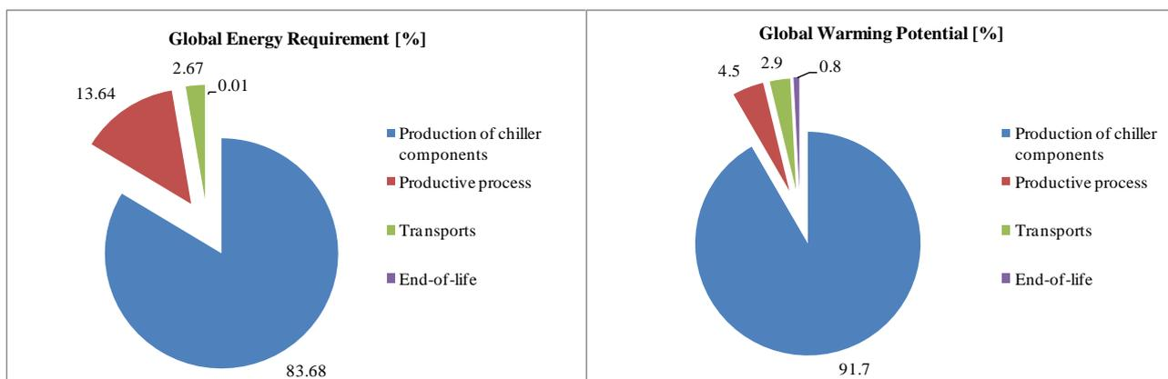
Figure 9: Percentage contribution of different phases of the chiller life-cycle to GER and GWP
