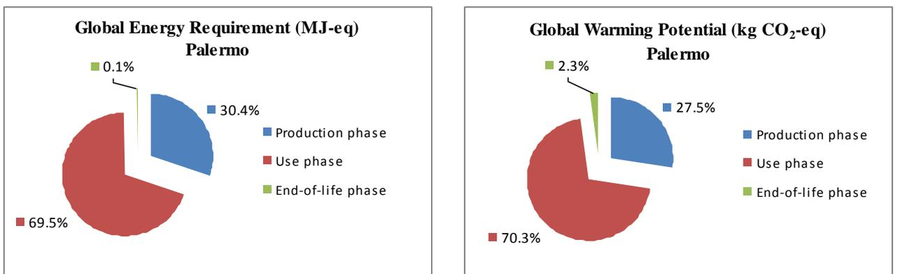
**Figure 33: Relative contribution of the three different phases for the whole life-cycle to GER and GWP for Palermo**
