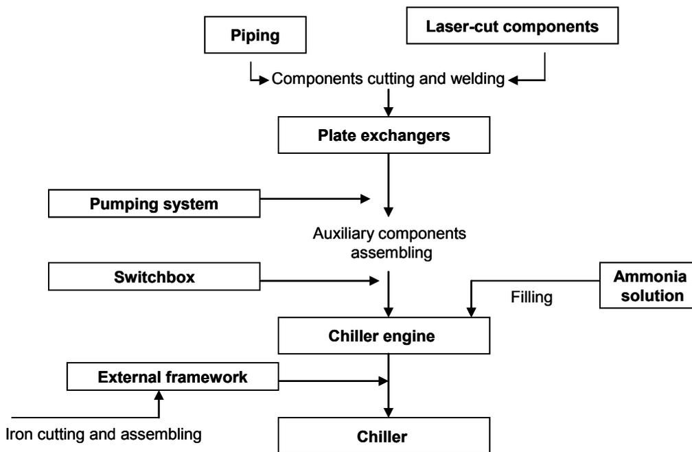
Figure 8: Production diagram flow
