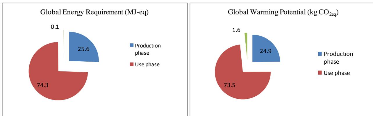
Figure 11: Percentage contribution of different phases of the plant life-cycle to GER and GWP for Palermo
