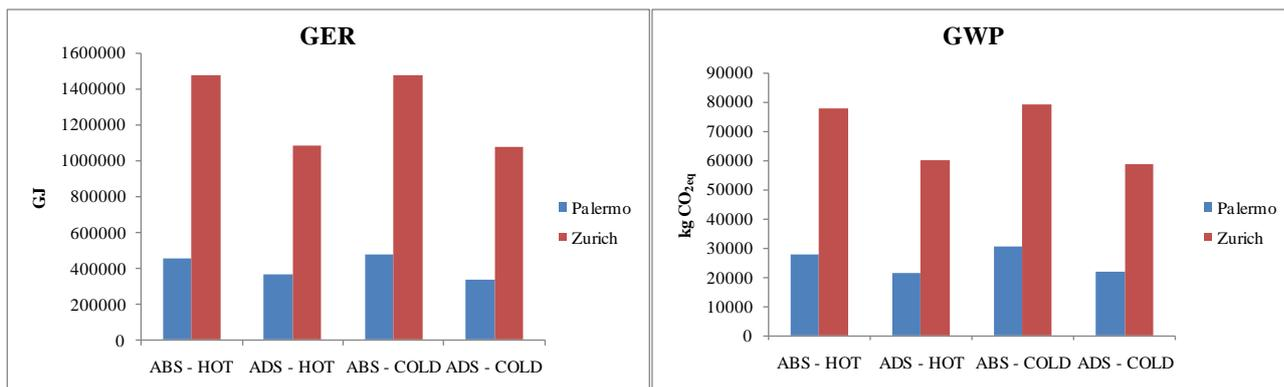
Figure 54: Comparison of GER (MJ) and GWP for ABS and ADS plants
