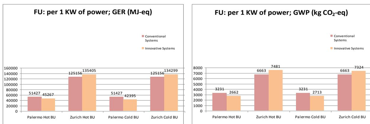
Figure 40: Comparison per 1kW of cooling power during 25 years of energy use in both climates and both back-up for GER and GWP
