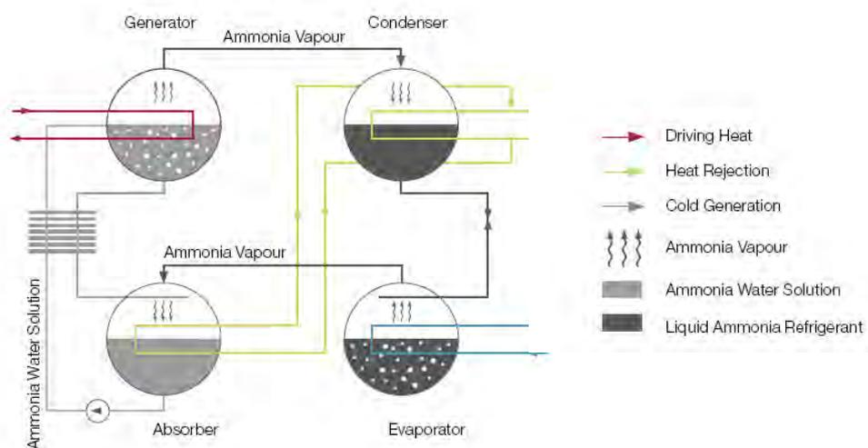
**Figure 6: Ammonia cycle into Absorption Chiller [Solarnext, 2009]**
