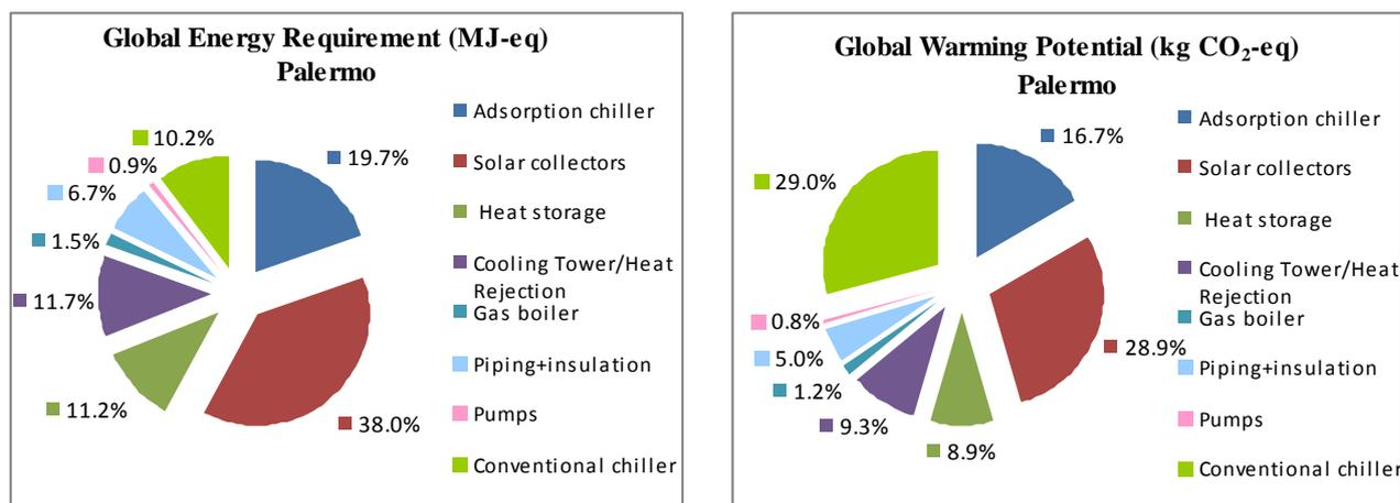
**Figure 35: Production phase: Percentage contribution of different plant components to GER and GWP for Palermo**
