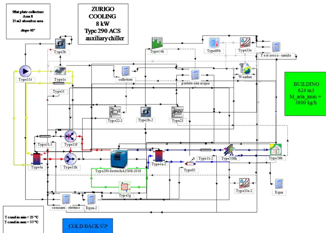
**Figure 3: TRNSYS project for simulation of the adsorption chiller plant with cold back up**
