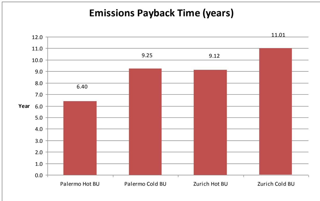
**Figure 43: Emissions Payback Time for Adsorption Solar Cooling systems with hot and cold back-up**
