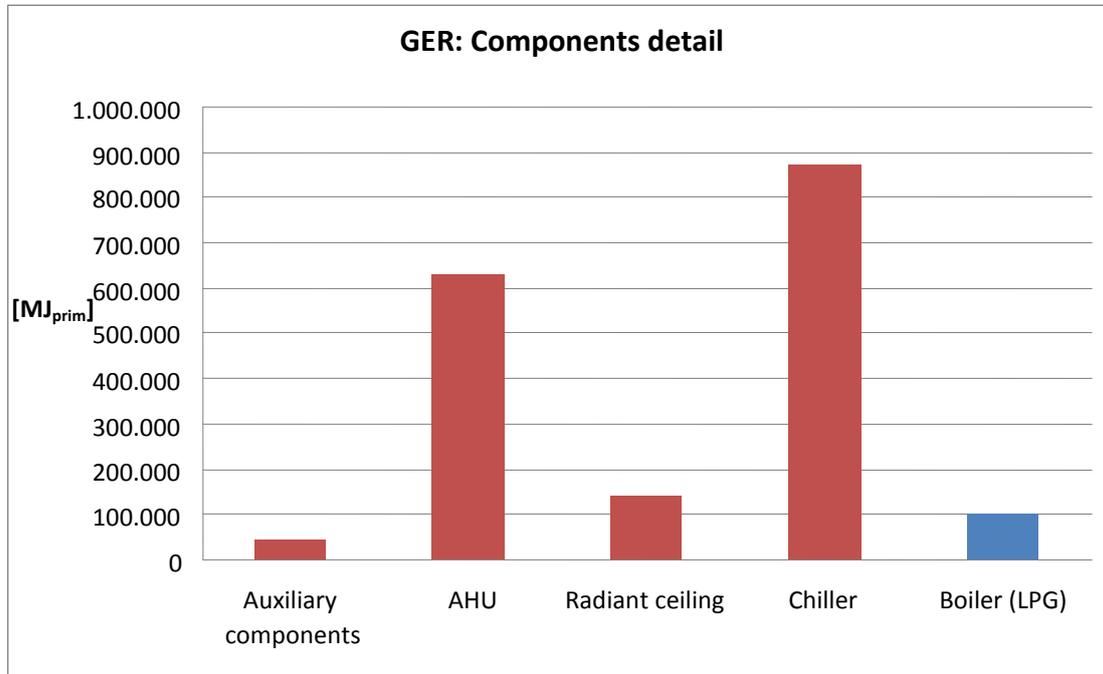
Figure 49: Comparison of impacts related to system components (GER)
