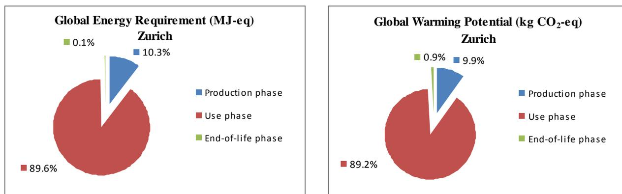
**Figure 34: Relative contribution of the three different phases for the whole life-cycle to GER and GWP for Zurich**
