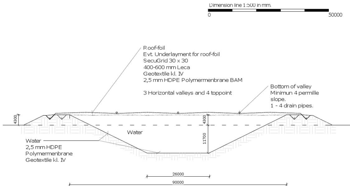
Figure 13: Cross section of the PIT storage construction in Marstal, Dk (75,000 m<sup>3</sup>) (source: Planenergi)
