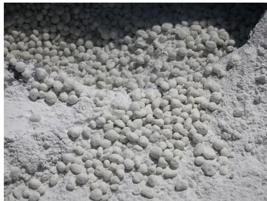
Detailed view of the expanded glass granules. Due to the blowing in process a small part of the granules are pulverized to dust.
