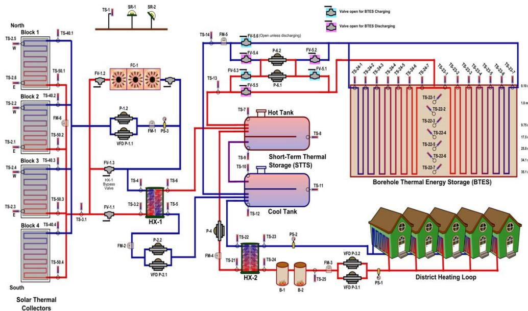
Figure 19: Overall system with the integrated BTES in Drake Landing Solar Community (source: Natural Resources Canada)
