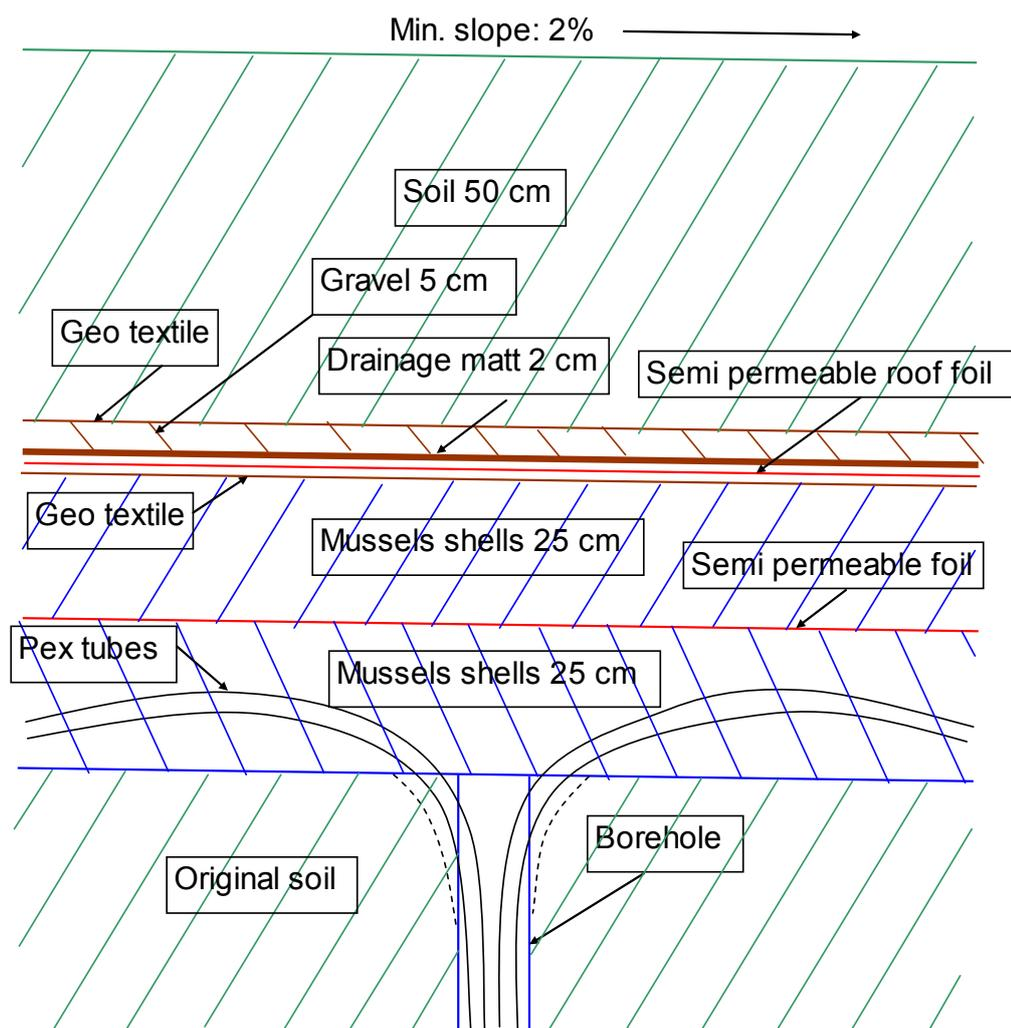
Figure 18: Cross section through the top horizontal layer of the BTES in Bradstrup (source: Planenergi)
