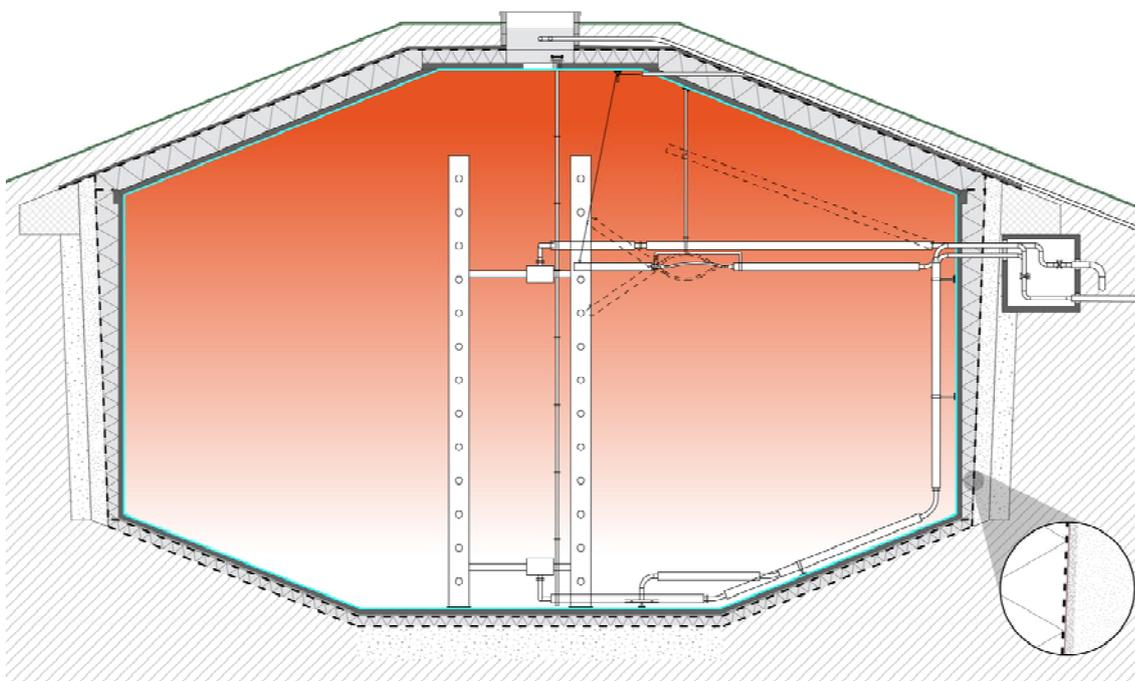
Figure 12: Vertical section of the Munich STES (source: Solites)
