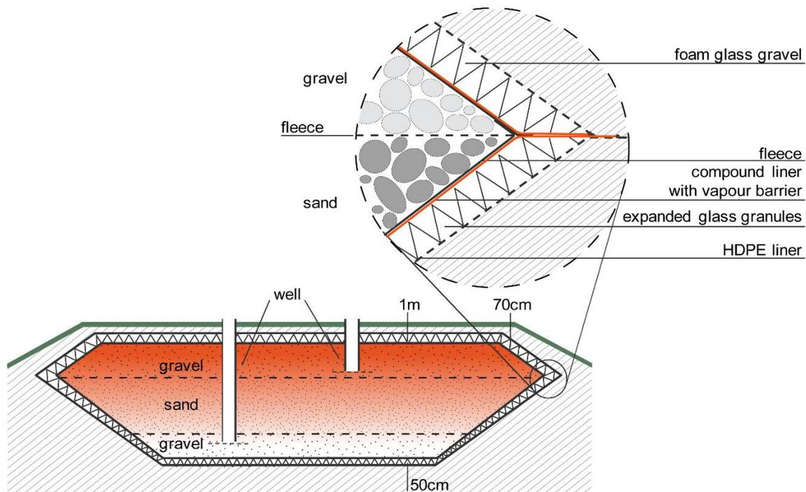
Figure 14: Cross section of the PIT storage construction in Eggenstein-Leopoldshafen, Germany (4,500 m<sup>3</sup>) (source: Solites)
