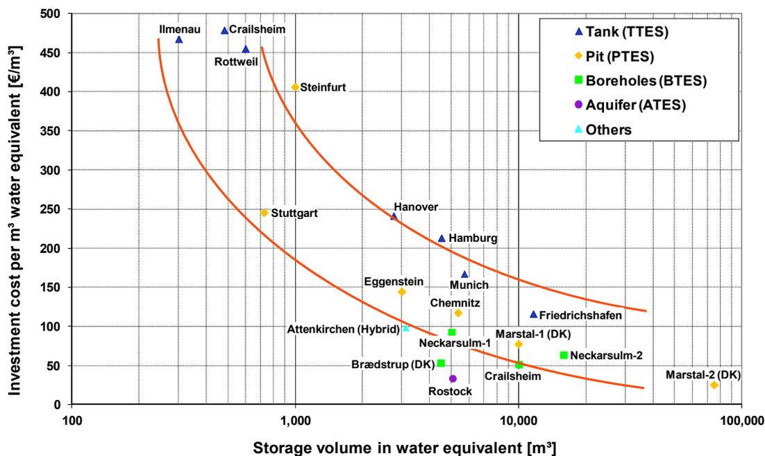
Figure 10: Specific storage costs of demonstration plants (cost figures without VAT) (source: Solites)
