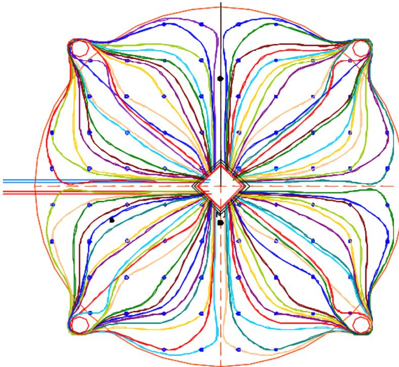
Figure 15: Top view with horizontal piping of BTES in Crailsheim, 2008 (source: Utilities of Crailsheim)
