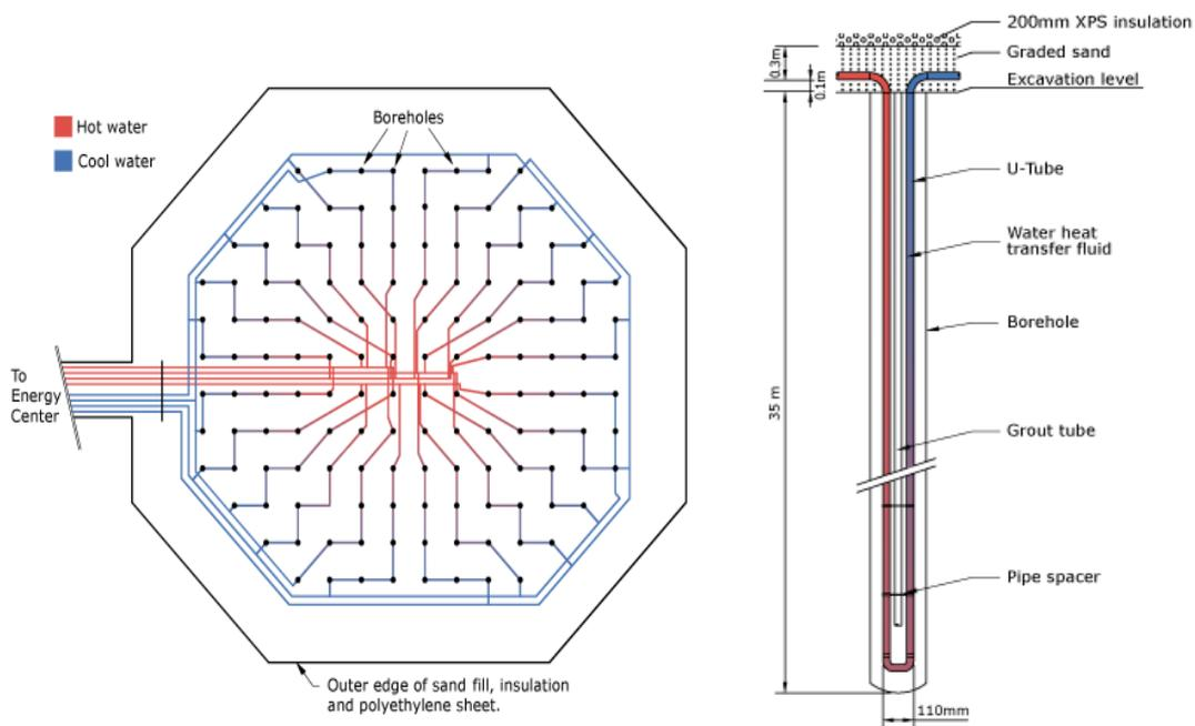
Figure 20: Storage schematic of the BTES in Drake Landing Solar Community (source: Natural Resources Canada)
