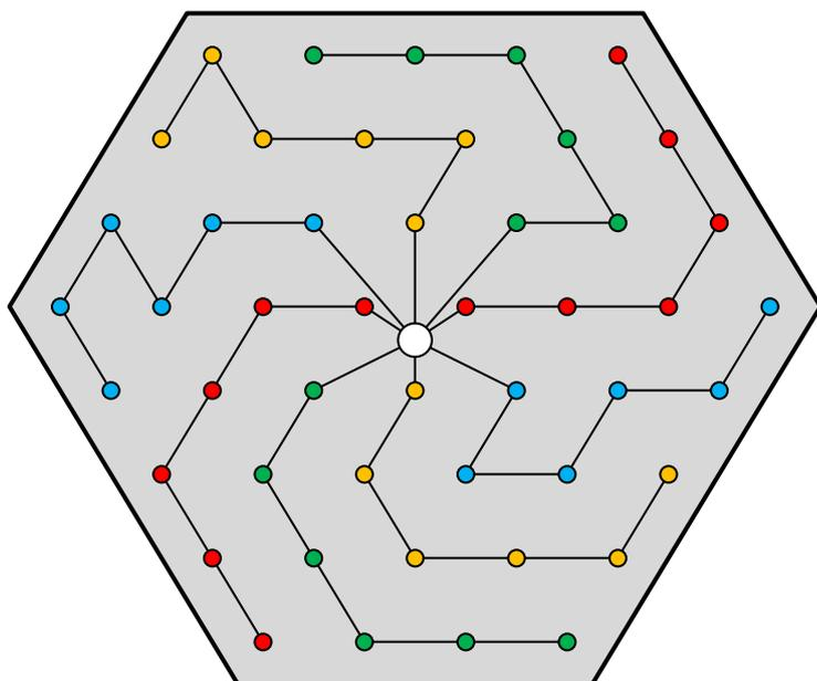
Figure 17: Pipe layout for the BTES in Braedstrup. Only connections to one of the U-pipes in each borehole are shown. The pipe layout for the second U-pipes will be mirrored through a vertical line to minimize the number of boreholes shared by two flow strings. All "dead ends" will be connected to the shaft in the center (source: Planenergi)
