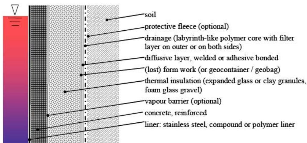
Figure 6: Multilayered (composite) side wall of a seasonal thermal energy storage, exterior insulation with respect to the concrete/steel structure (source: Solites)
