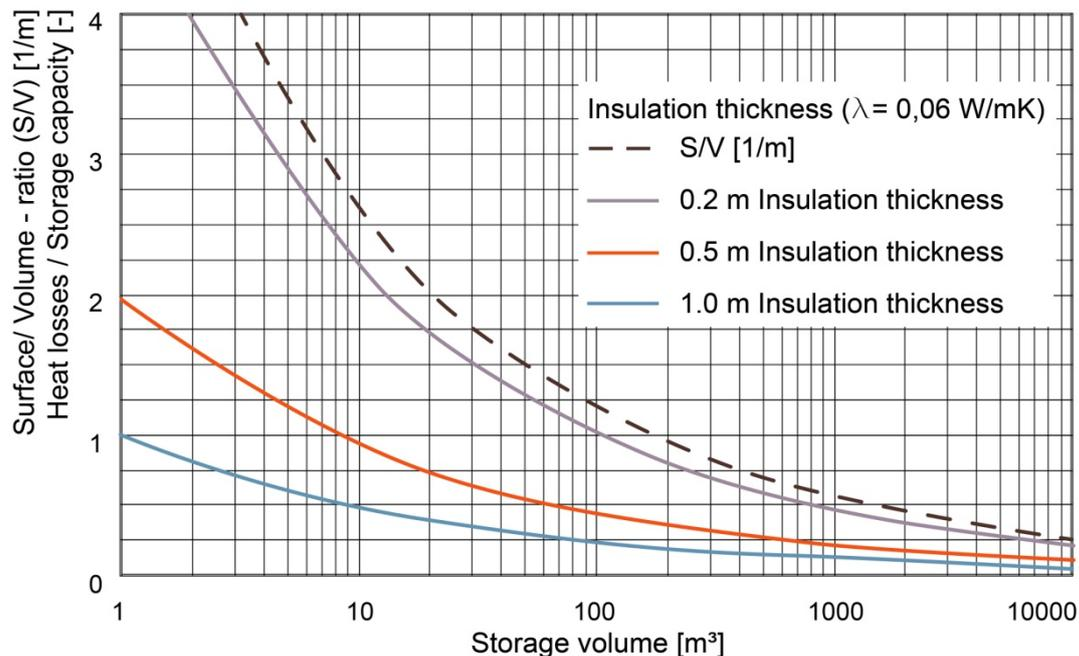
Figure 3: Heat losses/storage capacity ratio based on storage volume in  $m^3$  (source: Solites)
