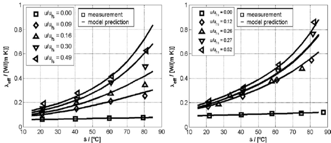
Figure 11: Model predictions and measured data for the thermal conductivity ( $\lambda_{eff}$ ) of expanded glass granules 4-8 mm type II (EGG:left) and expanded clay 4-8 type I (EC: right) as function of the temperature ( $\theta$ ) with normalised water content ( $u/u_{ts}$ ) as parameter. (source: F. Ochs, University of Innsbruck, Austria)
