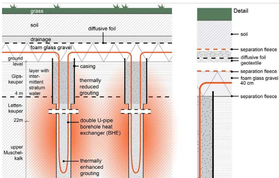
Figure 16: Cross section through the BTES in Crailsheim (source: Solites)
