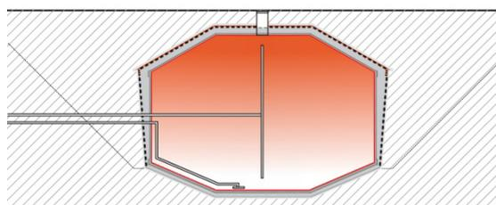
Figure 5: Tank thermal energy storage concept (source: Solites)
