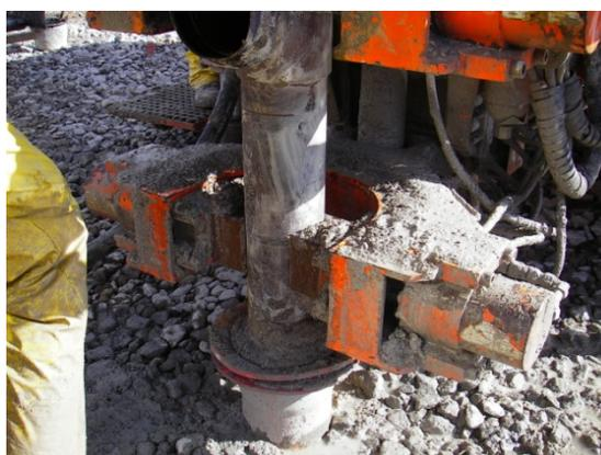
*The drilling head inside the borehole*
