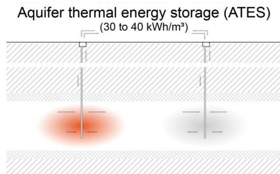
Figure 9: Aquifer thermal energy storage concept (source: Solites)
