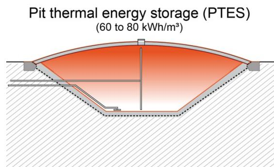
Figure 7: Pit thermal energy storage concept (source: Solites)
