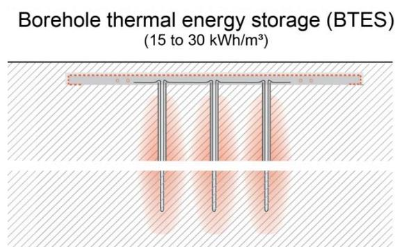
*Figure 8: Borehole thermal energy storage concept
