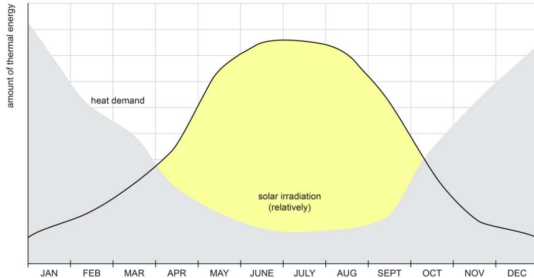
Figure 1: Solar radiation and heat demand repartition over a year (source: Solites)
