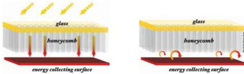
Figure 4: The Principle of Using Transparent Insulation (Source: TIGI Limited)
