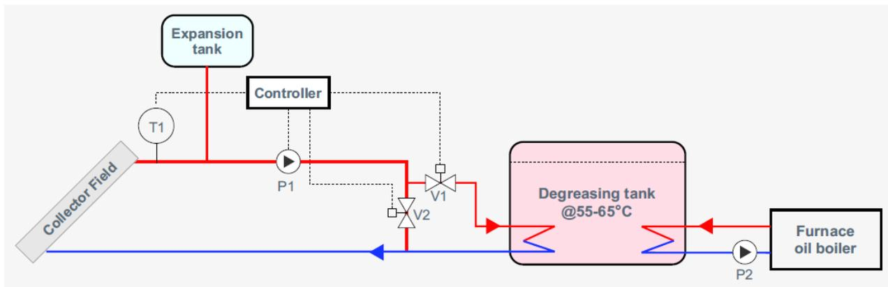
**Figure 11: Hydraulic scheme of solar water heating system at Wheels India Ltd. (Source: Aspiration Energy)**
