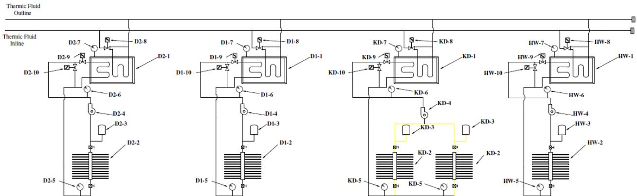
**Figure 10: Four separate solar thermal systems installed for each heat demanding process. (from left to right) System 4, System 3, System 2, System 1. (Source: Aspiration Energy)**
