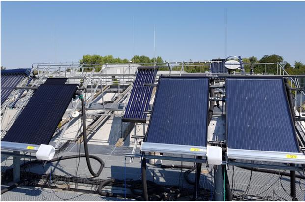
Fig. 4. Outdoor test facilities with the investigated PVT collectors.
