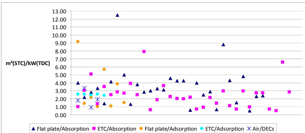
Figure 4.5 Rates between the solar surface collectors installed per kW of cooling capacity for the most used technologies combinations
