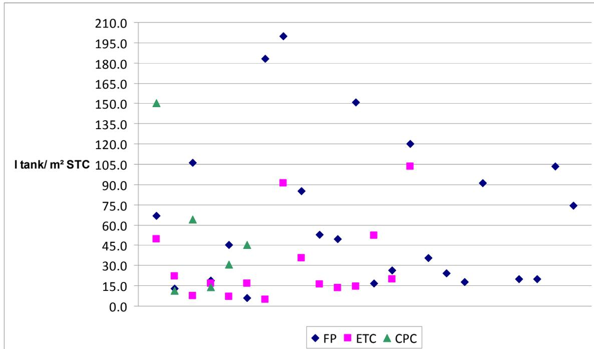
Figure 4.7 Rate between the litres of hot water storage tanks used in each of 46 installations and classified according to the technology used for solar thermal collectors
