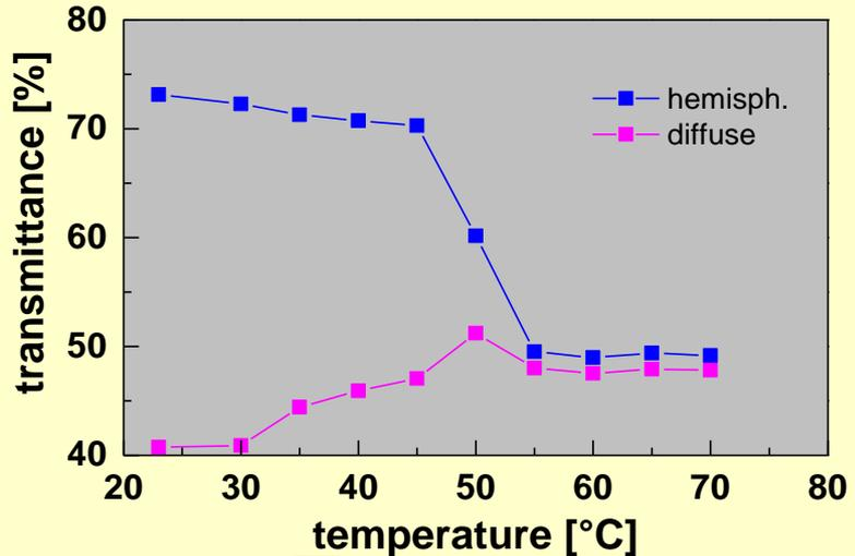
Absorber materials for overheating protected collectors
