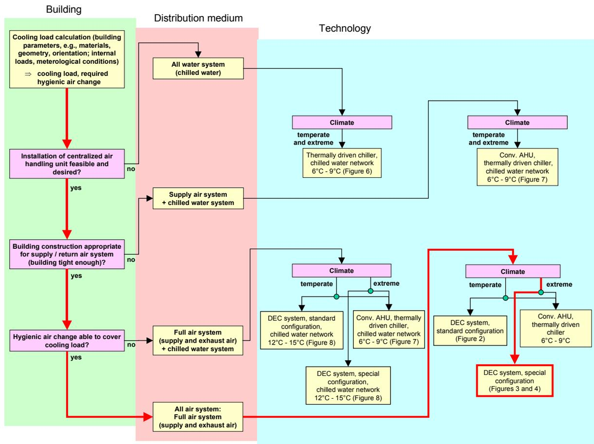
Figure 15 - Path leading to a desiccant air handling unit in an all, full air system (extreme climate)
