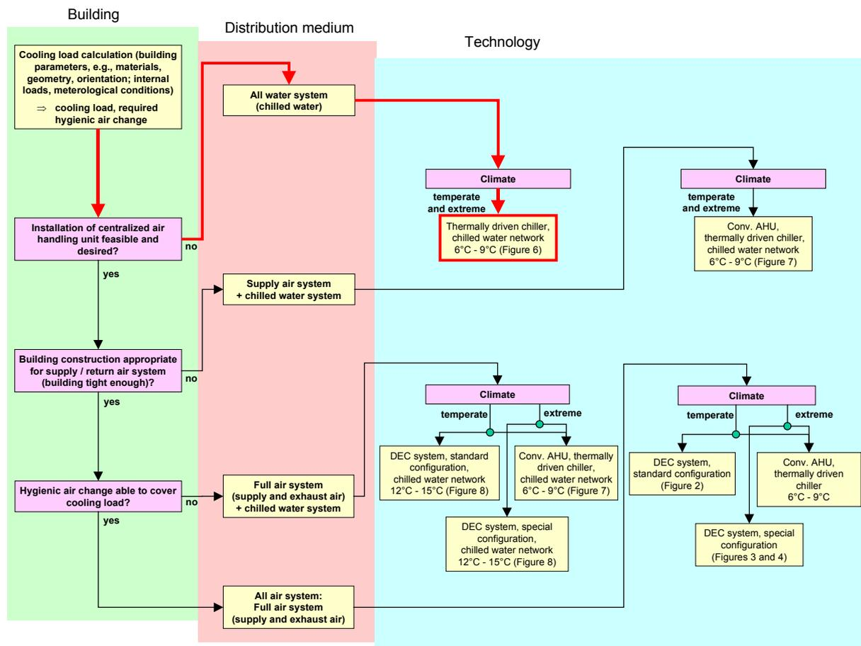
**Figure 3** – Path leading to an all water system using a thermally driven chiller
