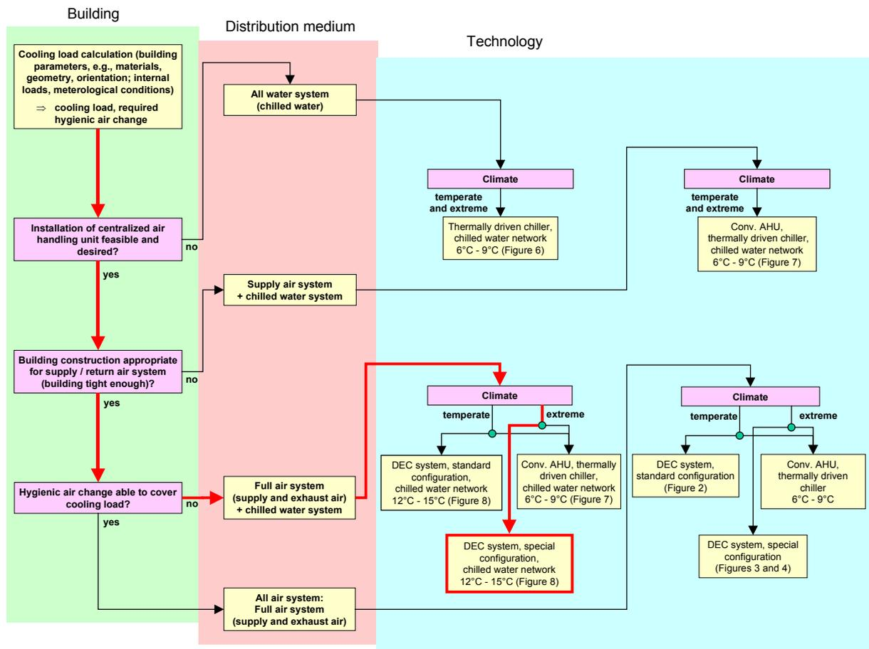
Figure 9 - Path leading to a desiccant system and a an additional chilled water system (humid climates)
