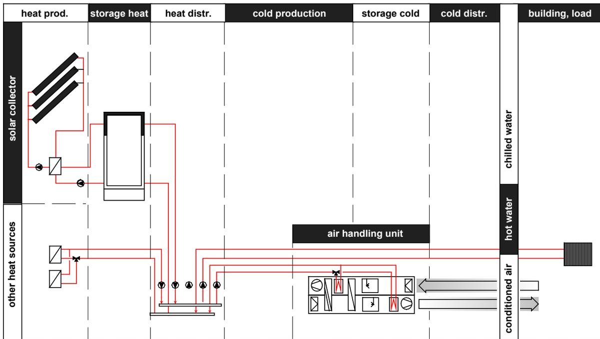
Figure 14 - Example of a technical solution for the path shown in Figure 13
