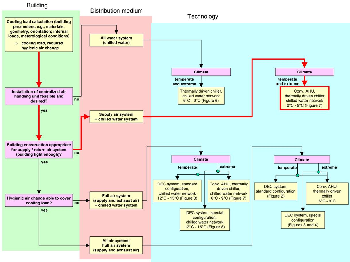
**Figure 5** – Path leading to a thermally driven chiller which provides chilled water to a supply air system and a chilled water system
