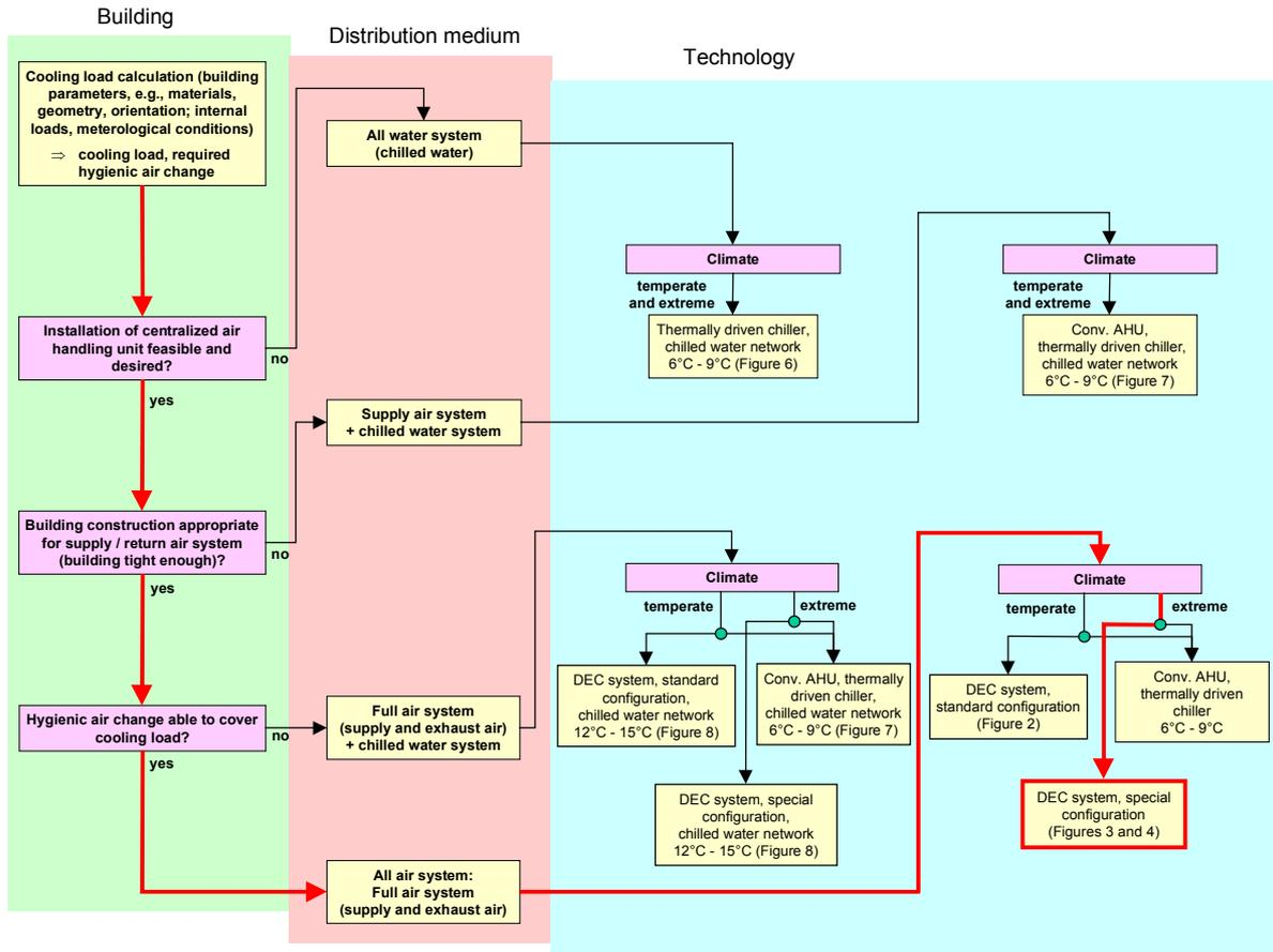
Figure 17 - Path leading to an all, full air system using a conventional air handling unit and a thermally driven chiller
