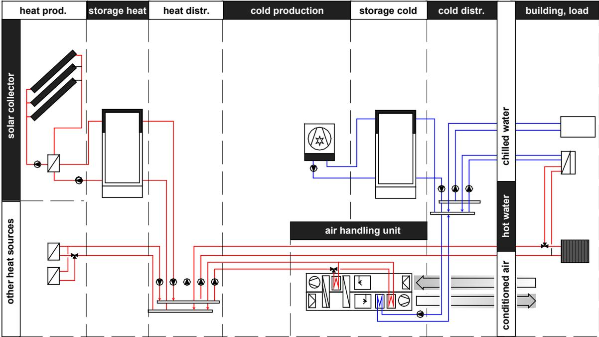
Figure 10 – Example of a technical solution for the path shown in Figure 9
