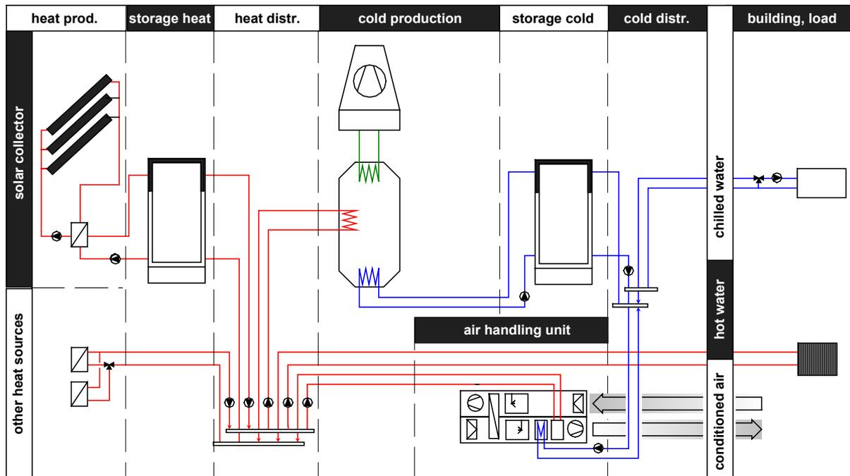
**Figure 12** - Example of a technical solution for the path shown in Figure 11
