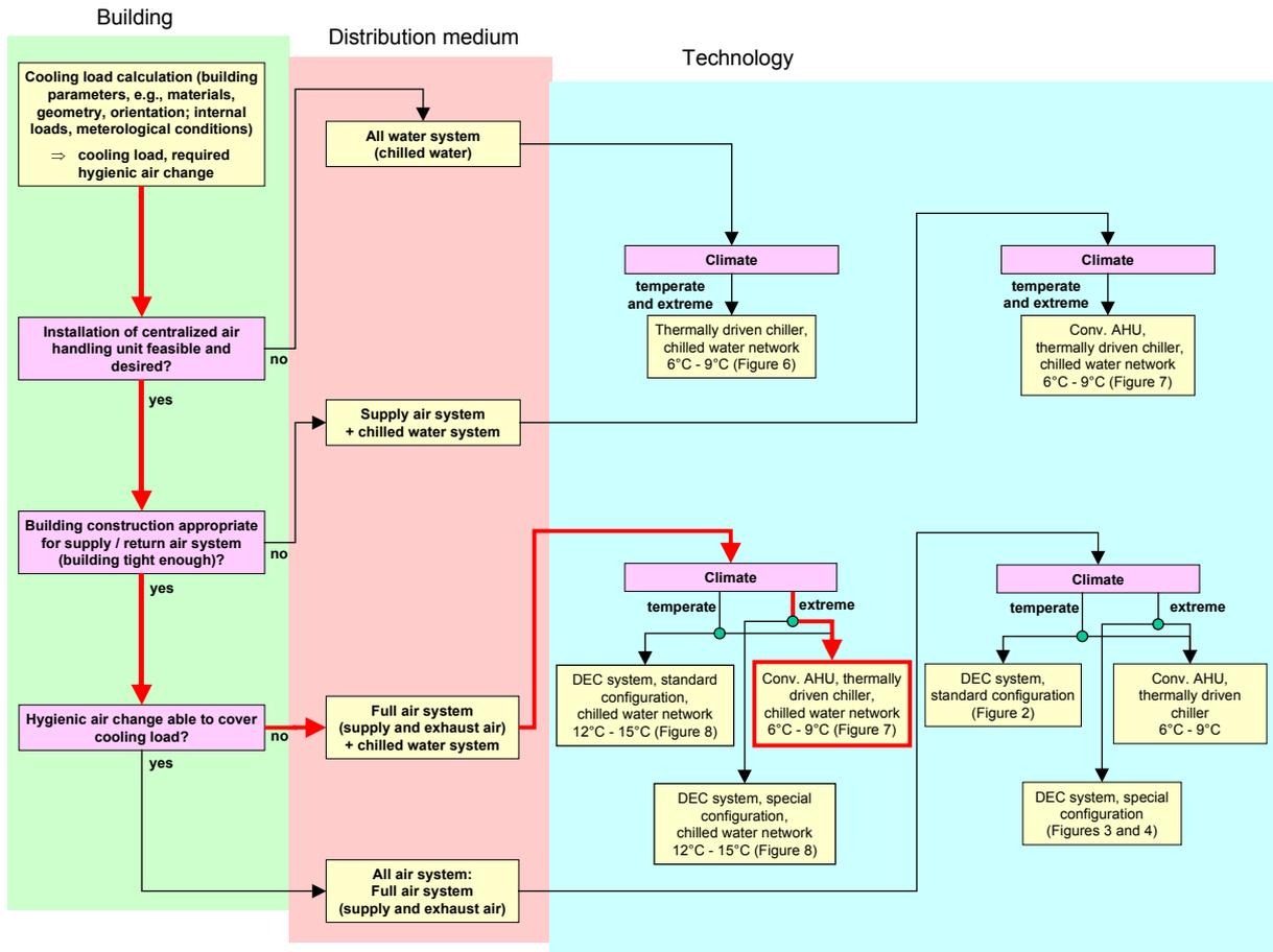
**Figure 11** - Paths leading to a conventional supply/return air system and an additional chilled water system
