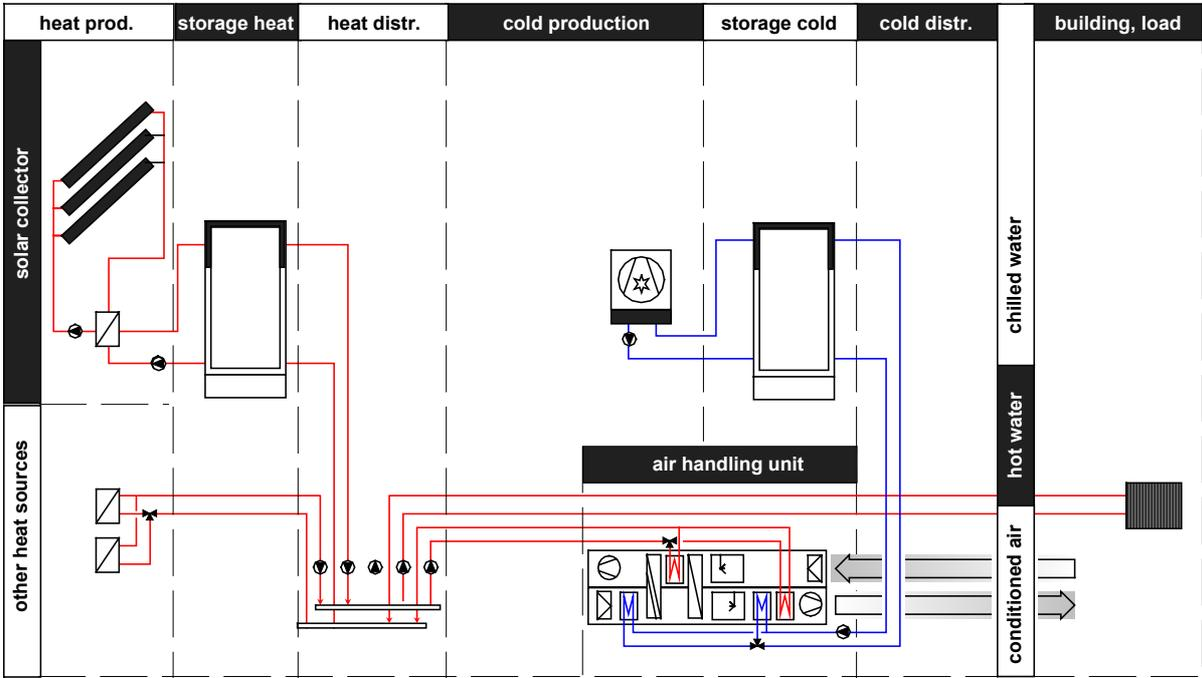
Figure 16 - Example of a technical solution for the path shown in Figure 15
