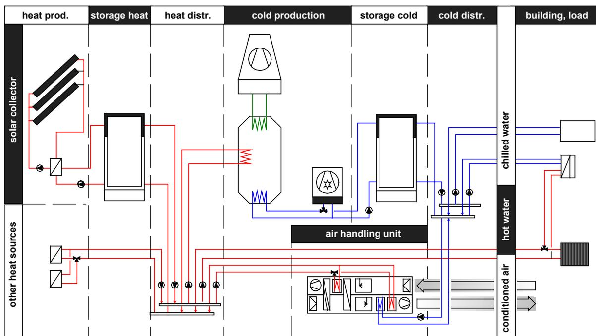
**Figure 2** – Scheme of a complete system including desiccant technique and thermally driven water chiller
