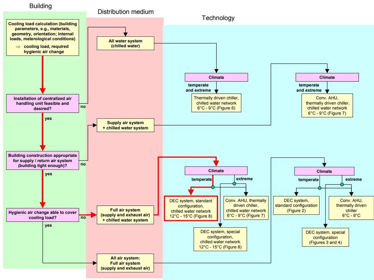
**Figure 7** – Path leading to a desiccant system and a an additional chilled water system
