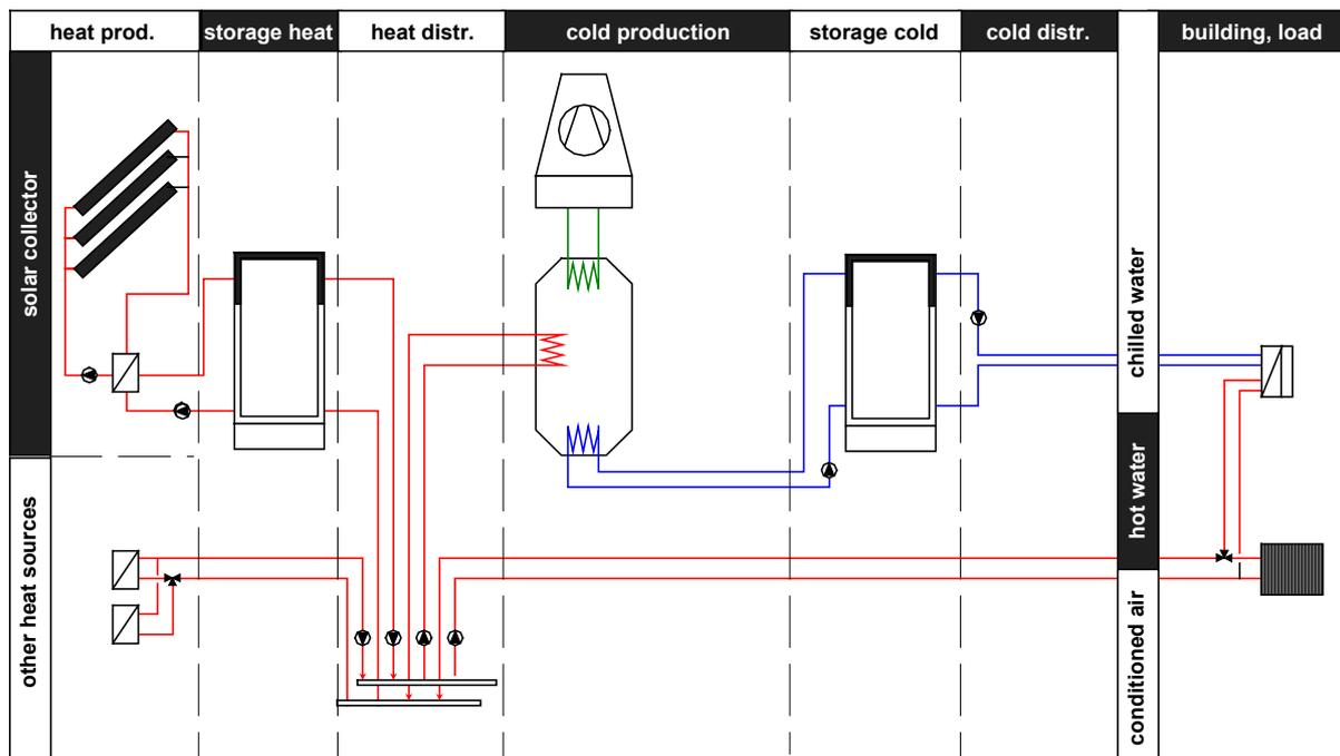
**Figure 4** – Example of a technical solution for the path shown in Figure 3
