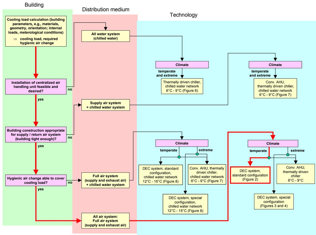
**Figure 13** - Path leading to a desiccant air handling unit in an all air, full air system (moderate climate)
