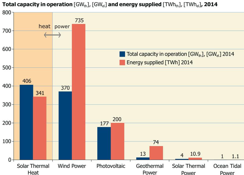
**Figure 3:** Global capacity in operation [GW<sub>el</sub>], [GW<sub>th</sub>] 2014 and annual energy yields [TWh<sub>el</sub>], [TWh<sub>th</sub>] (Sources: AEE INTEC, Global Wind Energy Council (GWEC), European PV Industry Association (EPIA), REN21 - Global Status Reports 2014 and 2015)
