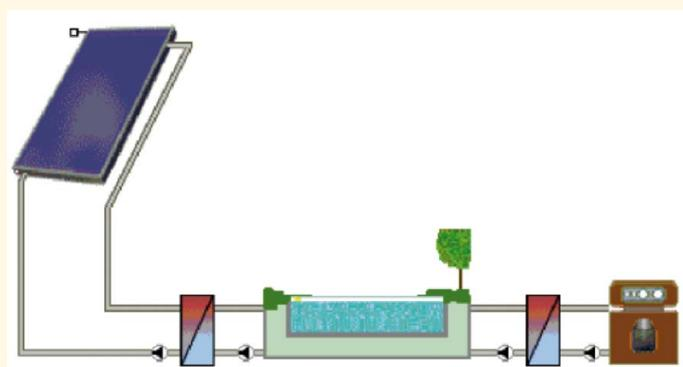
Figure 52: Hydraulic scheme of the swimming pool reference system
