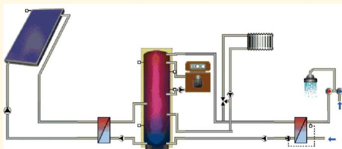
**Figure 56:** Hydraulic scheme of the solar-combi reference system for single and multi-family houses
