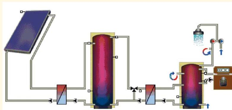
**Figure 55:** Hydraulic scheme of the domestic hot water pumped reference system for multifamily houses
