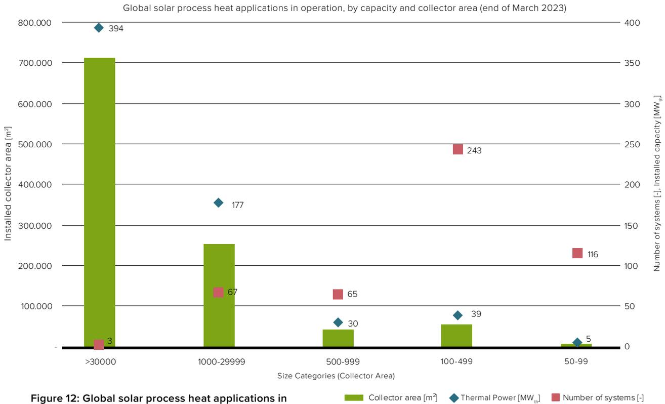
**Figure 12: Global solar process heat applications in operation the end of March 2023 by number, capacity and collector area** Source: IV SHIP database
