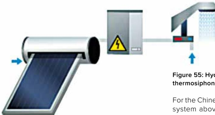
**Figure 55: Hydraulic scheme of the domestic hot water thermosiphon reference system for single-family houses**
