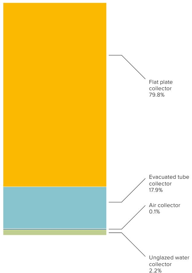
**Figure 22: Distribution of the total installed capacity in operation by collector type in 2021 – EUROPE**
