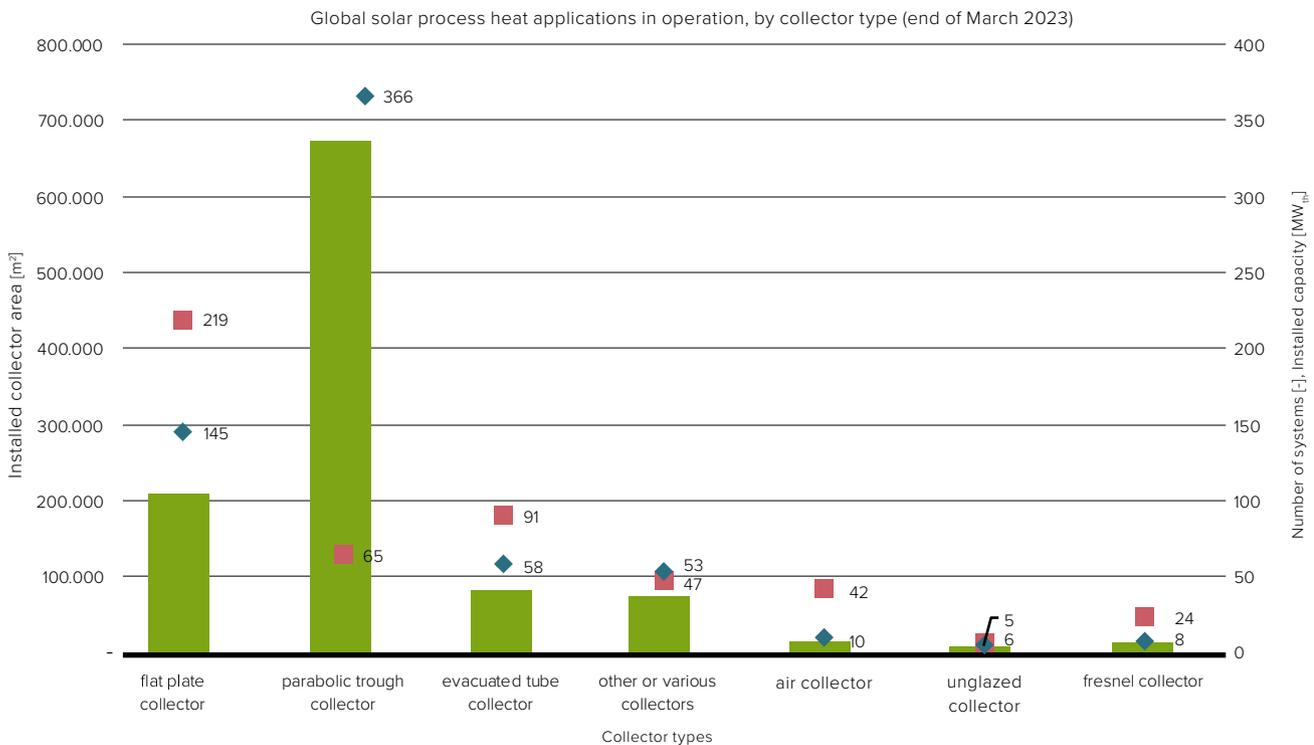
**Figure 13: Global solar process heat applications in operation at the end of March 2023 by collector type** Source: SHIP database
