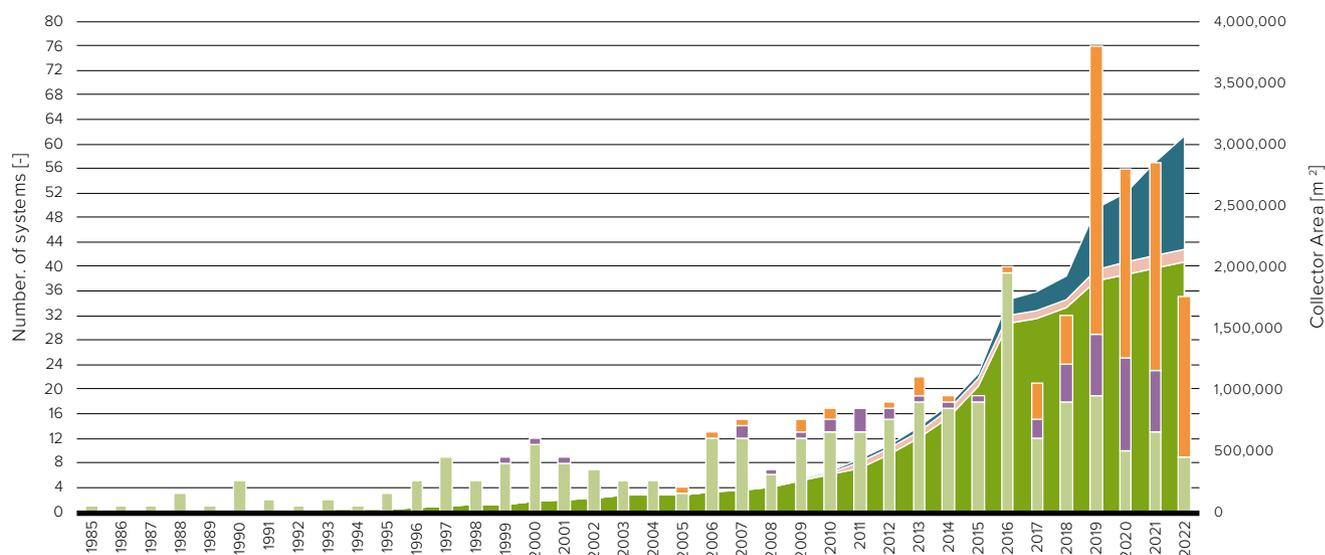
**Figure 8: Large-scale systems for solar district heating and large residential, commercial and public buildings worldwide – annual installations and cumulated area in operation in 2022**
