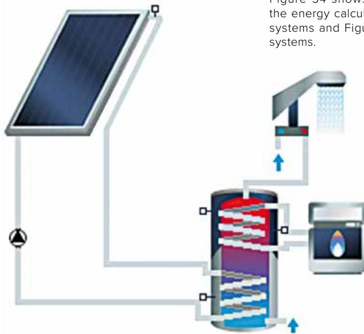
Figure 54 shows the hydraulic scheme used for the energy calculation for all pumped solar thermal systems and Figure 55 refers to the thermosiphon systems.
