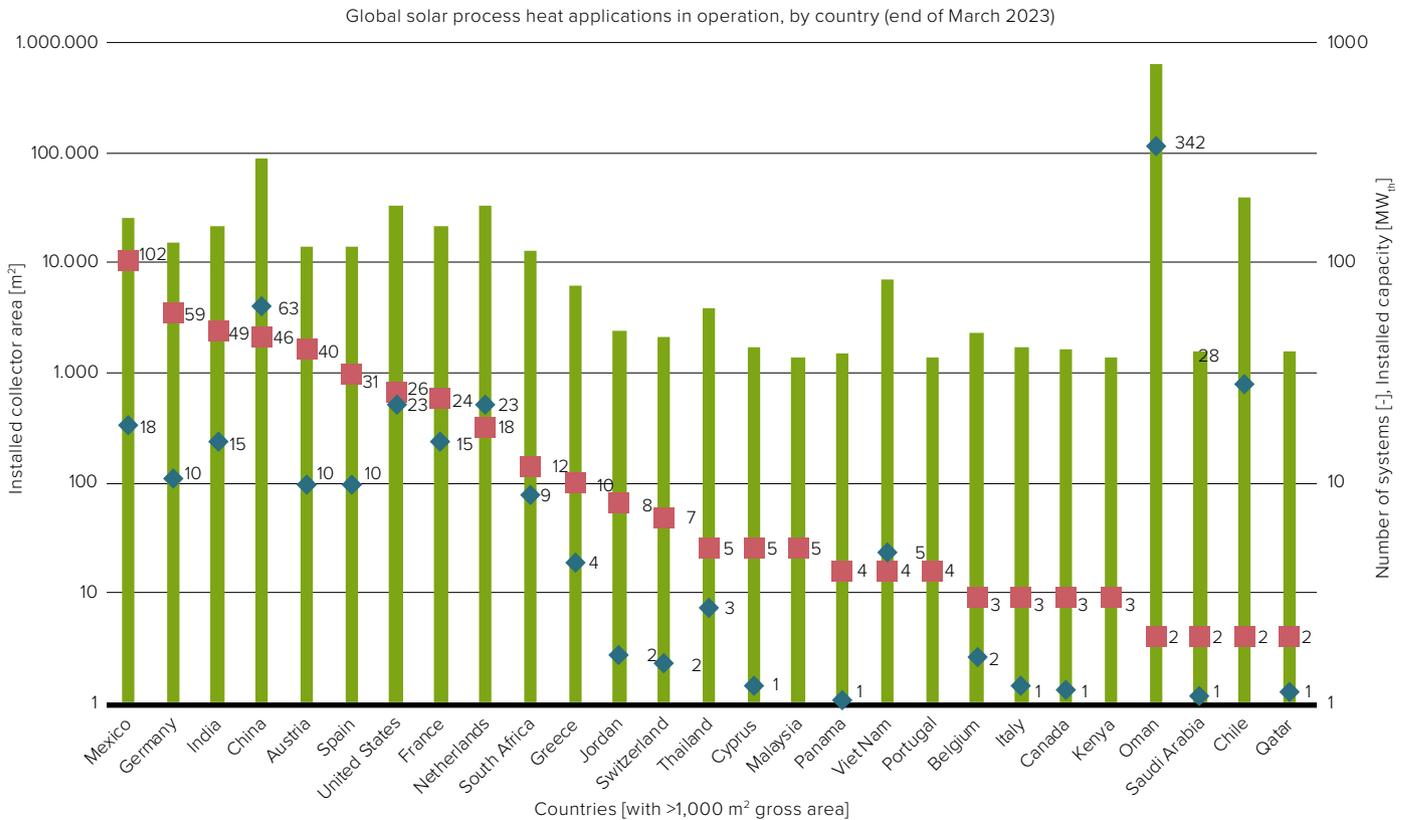
**Figure 15: Global solar process heat applications in operation by country at the end of March 2023**
