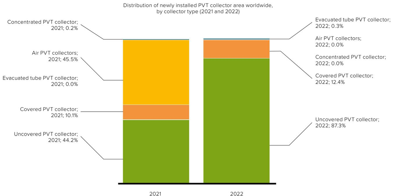
**Figure 18: Distribution of newly installed PVT collector area worldwide by collector type in 2021 (left) 2022 (right)**
