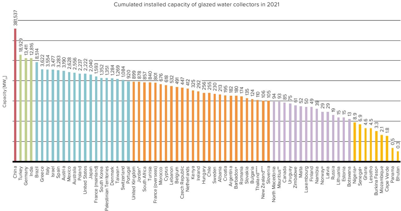
Figure 25: Total capacity of glazed water collectors in operation by the end of 2021
