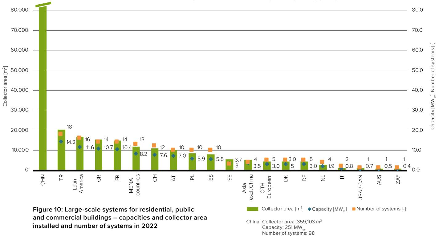
Figure 10: Large-scale systems for residential, public and commercial buildings – capacities and collector area installed and number of systems in 2022
