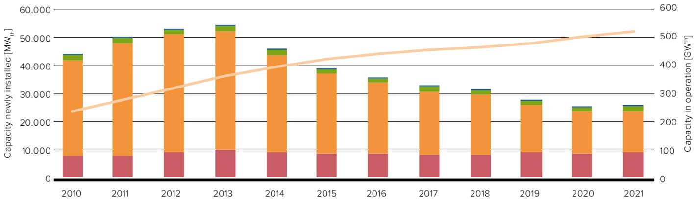
Figure 4: Annual installed capacity by collector type and total installed capacity 2010-2021
