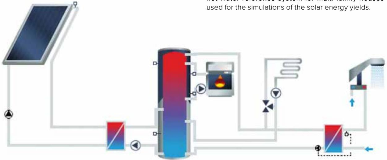
Figure 57 shows the hydraulic scheme of the domestic hot water reference system for multi-family houses used for the simulations of the solar energy yields.
