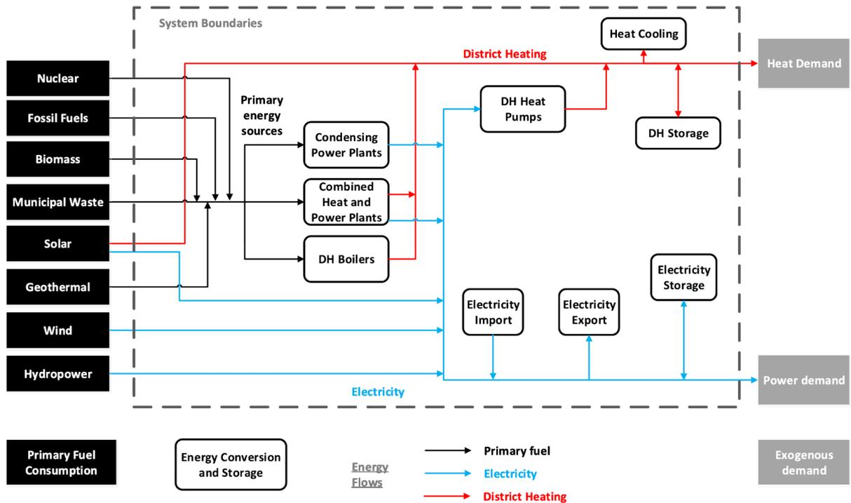
Figure 1: Core structure of Balmorel model [3]
