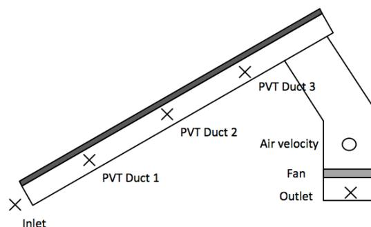
Figure 21 Schematic of thermocouple and air velocity sensor location
