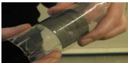
**Figure 13** A small module showing the flexibility of all components.
