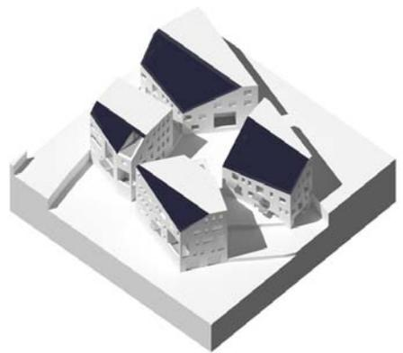
Figure 2: VectorWorks, sun and shade study. Outputs such as this can aid the architect in design decision making and improve his/her communication with the engineer and/or solar consultant(s).
