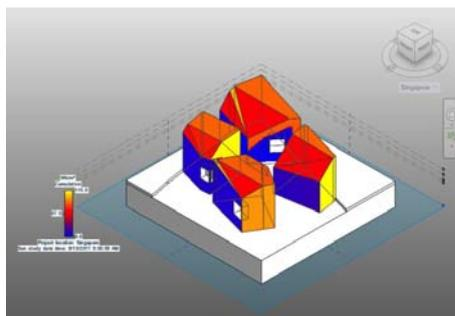
Figure 3: Project Vasari can present various solar radiation options: cumulative, average mean of hourly values, and peak maximum value in [kWh/m<sup>2</sup>/year]. Output such as this can help improve communication with engineer and solar consultant and can lead to joint decision making regarding solar strategies. In order to assist communication between architect and client such results could be transferred into potential energy savings or potential financial savings.
