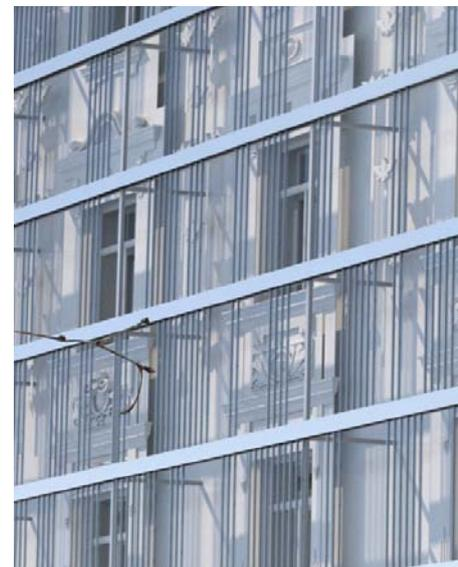
Figure 5: Visualization of proposal for evacuated tube collectors in front of listed building façade in Graz, Austria. Source: Institute of Architectural Typologies, Graz Technical University
