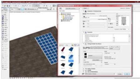
A number of PV plug-in modules for CGI tools are currently in development. The Solar Energy Research Institute of Singapore (SERIS) recently developed PV modules of 7 manufacturers for Revit (currently being tested). Similar modules are also being developed at the University of Applied Sciences and Arts of Southern Switzerland (SUPSI).
