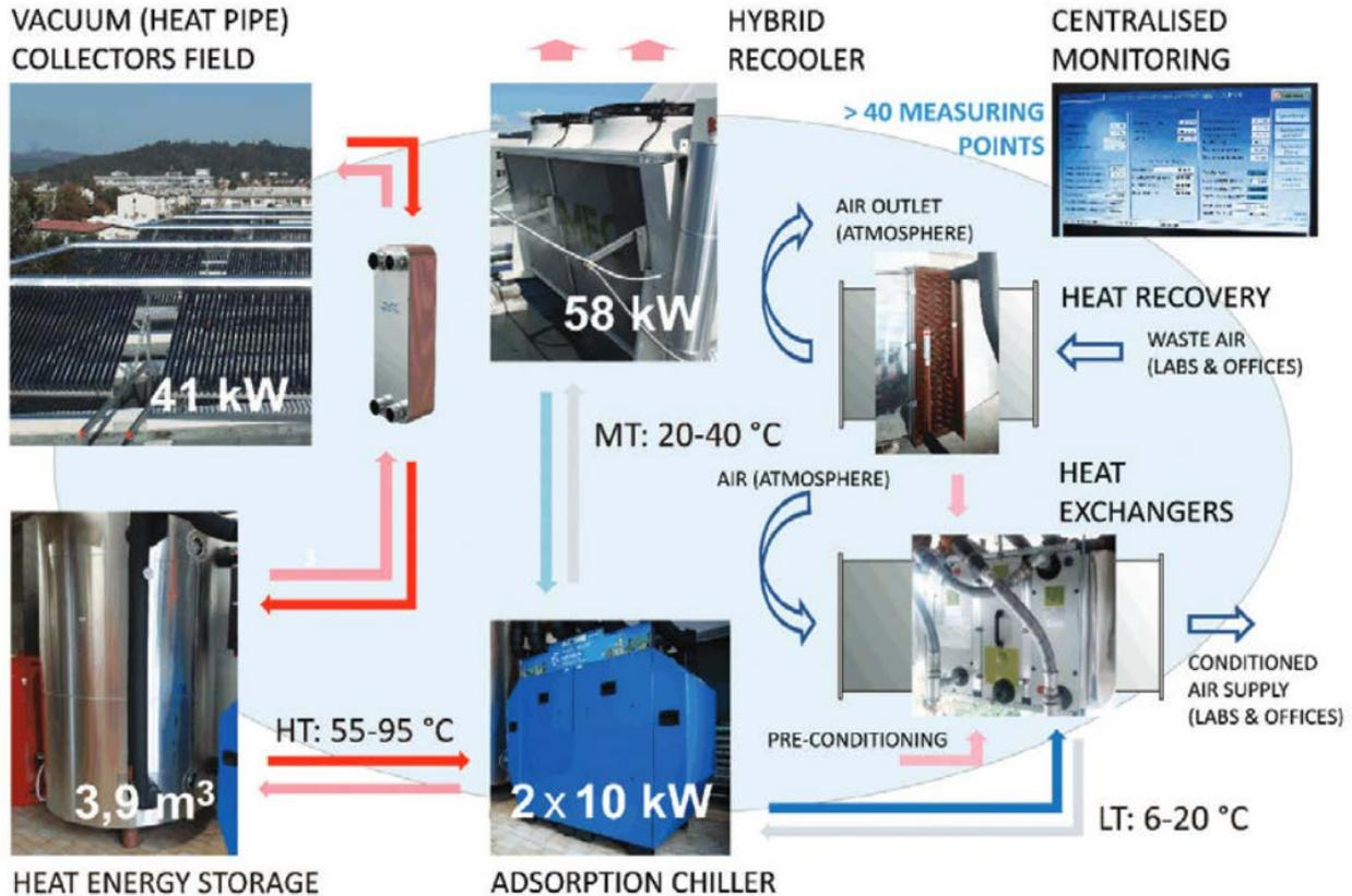
Figure 15: Scheme of the solar cooling system at the Jožef Stefan Institute (Source: JSI)
