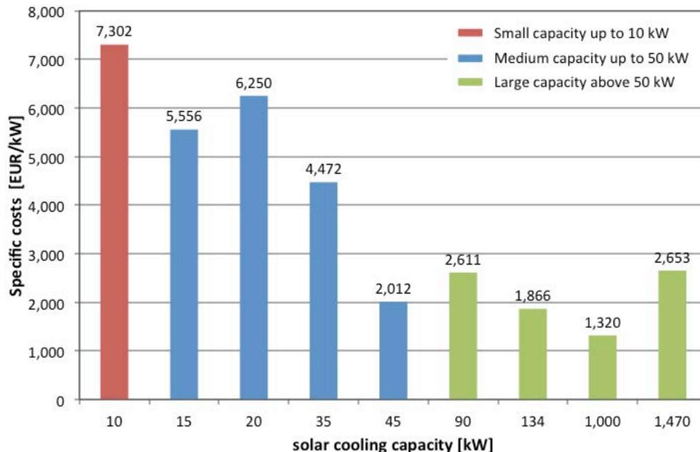
Figure 31: Specific costs of installed best practice solar cooling systems (Source: Green Chiller)
