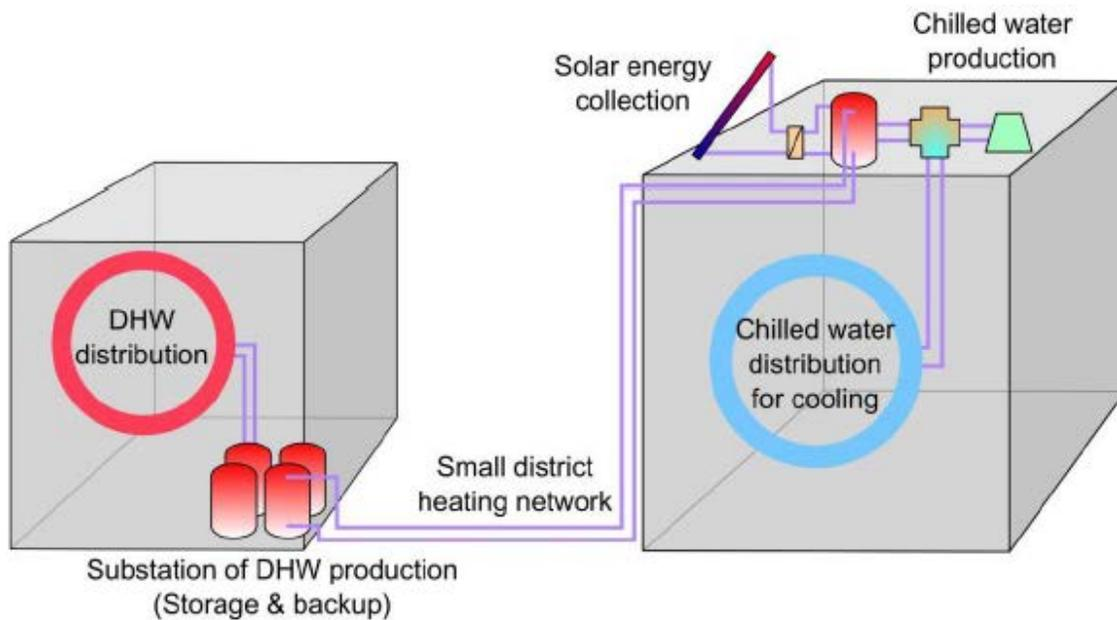
Figure 6: Hydraulic principle of the solar system in reference to the two building (Source: TECSOL)
